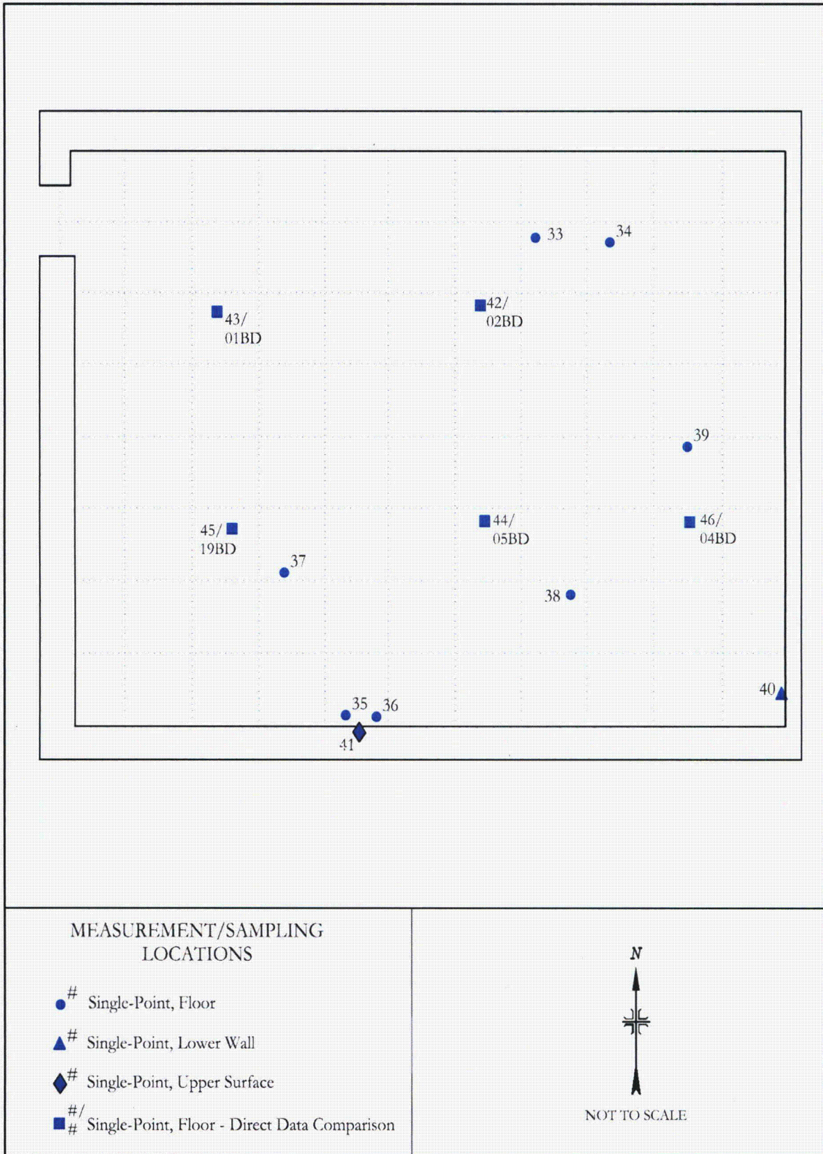
FIGURE 5: Auxiliary Building, Room 25 - Direct Measurement Locations
