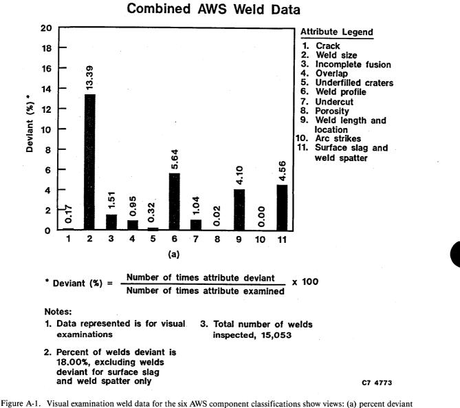
Figure A-1. Visual examination weld data for the six AWS component classifications show views: (a) percent deviant for each attribute inspected and (b) percent of acceptable and deviant attributes and tabulation of the percent of each deviant attribute relative to the total deviant attributes.
