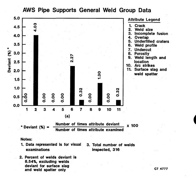
Figure A-5. Visual examination weld data for AWS pipe supports general weld group components show views: (a) percent deviant for each attribute inspected and (b) percent of acceptable and deviant attributes and tabulation of the percent of each deviant attribute relative to the total deviant attributes.
