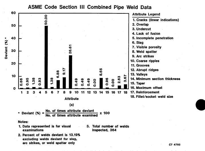
Figure A-20. Visual examination weld data for all ASME Code Section III pipe welds show views: (a) percent deviant for each attribute inspected and (b) percent of acceptable and deviant attributes and tabulation of the percent of each deviant attribute relative to the total number of deviant attributes.
