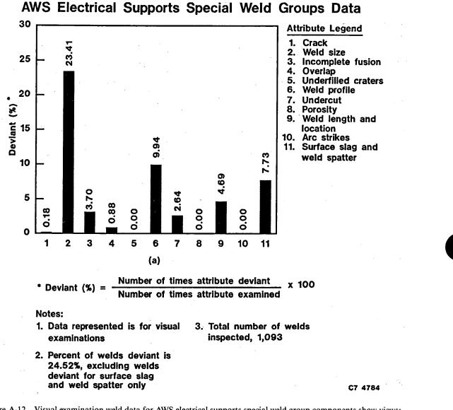
Figure A-12. Visual examination weld data for AWS electrical supports special weld group components show views: (a) percent deviant for each attribute inspected and (b) percent of acceptable and deviant attributes and tabulation of the percent of each deviant attribute relative to the total deviant attributes.
