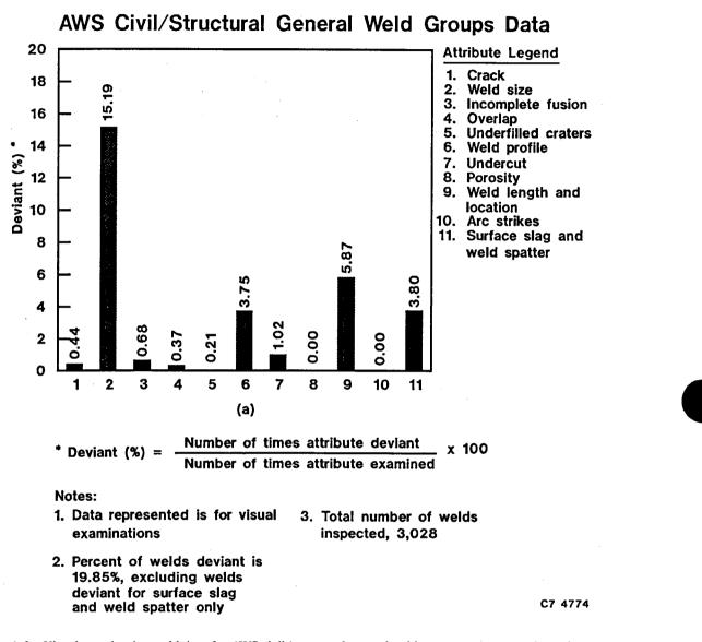
Figure A-2. Visual examination weld data for AWS civil/structural general weld group components show views: (a) percent deviant for each attribute inspected and (b) percent of acceptable and deviant attributes and tabulation of the percent of each deviant attribute relative to the total deviant attributes.
