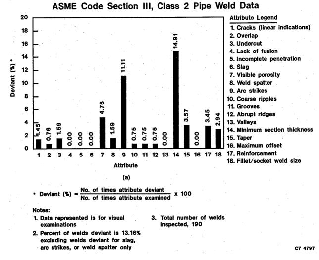
Figure A-26. Visual examination weld data for ASME Code Section III, Class 2 piping welds show views: (a) percent deviant for each attribute inspected and (b) percent of acceptable and deviant attributes and tabulation of the percent of each deviant attribute relative to the total deviant attributes.
