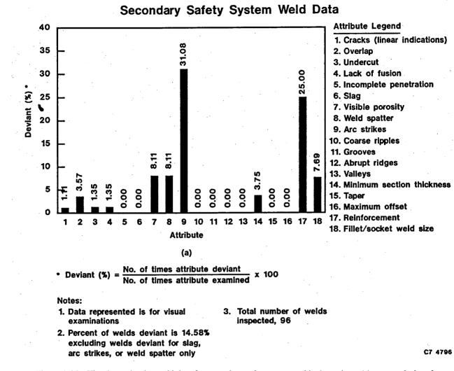
Figure A-25. Visual examination weld data for secondary safety system welds show views: (a) percent deviant for each attribute inspected and (b) percent of acceptable and deviant attributes and tabulation of the percent of each deviant attribute relative to the total deviant attributes.
