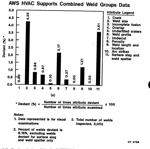
Figure A-16. Visual examination weld data for all AWS HVAC supports weld group components show views: (a) percent deviant for each attribute inspected and (b) percent of acceptable and deviant attributes and tabulation of the percent of each deviant attribute relative to the total deviant attributes.
