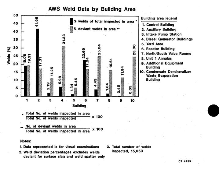
Figure A-23. Visual examination weld data by plant geographic areas (1 through 10) for AWS component classifications showing percent by area of the total welds inspected.
