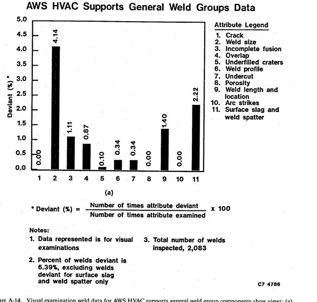
Figure A-14. Visual examination weld data for AWS HVAC supports general weld group components show views: (a) percent deviant for each attribute inspected and (b) percent of acceptable and deviant attributes and tabulation of the percent of each deviant attribute relative to the total number of deviant attributes identified.
