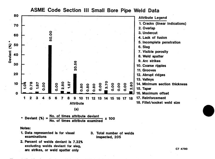
Figure A-18. Visual examination weld data for ASME Code Section III small bore pipe welds show views: (a) percent deviant for each attribute inspected and (b) percent of acceptable and deviant attributes and tabulation of the percent of each deviant attribute relative to the total deviant attributes.
