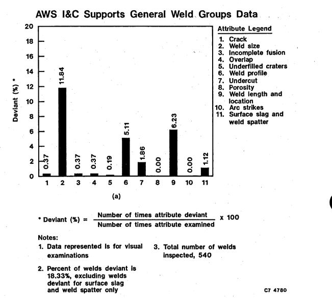
Figure A-8. Visual examination weld data for AWS I&C supports general weld group components show views: (a) percent deviant for each attribute inspected and (b) percent of acceptable and deviant attributes and tabulation of the percent of each deviant attribute relative to the total deviant attributes.
