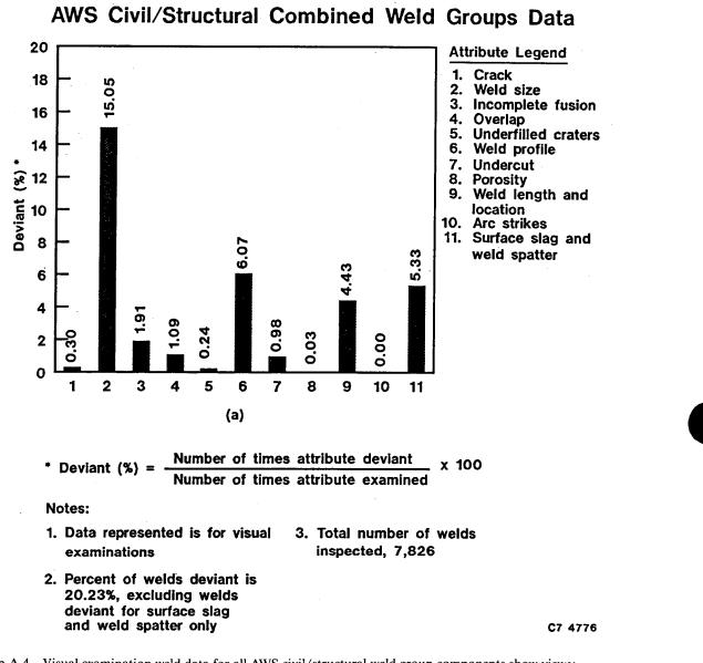
Figure A-4. Visual examination weld data for all AWS civil/structural weld group components show views: (a) percent deviant for each attribute inspected and (b) percent of acceptable and deviant attributes and tabulation of the percent of each deviant attribute relative to the total deviant attributes.
