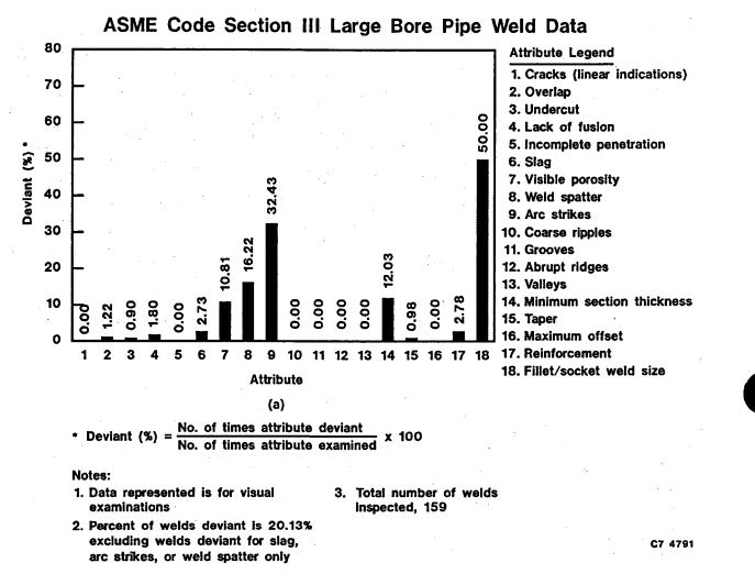
Figure A-19. Visual examination weld data for ASME Code Section III large bore pipe welds show views: (a) percent deviant for each attribute inspected and (b) percent of acceptable and deviant attributes and tabulation of the percent of each deviant attribute relative to the total deviant attributes.
