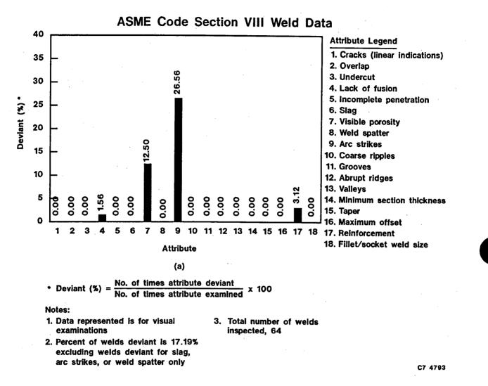
Figure A-21. Visual examination weld data for ASME Code Section VIII welds show views: (a) percent deviant for each attribute inspected and (b) percent of acceptable and deviant attributes and tabulation of the percent of each deviant attribute relative to the total deviant attributes.
