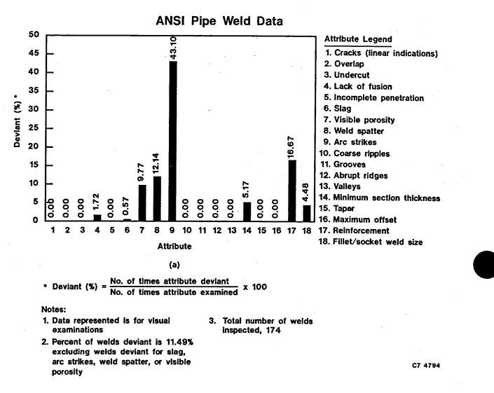
Figure A-22. Visual examination weld data for ANSI piping welds show views: (a) percent deviant for each attribute inspected and (b) percent of acceptable and deviant attributes and tabulation of the percent of each deviant attribute relative to the total deviant attributes.
