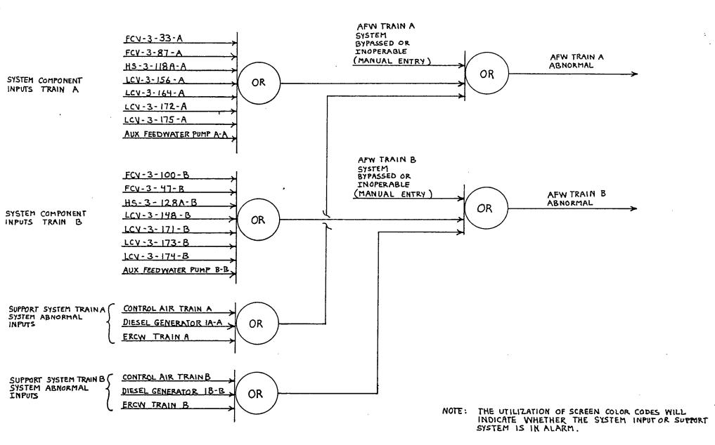
FIGURE 1 SAMPLE LOGIC TREE FOR AUXILIARY FEED WATER SYSTEM A strand grant strate
