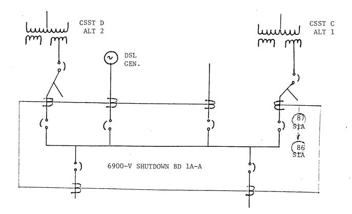
The design of the protective scheme is such that it would require multiple failure to incapacitate both offsite power sources.
