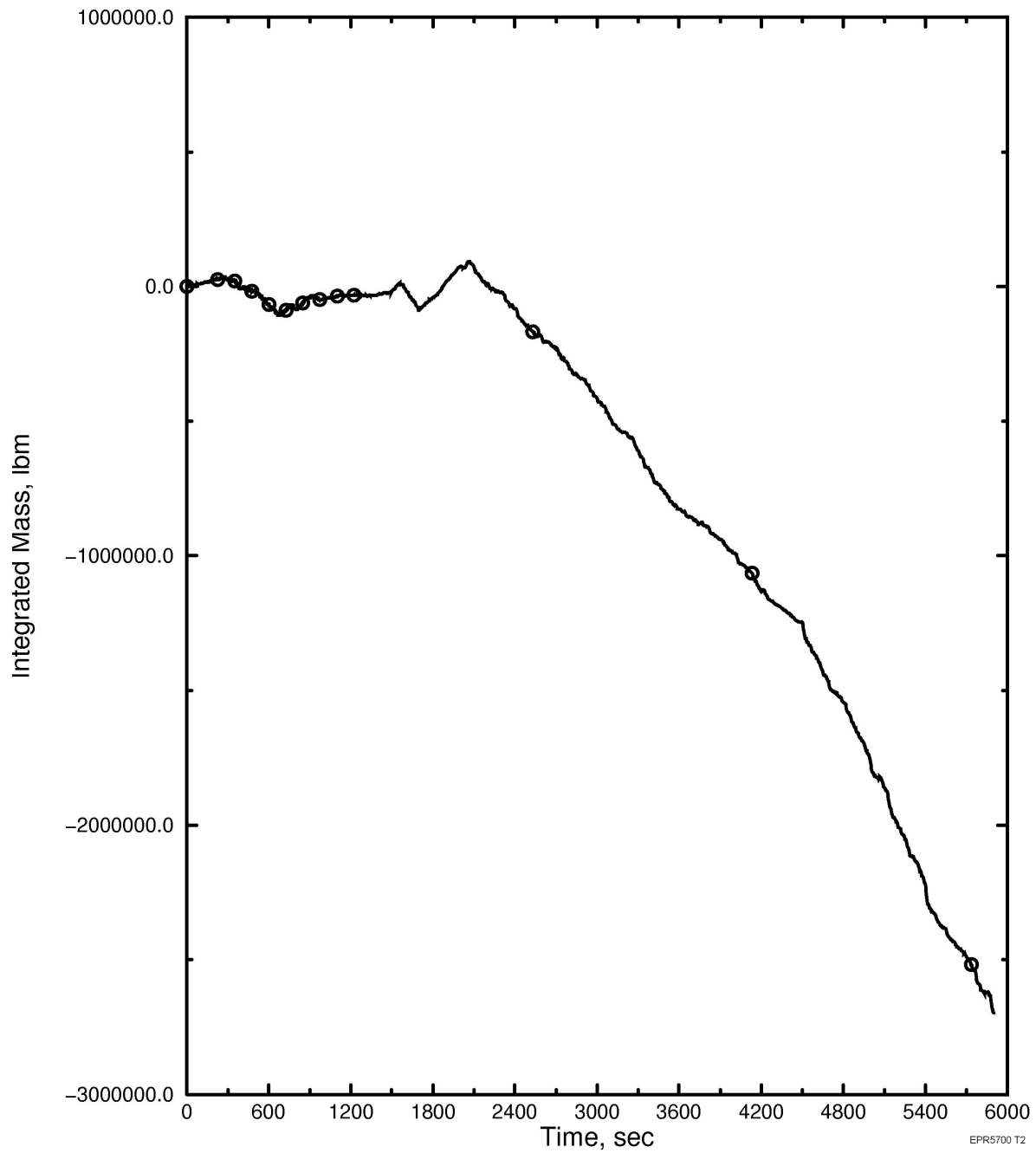
Figure 15.6-89—Peripheral Core Region Flow into Upper Plenum
