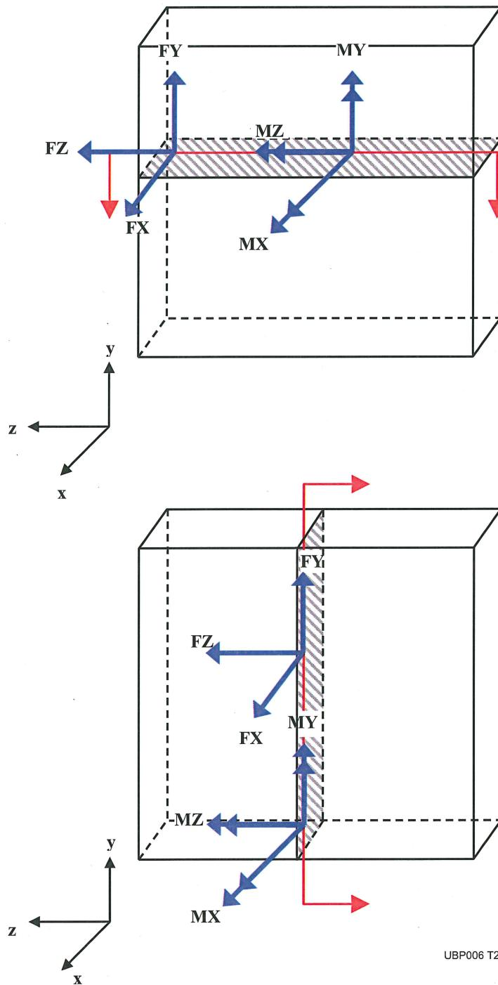
**Figure 3E.2-6—Nomenclature for Section Cuts through EPGB Wall at Column Line 11**
