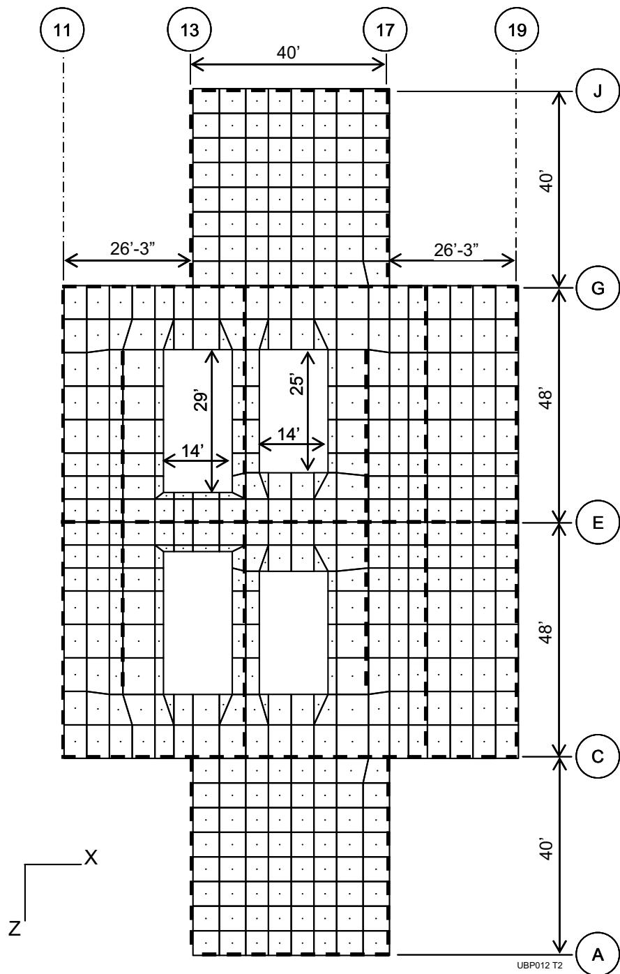
Figure 3E.2-12—Design Sketch of EPGB Elevation 51'-6"
