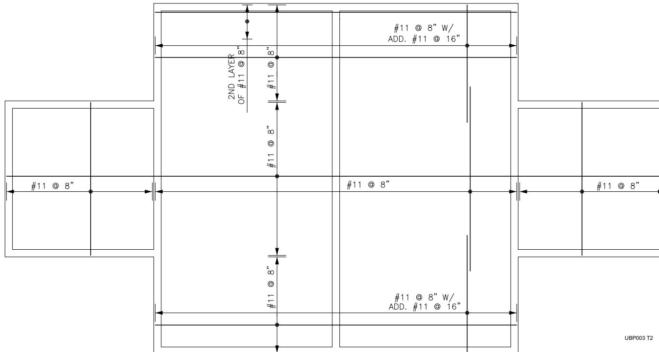
**Figure 3E.2-4—EPGB Wall at Column Line 11 - GT STRUDL FEM**
