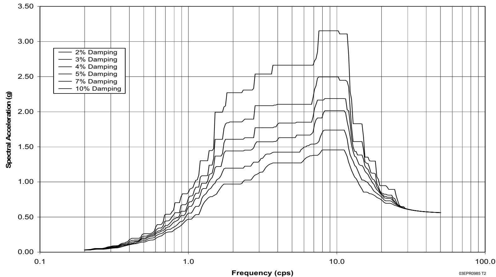
Figure 3.7.2-104—Spectrum Envelope of ESWB at Elev +63 ft, 0 inches at Node 12733 2%, 3%, 4%, 5%, 7% and 10% Damping X-Direction
