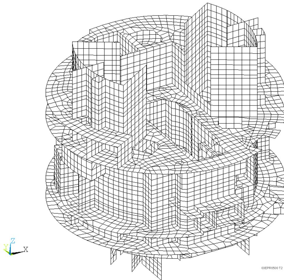
**Figure 3.7.2-10—Stick Model STICK-2T for Balance of NI Common Basemat Structures - Plan View**
