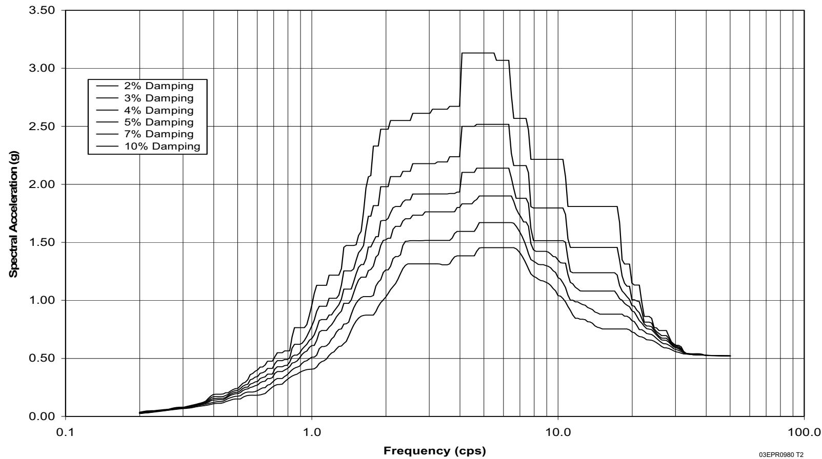
Figure 3.7.2-103—Spectrum Envelope of EPGB at Elev. +0 ft, 0 inches at Node 1172 2%, 3%, 4%, 5%, 7% and 10% Damping Z-Direction
