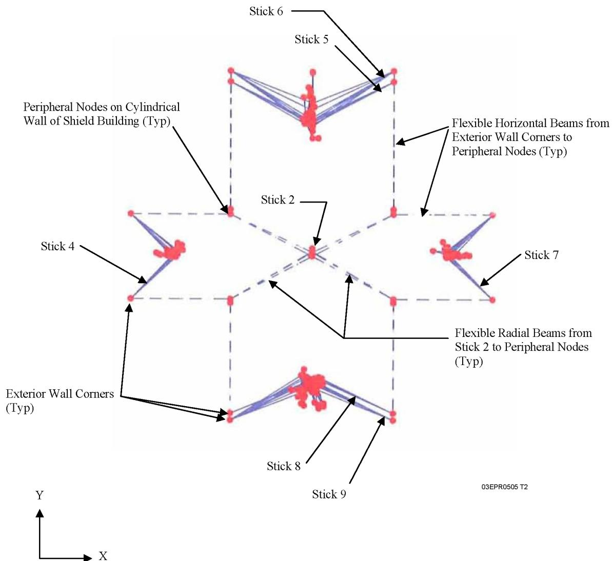
Figure 3.7.2-11—Stick Model STICK-2T for Balance of NI Common Basemat Structures - Perspective View
