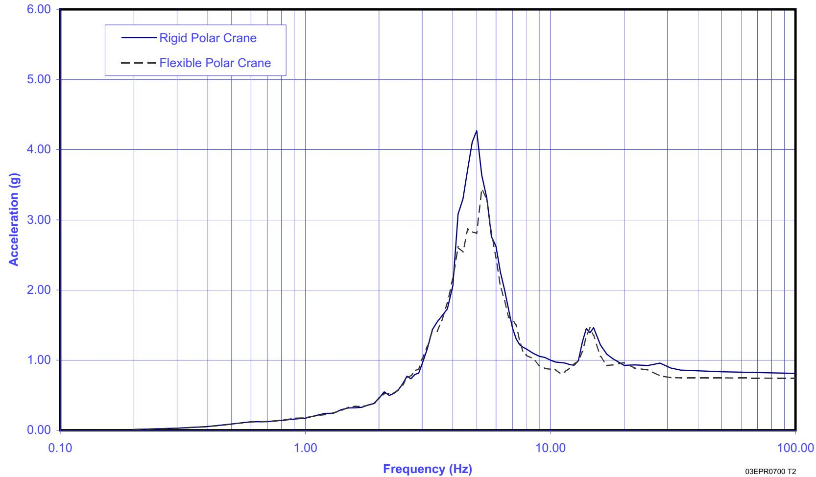
Figure 3.7.2-49—Spectrum Comparison at Elev. +123 ft, 4-1/4 inches (+37.60m) - Containment Building (Rigid vs. Flexible Polar Crane), 5% Damping, Z-Direction
