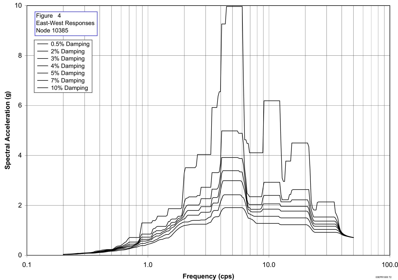
Figure 3.7.2-108—Spectrum Envelope of ESWB at Elev +14 ft, 0 inches at Node 10385 2%, 3%, 4%, 5%, 7% and 10% Damping Y-Direction
