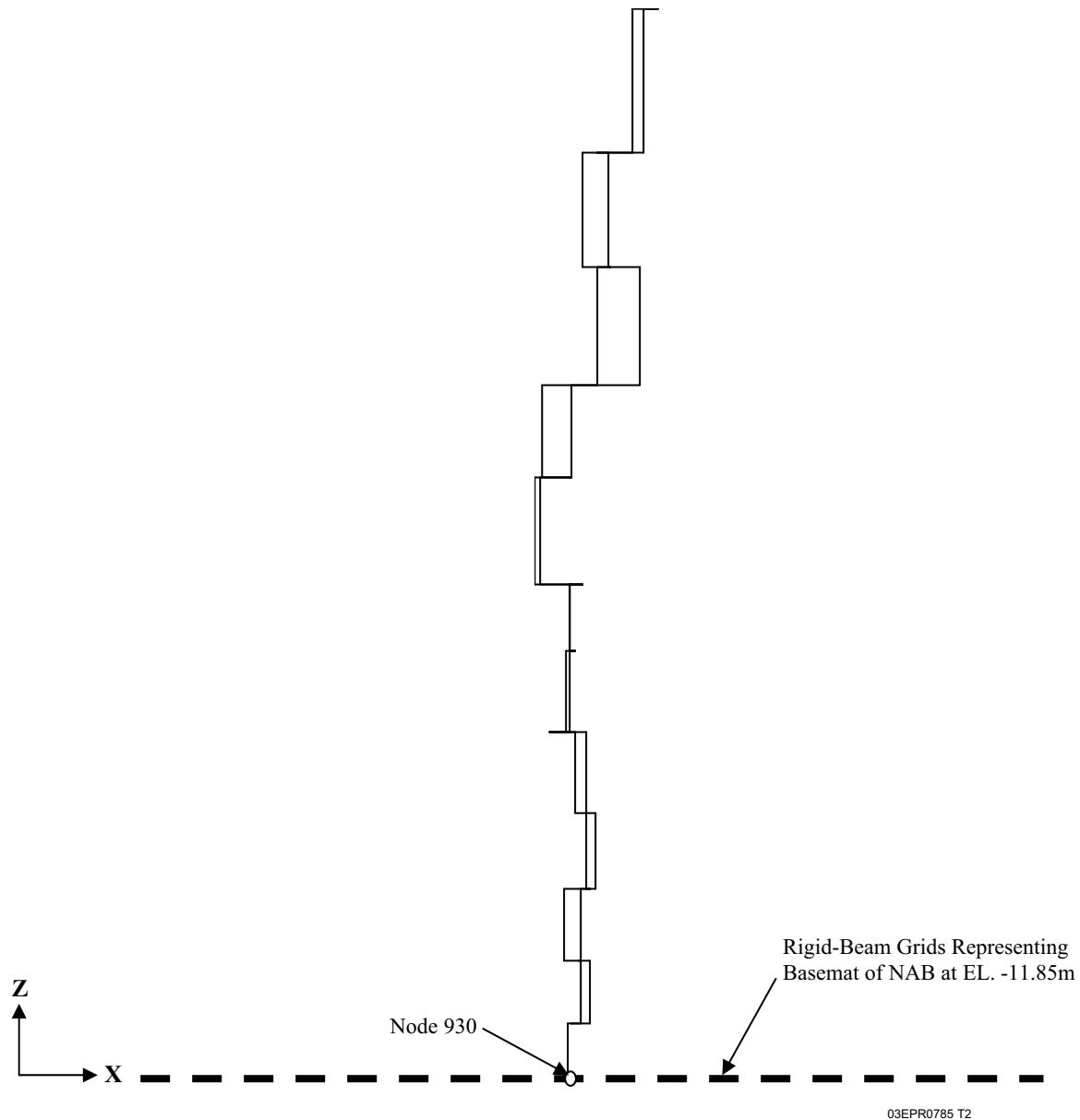
**Figure 3.7.2-67—Elevation View of NAB Stick Model in Y-Z Plane**
