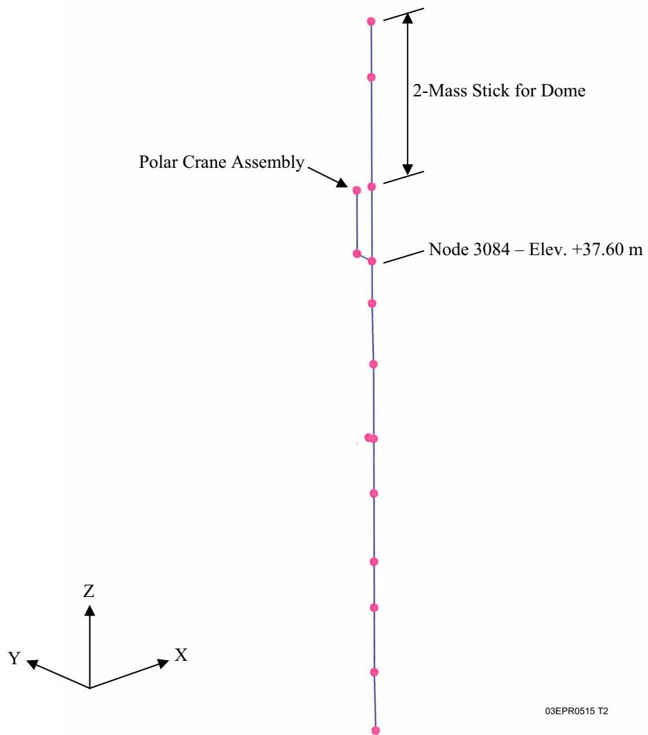
**Figure 3.7.2-13—Stick Model STICK-1T for Reactor Building Internal Structure - Perspective View**
