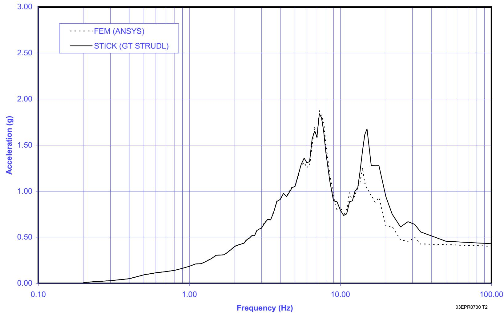
Figure 3.7.2-55—Spectrum Comparison at Elev. +16 ft, 10-3/4 inches (+5.15m) - Reactor Building Internal Structure, 4% Damping, Z-Direction
