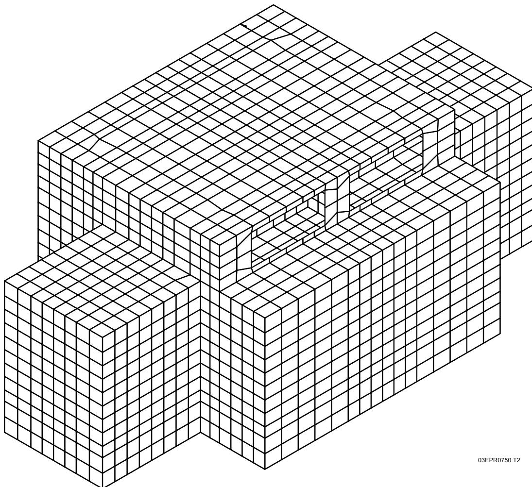
**Figure 3.7.2-58—Section View of GTSTRUDL FEM for Emergency Power Generating Building**
