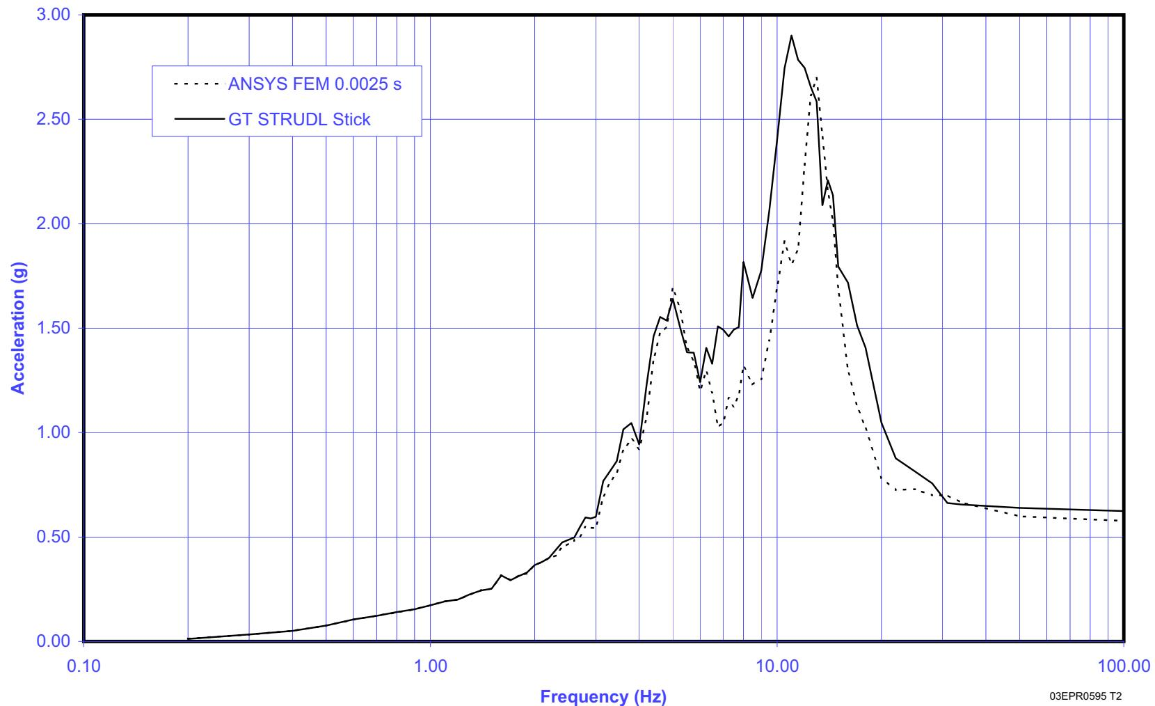
**Figure 3.7.2-29—Stick vs. FEM Spectrum Comparison at Elev. +68 ft, 10-3/4 inches (+21.00m) - Safeguard Building 2/3, 5% Damping, X-Direction**
