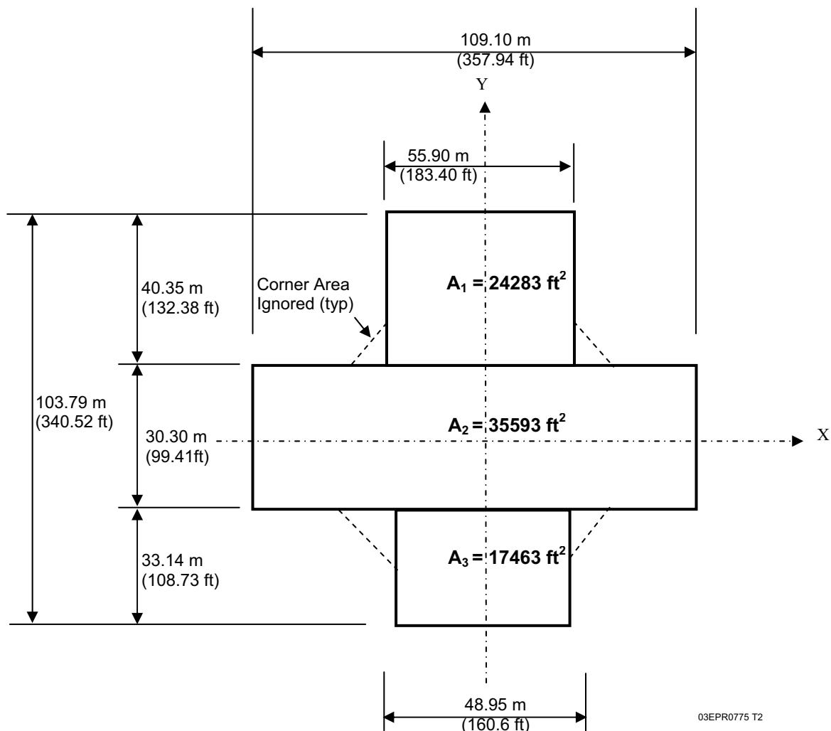
**Figure 3.7.2-65—RCS Stick Coupled to Model STICK-1T for Reactor Building Internal Structure**
