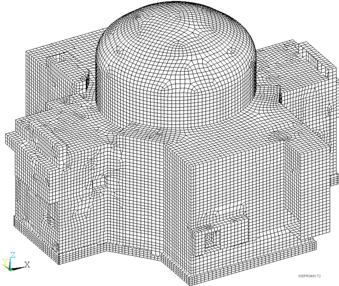
**Figure 3.7.2-6—3D Finite Element Model of Balance of NI Common Basemat Structures Cutoff View on Y-Z Plane**
