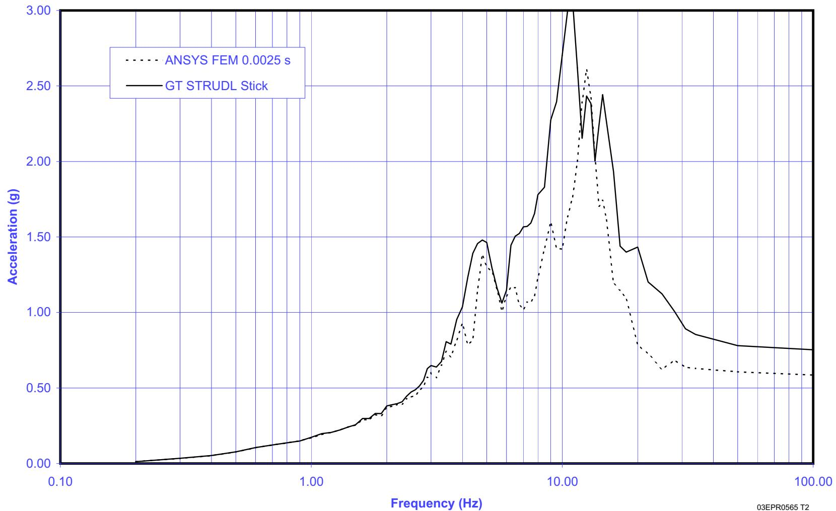
Figure 3.7.2-23—Stick vs. FEM Spectrum Comparison at Elev. +95 ft, 1-3/4 inches (+29.00m) - Safeguard Building 4, 5% Damping, X-Direction
