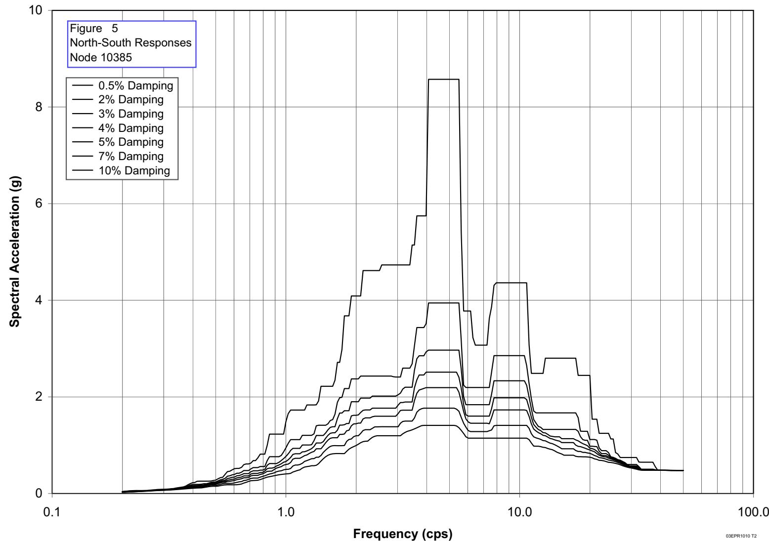
Figure 3.7.2-109—Spectrum Envelope of ESWB at Elev +14 ft, 0 inches at Node 10385 2%, 3%, 4%, 5%, 7% and 10% Damping Z-Direction
