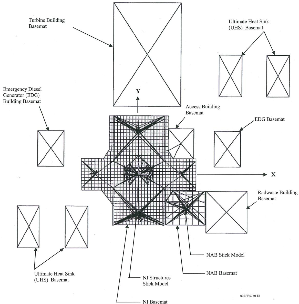
Figure 3.7.2-63—Elevation View of SSI Model for NI Common Basemat Structures and NAB in X-Z Plane
