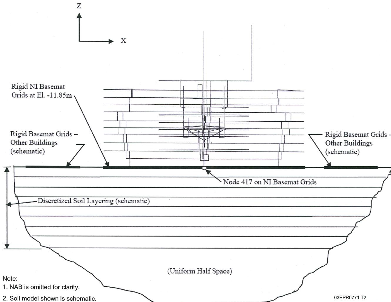
**Figure 3.7.2-64—Schematic Footprint Area of NI Common Basemat**
