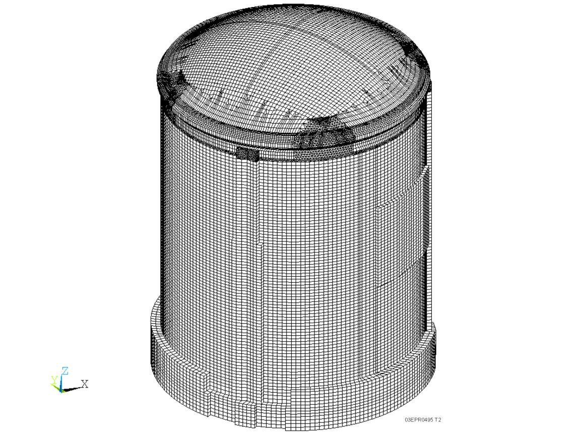
**Figure 3.7.2-9—3D Finite Element Model of Reactor Building Internal Structures**
