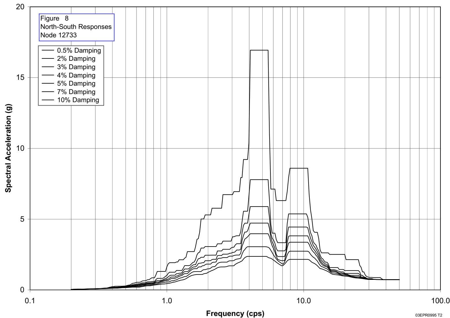
Figure 3.7.2-106—Spectrum Envelope of ESWB at Elev +63 ft, 0 inches at Node 12733 2%, 3%, 4%, 5%, 7% and 10% Damping Z-Direction
