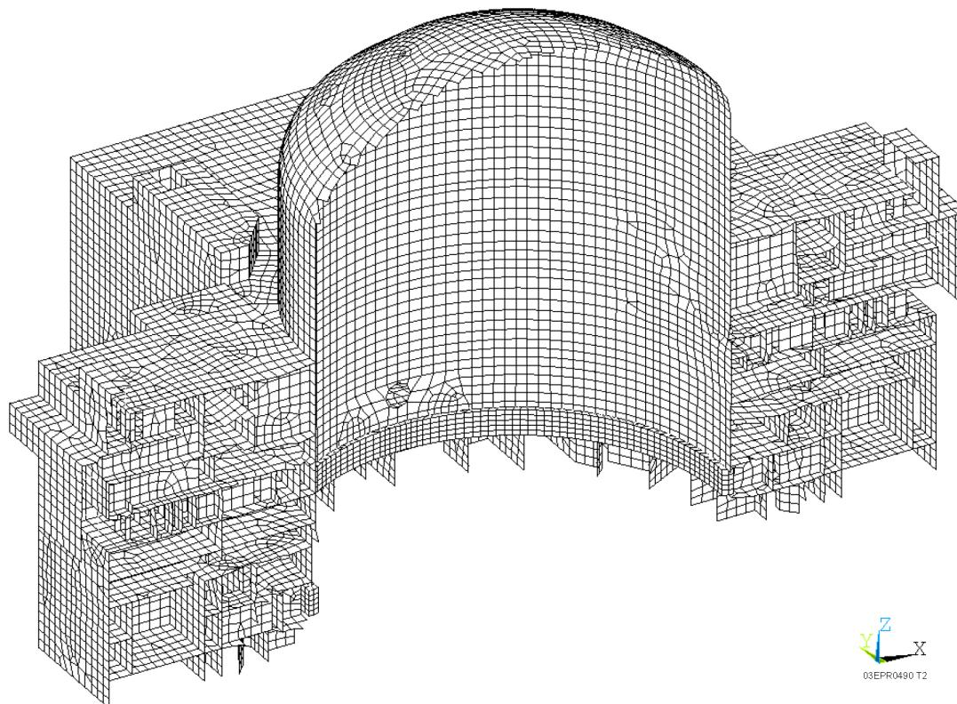
**Figure 3.7.2-8—3D Finite Element Model of Reactor Containment Building**
