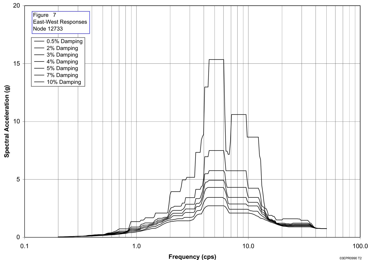
Figure 3.7.2-105—Spectrum Envelope of ESWB at Elev +63 ft, 0 inches at Node 12733 2%, 3%, 4%, 5%, 7% and 10% Damping Y-Direction
