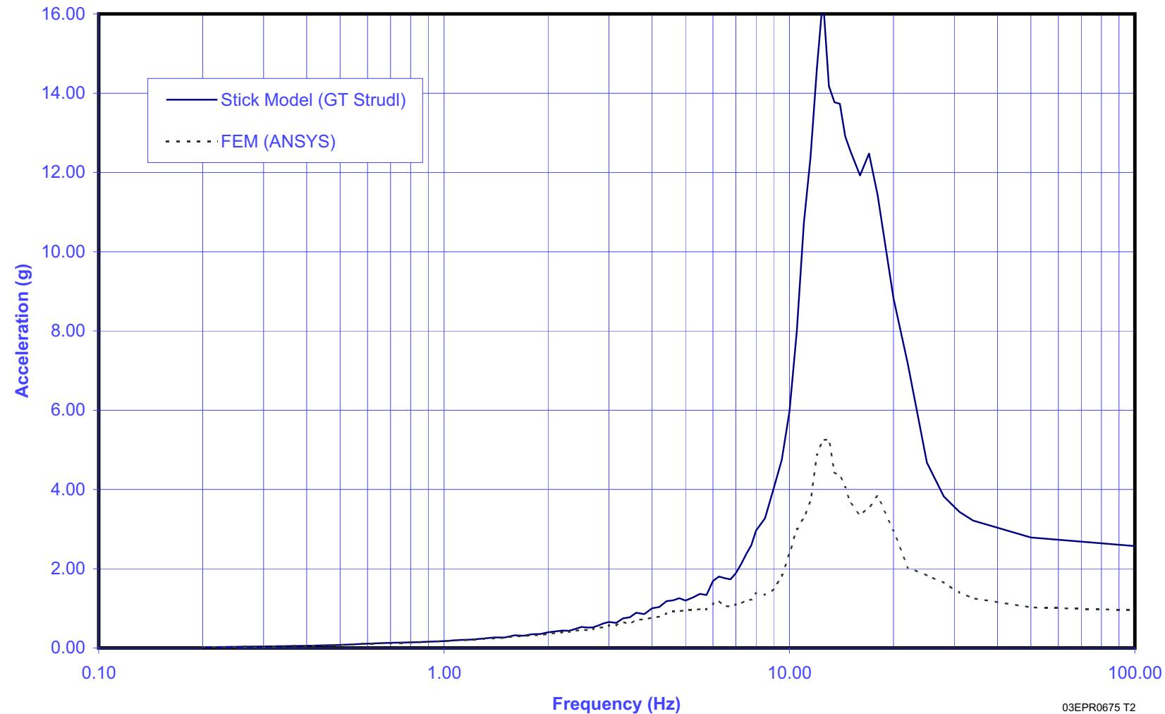
Figure 3.7.2-44—Stick vs. FEM Spectrum Comparison at Elev. +123 ft, 4-1/4 inches (+37.60m) - Containment Building (Without Polar Crane), 5% Damping, X-Direction
