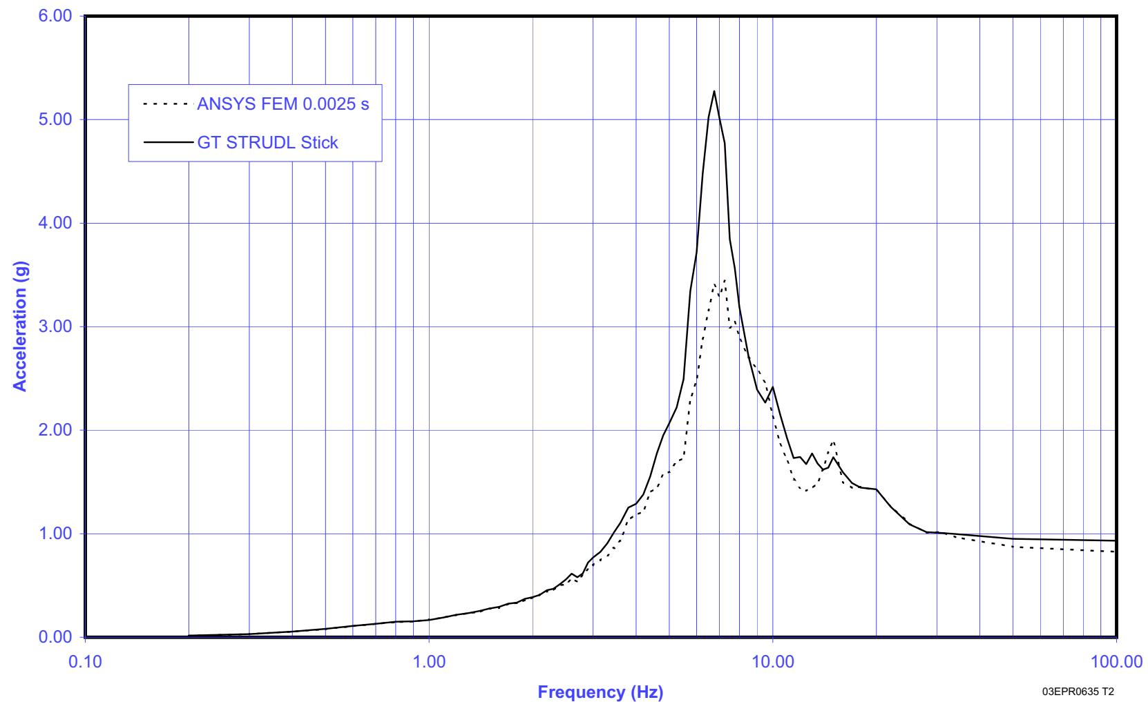
Figure 3.7.2-36—Stick vs. FEM Spectrum Comparison at Elev. +62 ft, 4-1/4 inches (+19.00m) - Fuel Building, 5% Damping, Y-Direction
