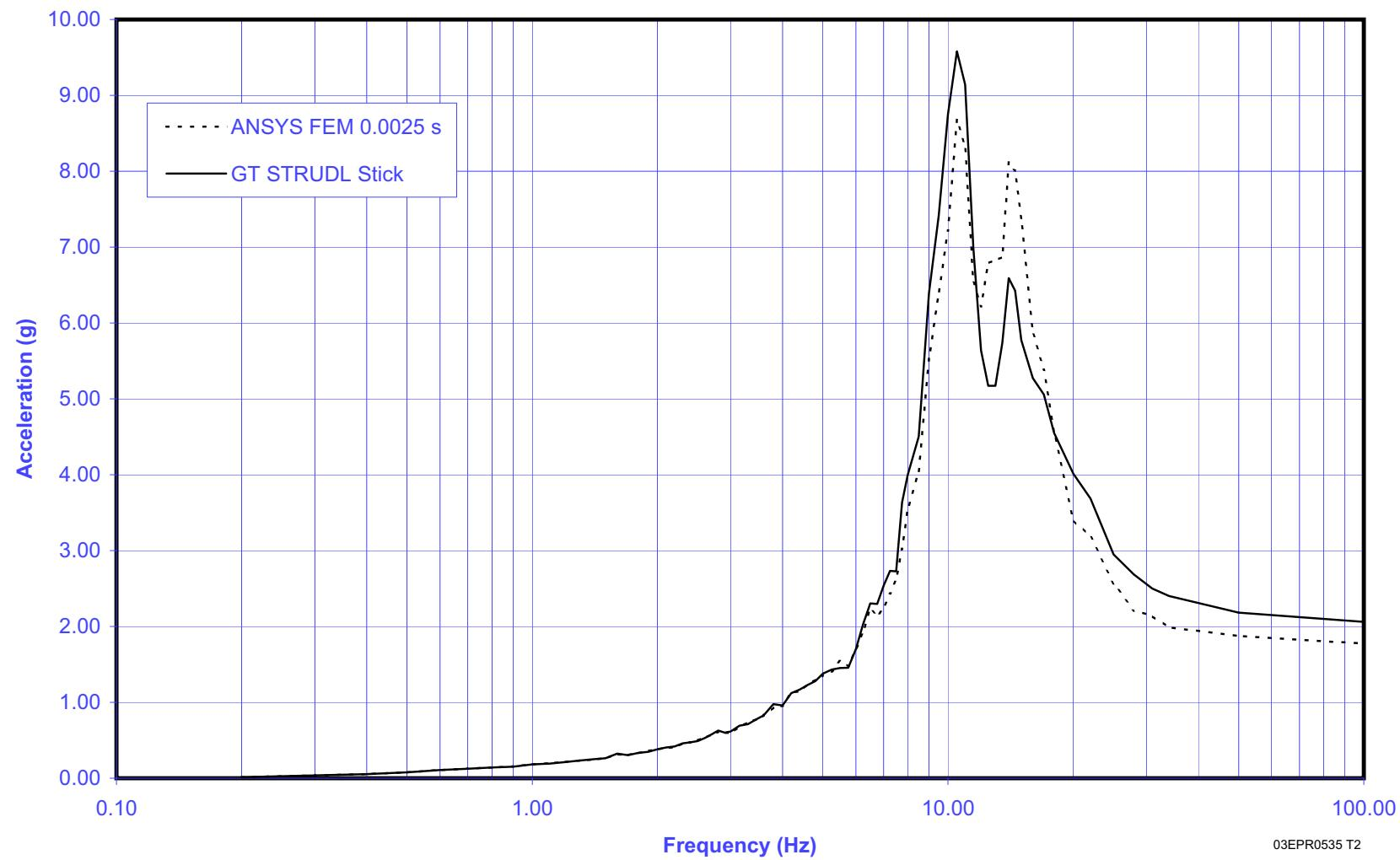
Figure 3.7.2-17—Stick vs. FEM Spectrum Comparison at Elev. +95 ft, 1-3/4 inches (+29.00m) - Safeguard Building 1, 5% Damping, X-Direction
