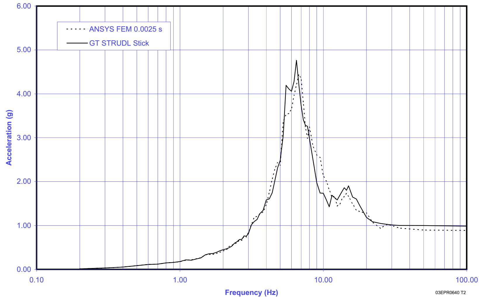
Figure 3.7.2-37—Stick vs. FEM Spectrum Comparison at Elev. +62 ft, 4-1/4 inches (+19.00m) - Fuel Building, 5% Damping, Z-Direction
