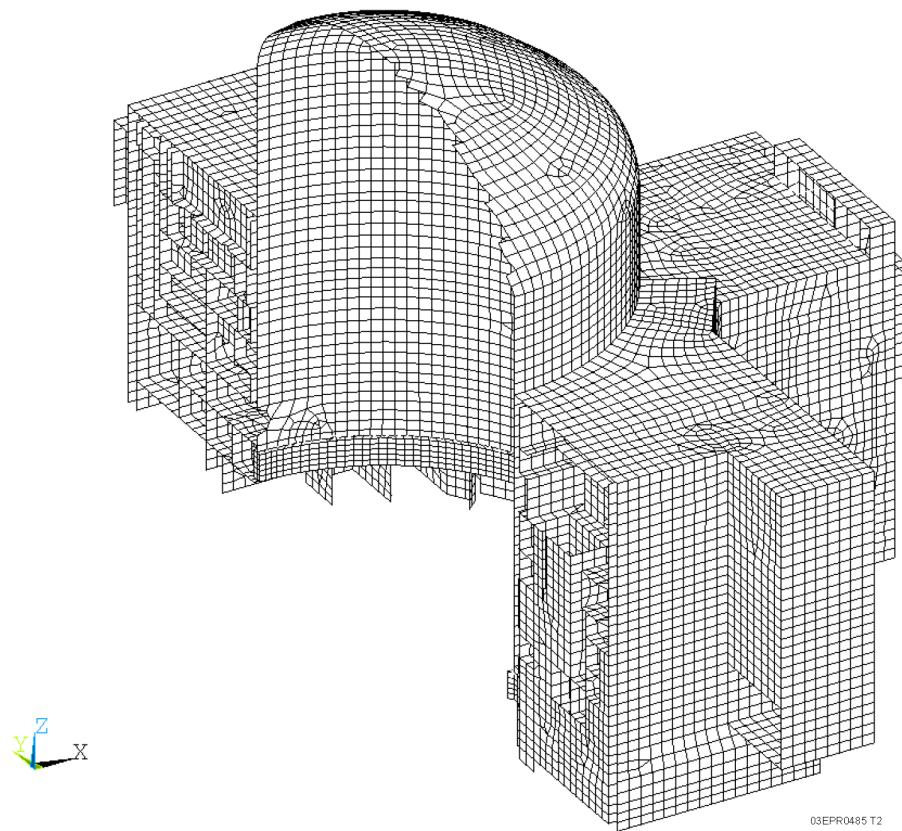
**Figure 3.7.2-7—3D Finite Element Model of Balance of NI Common Basemat Structures Cutoff View on X-Z Plane**
