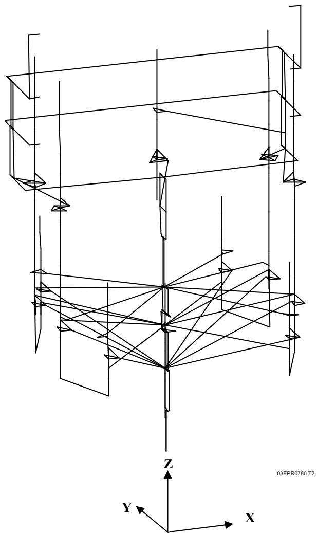
**Figure 3.7.2-66—Elevation View of NAB Stick Model in X-Z Plane**
