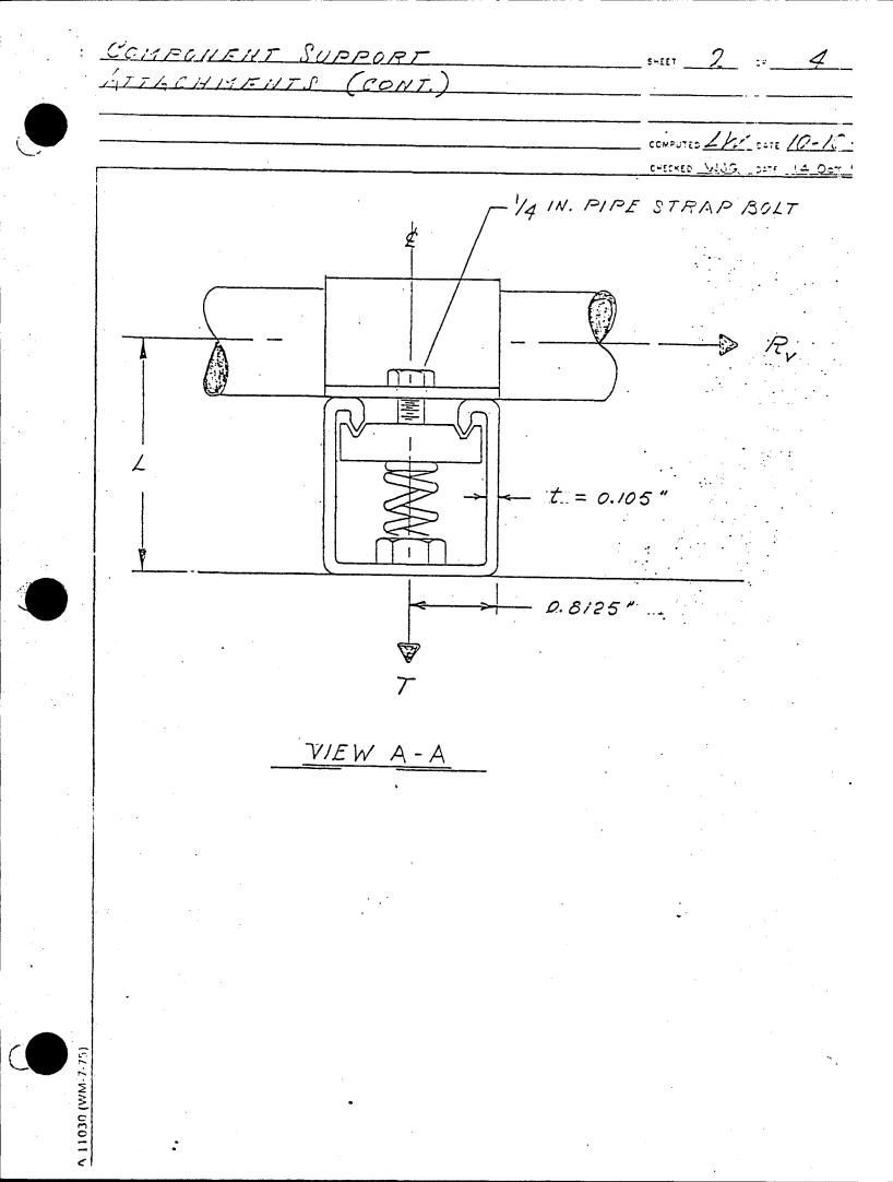
MEUNENT OUNP \_ SHEET \_\_\_\_\_ OF 4 CONT SHITENTS (CONT) COMPUTED -11 DATE 10-10-CHECKED WUG CATE 14 OCT B BEAM ANALOGY PIOOD UNISTRUT SIDES 2t = 0.21" R MAXIMUM BENDING MOMENT : ASSUME L & GIN. (SEE VIEW A-A)  $M_{\rm A} = M_{\rm B} = R_{\rm Y} \frac{1}{2} = 3 R_{\rm Y}$ MOMENT-OF-INERTIA OF CHANNEL SIDES :  $I = \frac{b(2t)^3}{12} = 0.0031 \text{ in }^4$ WHERE: B = MINIMUM SPACING BETWEEN ANCHORS (4 IN.) t = CHANNEL MATERIAL THICKNESS (0.105 M.)
