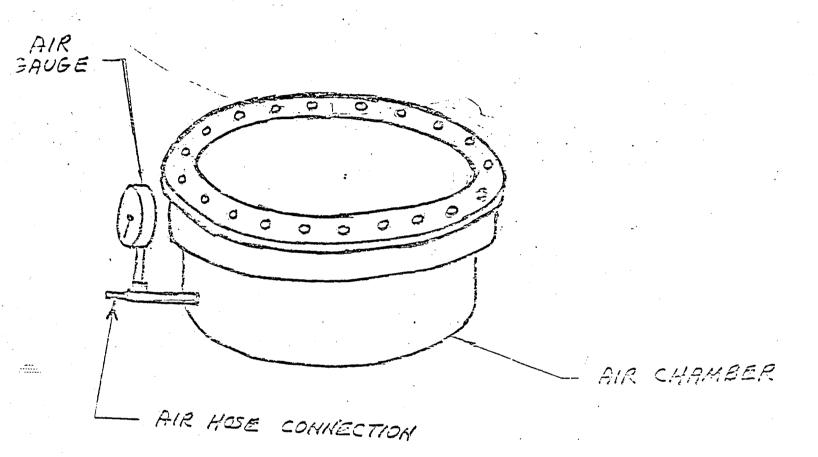
Figure 1. "Sketch of Pressure Test Fixture for Ice Condenser Seals"
