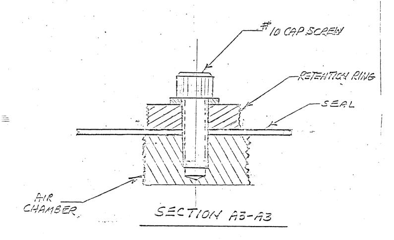
Figure 3 "Sketch of Hold-down Assembly - Section A3-A3
