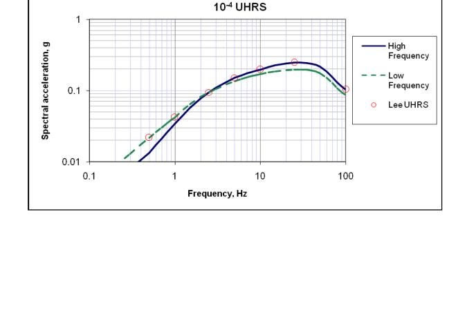
WILLIAM STATES LEE III NUCLEAR STATION UNITS 1 & 2 High-Frequency and Low-Frequency Rock Spectra for 10<sup>-4</sup> Annual Frequency of Exceedence FIGURE 2.5.2-237 Rev 0
