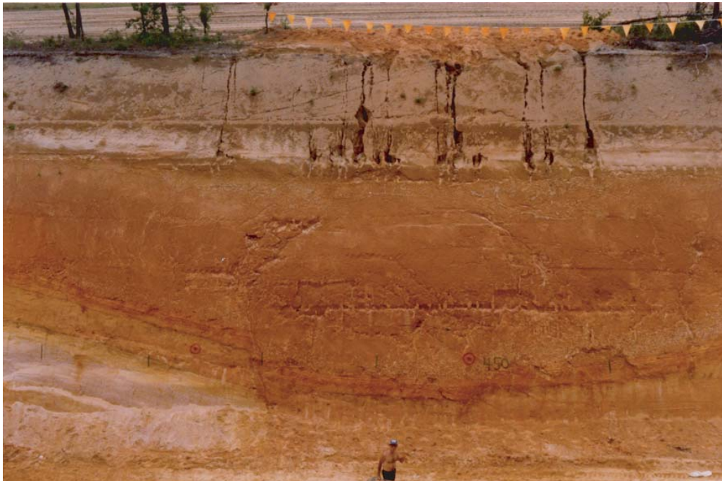
Figure 2.5.3-2 West Wall of Garbage Trench Showing Small Offsets (1–24 inches) (Upper) and Arcuate Fractures and Clastic Dikes Over Center of Depression (Lower)
