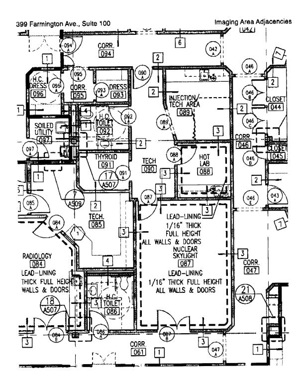
NOTE: The Hot Lab is equipped with a base cabinet, a counter-top + sink, an L-block shield, dose calibrator, GM survey meter, shielded prep area, and above/below cabinet storage for records, wastes and supplies.
