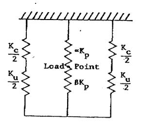
Figure 4.2 Mathematical Model of the U-Bolt / Pipe Assembly
