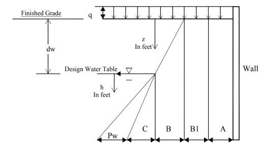
A = 1.47 (q) = Effect of uniform full coverage surface surcharge B1 = 3346 psf = Passive earth pressure at ground surface due to soil cohesion B = 194 (z) = Passive earth pressure above water table C = 102.3 (h) = Passive earth pressure increment below water table Pp = A + B1 + B = Passive lateral earth pressure above water table (z  $\leq$  dw) Pp = A + B1 + 194.3 dw + 102.3 (z – dw) = Passive lateral earth pressure below water table
