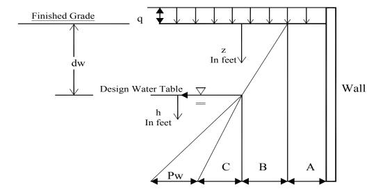
A = 0.81 (q) = Effect of uniform full coverage surface surcharge B = 106.9 (z) = Earth pressure at rest above water table C = 56.4 (h) = Earth pressure at rest increment below water table Pw = 62.4 (h) = Hydrostatic pressure increment H = A + B = Static lateral earth pressure above water table ( $z \le dw$ ) H = A + 106.9 (dw) + 56.4 (z - dw) = Static lateral earth pressure below water table (z > dw) (Pw not included)
