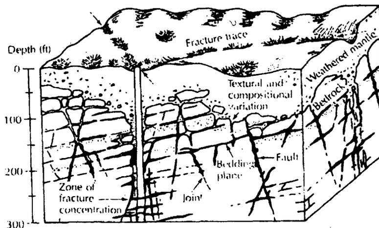
**FIGURE 8.25** Concentration of ground water along zones of fracture concentrations in carbonate rock. Wells that do not intercept an enlarged fracture or a bedding plane may be dry, thus indicating a discontinuous water table. Source: L. H. Lattman and R. R. Parizek, *Journal of Hydrology*, 2 (1964):73-91. Used with permission of Elsevier Scientific Publishing Company, Amsterdam.
