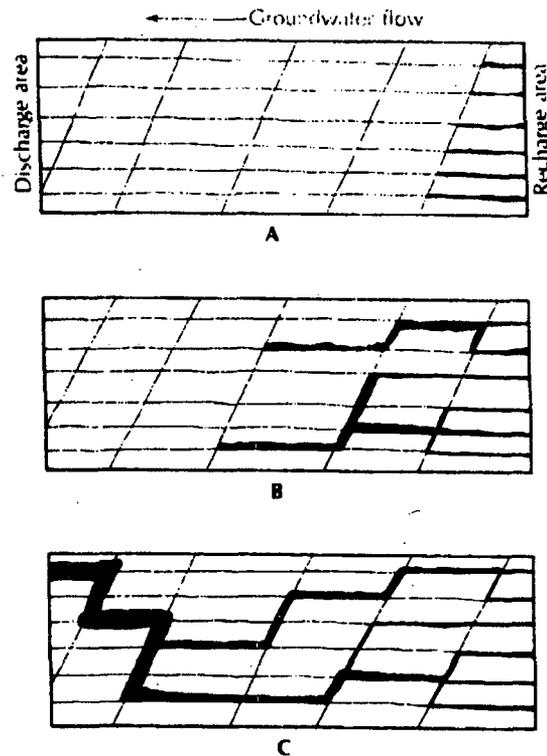
**FIGURE 8.21** Growth of a carbonate aquifer drainage system starting in the recharge area and growing toward the discharge area. **A.** At first, most joints in the recharge area undergo solution enlargement. **B.** As the solution passages grow, they join and become fewer. **C.** Eventually, one outlet appears at the discharge zone.
