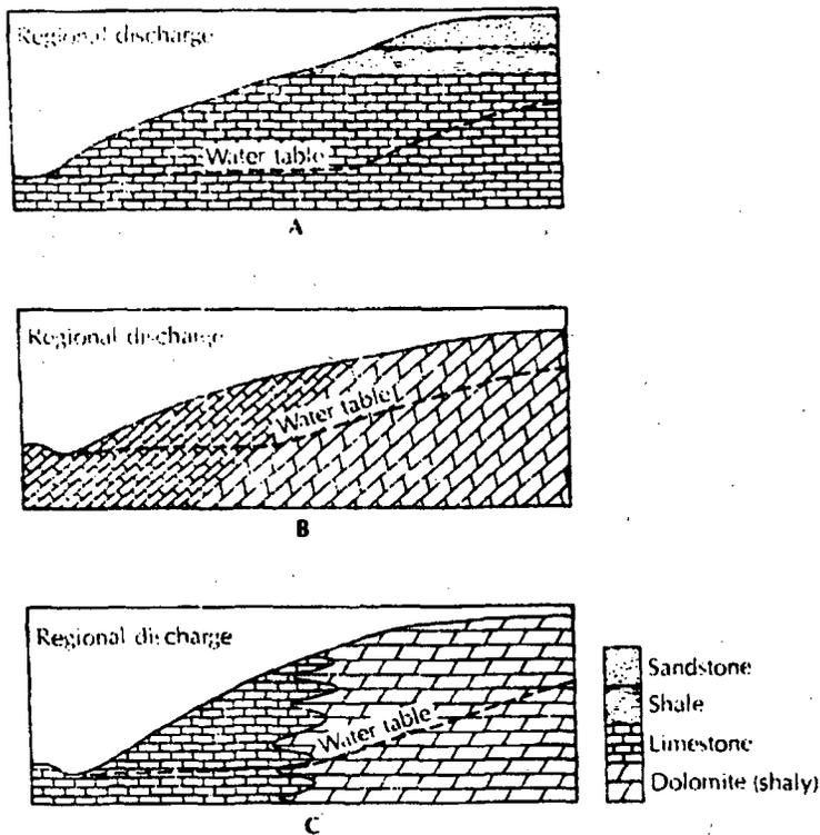
FIGURE 8.24 Geologic conditions resulting in a difference in hydraulic conductivity; hence, a difference in the water-table gradient.
