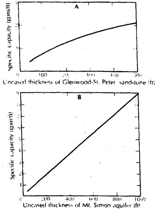
**FIGURE 8.19** Relation between the specific capacity of a well (gallons per minute of yield per foot of drawdown) and the uncased thickness of the sandstone aquifer: **A.** Glenwood-St. Peter Sandstone. **B.** Mt. Simon Sandstone. Both of northern Illinois. Source: W. C. Walton and S. Csallany, Illinois State Water Survey Report of Investigation 43, 1962.
