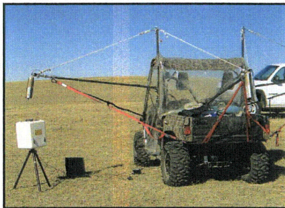
Figure 6.1-3: Measurements for cross-calibration of NaI detectors against the HPIC at a 4.5-foot NaI detector height.
