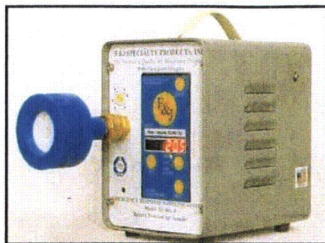
Figure 6.1-29: F&J air particulate sampler.
