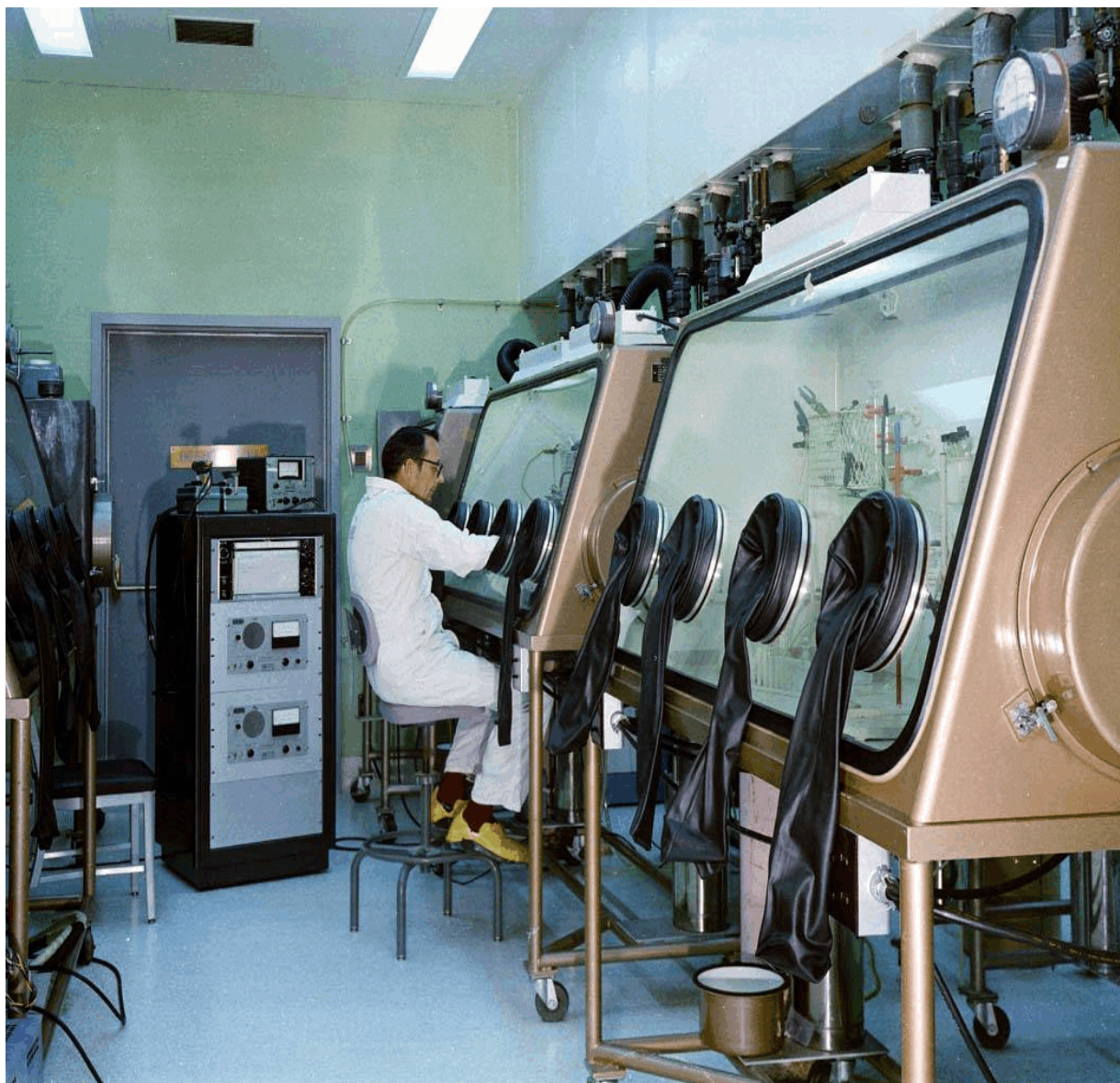
Fig. 12 Glove boxes used for handling nuclear materials having low levels of penetrating radiation
