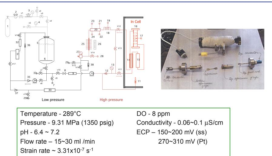
Stabilize test condition by soaking the specimen in high-DO water >24 hr
