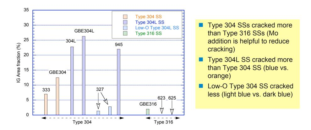
Appear to be significant differences within alloy types; such heat-to-heat variability may be dependent on differences in microstructure & minor impurity levels
