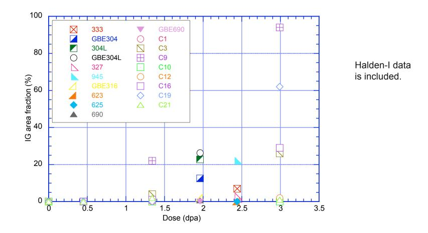
IG cracking does not occur below 0.45 dpa  $(3 \times 10^{20} \text{ n/cm}^2)$  for the commercial heats of austenitic SSs in the Halden irradiations.
