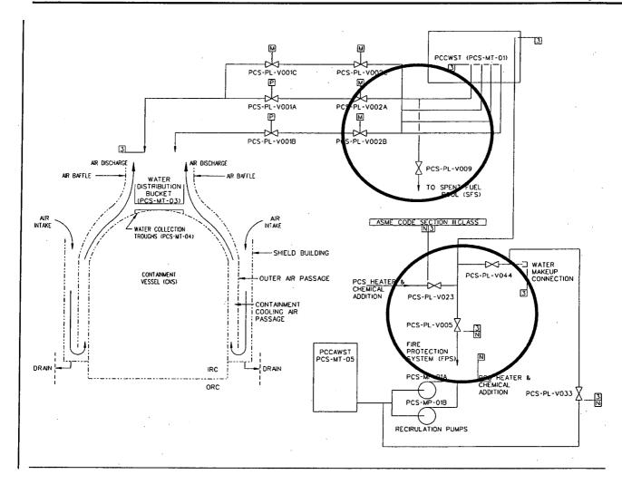
Figure 2.2.2-1 Passive Containment Cooling System
