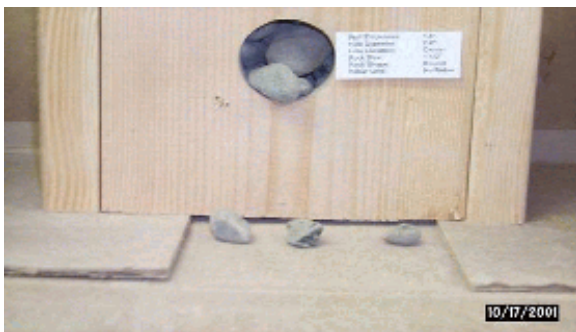
Figure 5-27. Prototype gabion wall construction showing small rock flowing easily through rebar.
