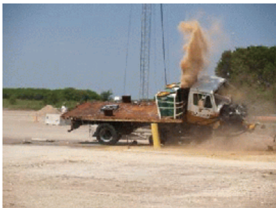
Figure 5-5. Testing new shallow mount vehicle barrier design
