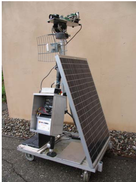
Figure 5-35. Prototype solar powered smart camera with wireless link.
