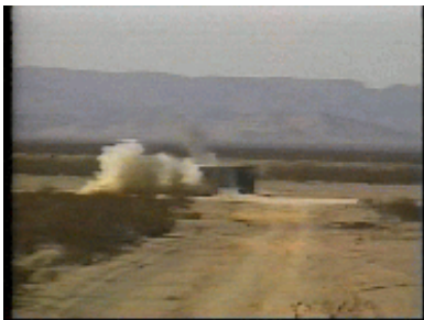
Figure 5-53. Silent Defender ® being subjected to an explosion.
