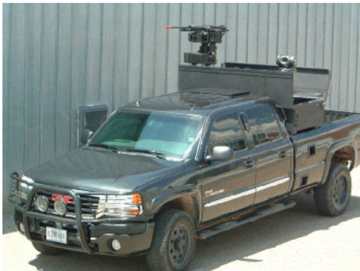
Figure 5-12. Advanced Concept Armored Vehicle II prototype with weapon aiming and surveillance platform.
