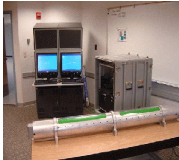
Figure 5-24. Munitions-Based Access Denial System (MBADS) command and control system, fire set, and MBADS assembly.
