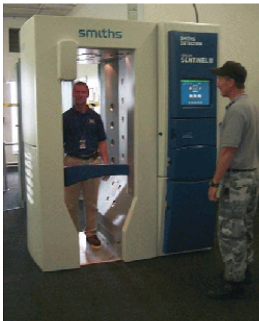
Figure 5-1. Trace explosives detection personnel portal undergoing a test at a Department of Energy facility.
