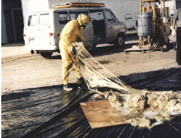
Figure 5-18. Attacker attempting to remove object covered in sticky foam.
