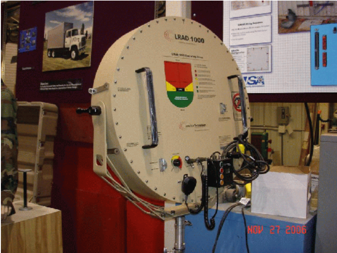
Figure 5-17. Backside image of Sandia National Laboratories' ATC Long Range Acoustical Device™ 1000 evaluation system showing the simple control interfaces.
