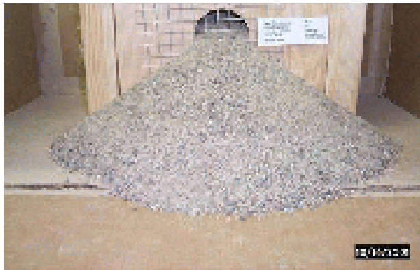
Figure 5-27. Prototype gabion wall construction showing small rock flowing easily through rebar.
