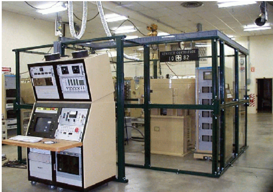
Figure 5-46. Patented polycarbonate/Unistrut® security barrier protects workers from flying debris.
