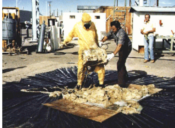
Figure 5-19. Attacker attempting to remove object covered in sticky foam.
