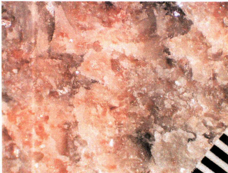
Figure 7. The pinkish-beige portions consist of medium to coarse-grained calcite that contains inclusions of hematite 'dust.' Millimeter scale.
