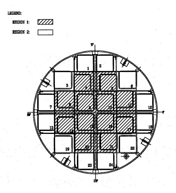
Figure 2.1-2 Fuel Loading Regions - MPC-24E/24EF
