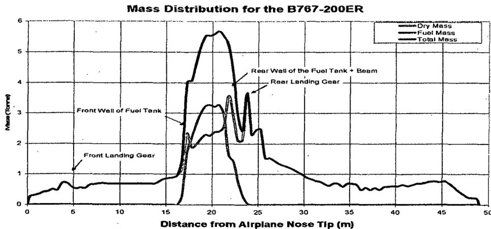
Figure 3. Mass Distribution for a Boeing 767-200ER.
