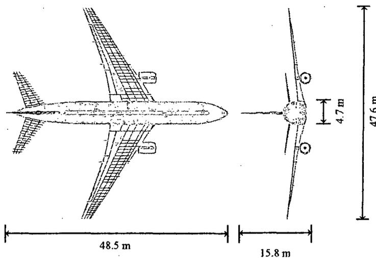
Figure 2. Dimensions of a Boeing 767-200ER.
