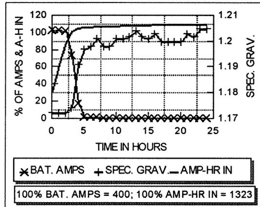
Fig.1 Recharge after Performance Test of Battery S2A
