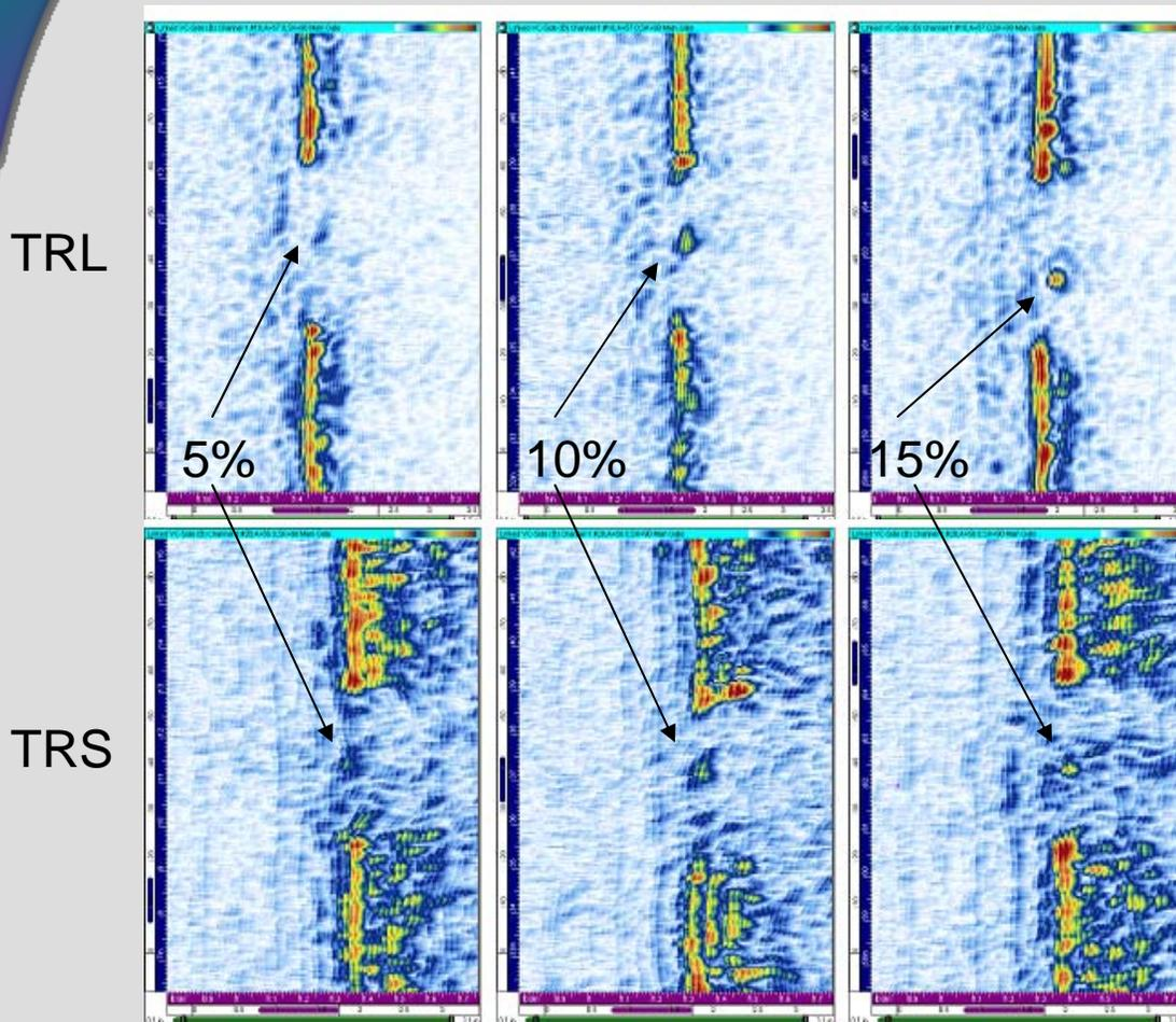
► Responses for small implanted TF cracks from far-side of weld
