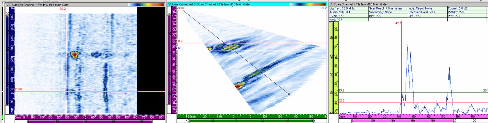
Far-side response for Flaw A – no tip diffracted signal
