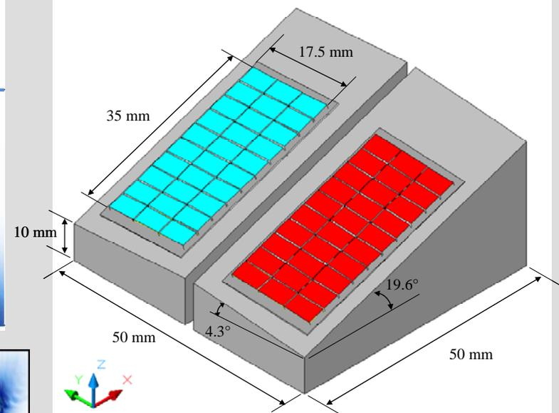
New probe design for detection of IGSCC from far-side
