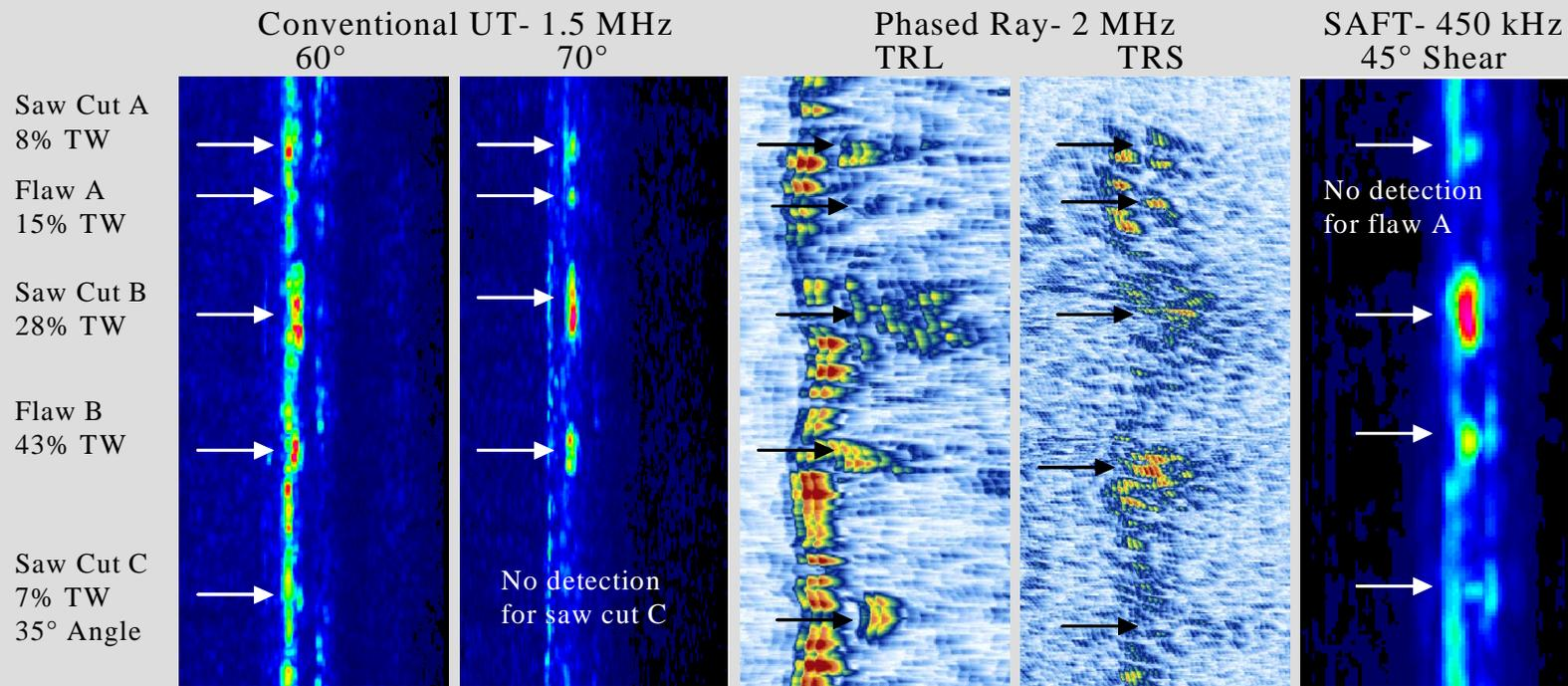
Comparison of typical responses from automated conventional UT, Phased array, and low-frequency SAFT; note TRL phased array showed best overall performance.
