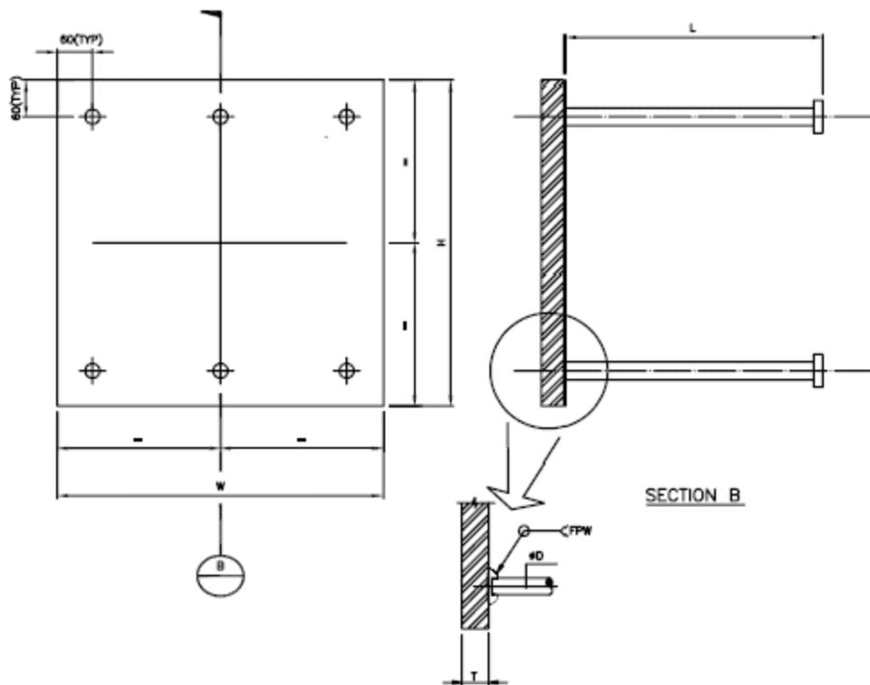
Figure 3.8-4. Typical External Containment Plate Support with Embedment
