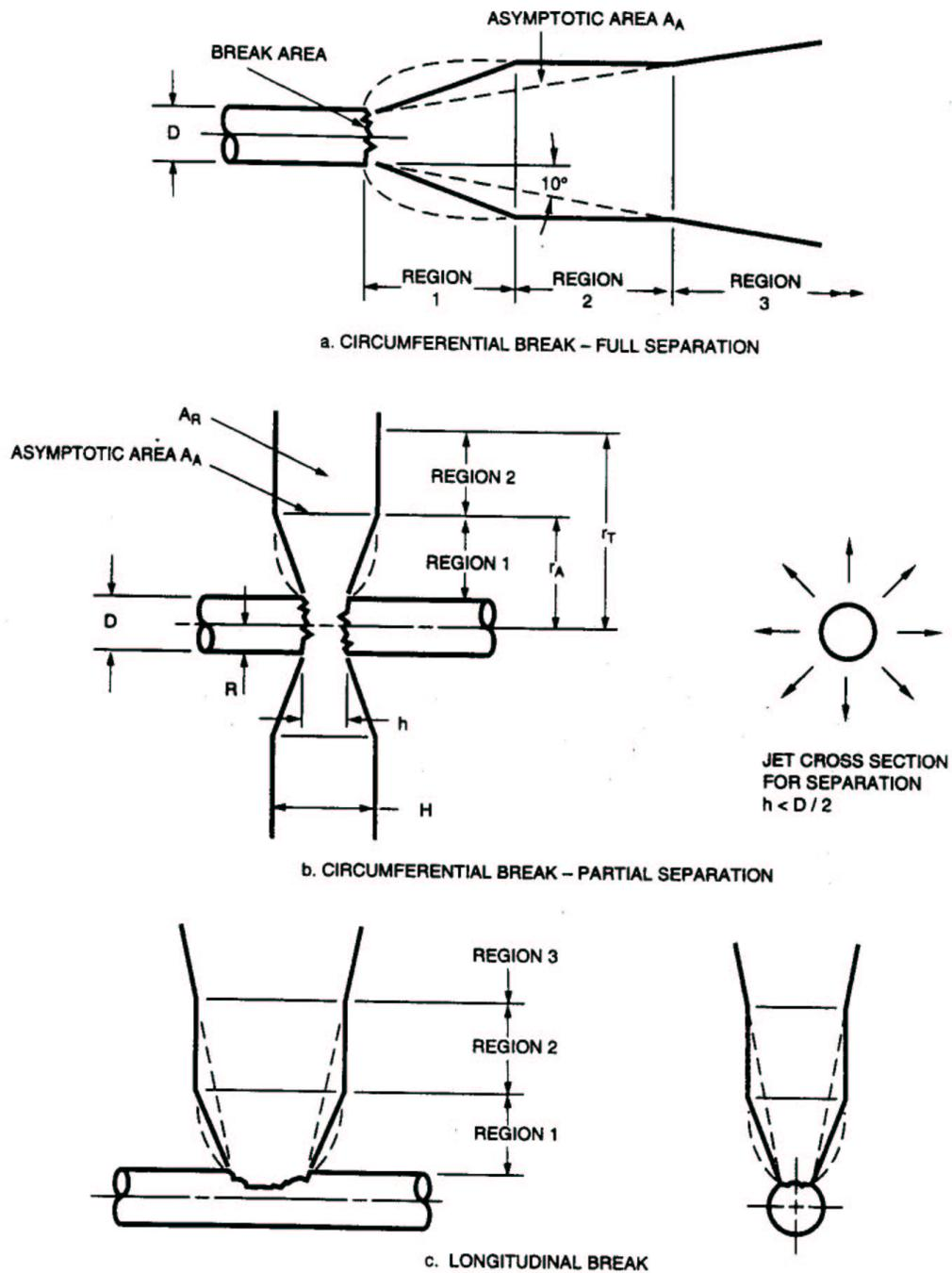
Figure 3.6-1. Jet Characteristics
