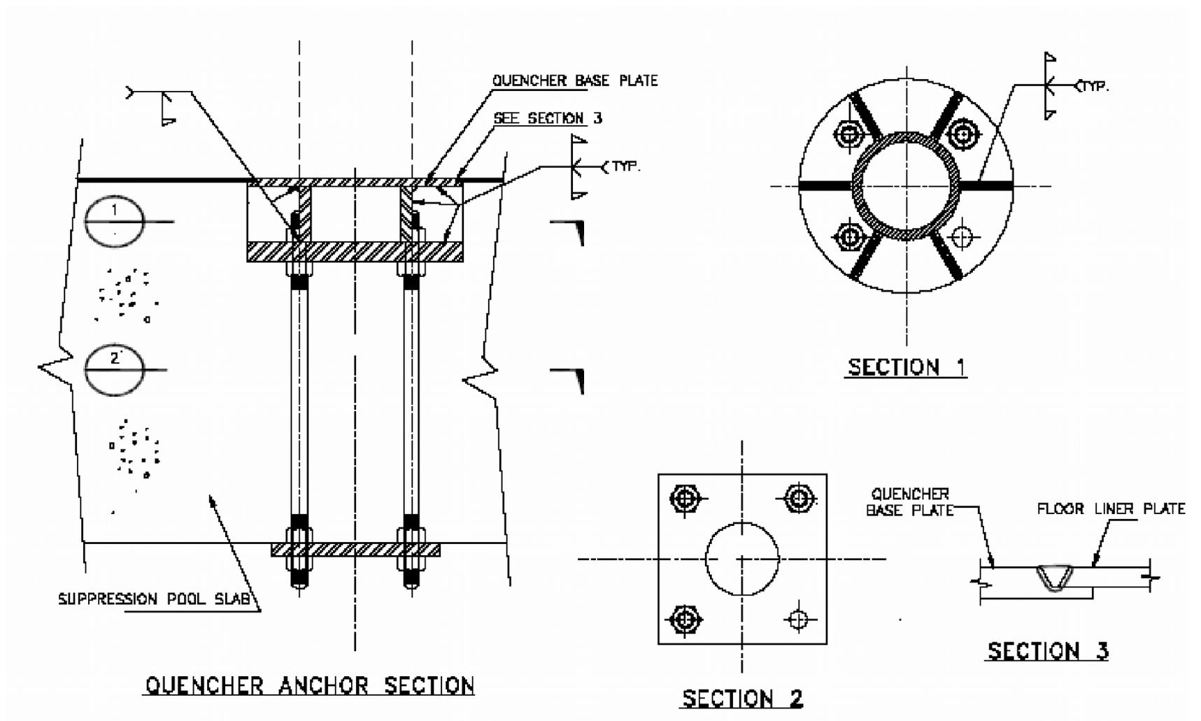
Figure 3.8-5. Quencher Anchorage
