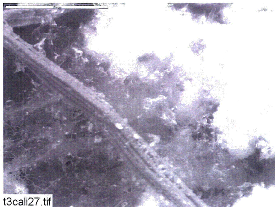
Figure H-19. ESEM image magnified 500 times for the interior of a Test#3, Day-30 raw cal-sil sample submerged in the birdcage. (T3Call27)
