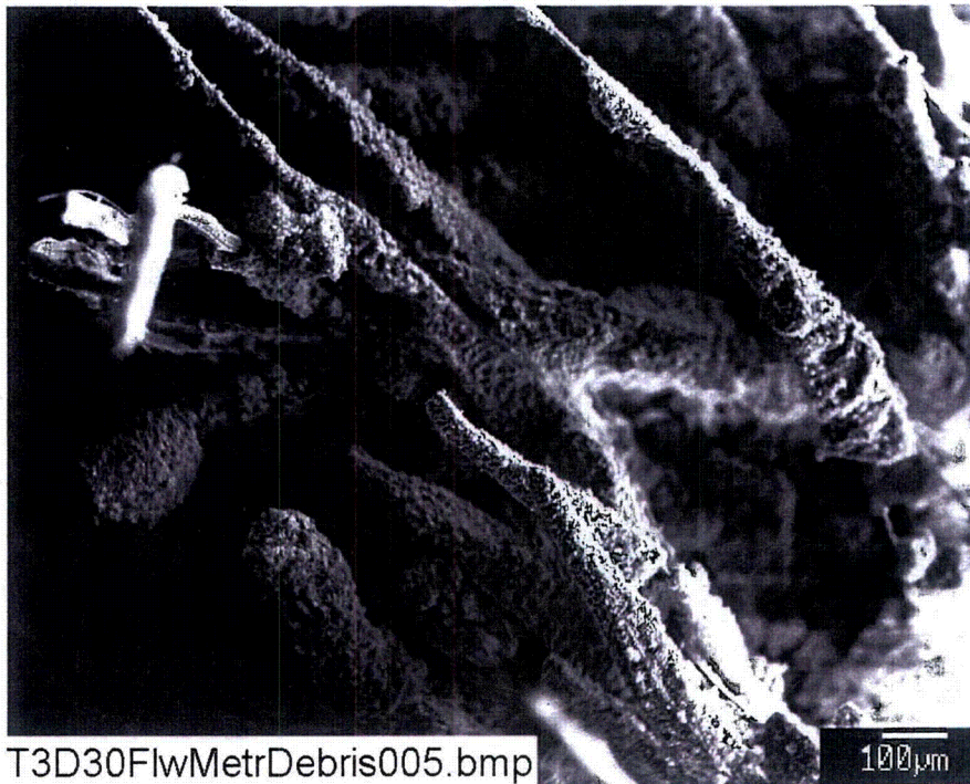
Figure F-1. SEM image magnified 80 times for Test #3, Day-30 debris within the flow meter. (T3D30FlwMetrDebris005)
