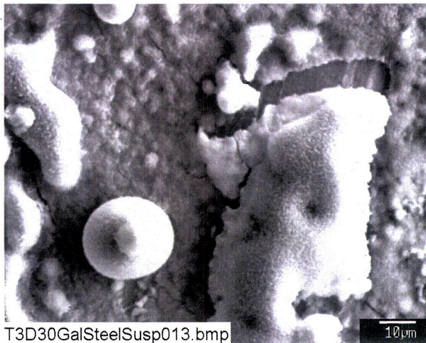
Figure E3-2. SEM image magnified 1000 times for a Test #3, Day-30 suspended galvanized steel coupon. (T3D30GalSteelSusp013)
