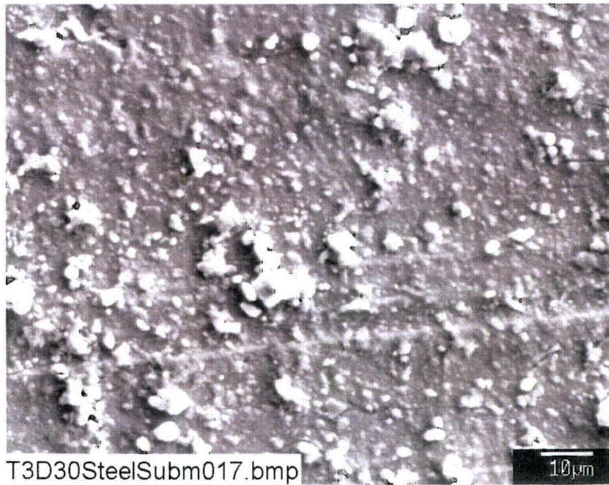
Figure E4-14. SEM image magnified 1000 times for a Test #3, Day-30 submerged carbon steel coupon. (T3D30SteelSubm017)
