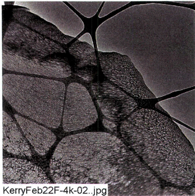
Figure F2-7. Electron micrograph magnified 4000 times for a second Test #2, Day-17 filtered sample location. (KerryFeb22F-4k-02)
