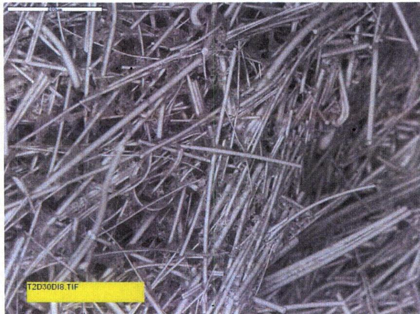
Figure D3-25. ESEM image for a Test #2, Day-30 interior fiberglass sample on the drain collar. (T2D30D18)
