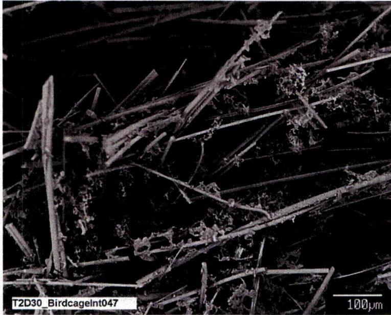
Figure D4-10. Backscattered SEM image for a Test #2, Day-30 interior fiberglass sample within the birdcage. The atomic number of the deposits is similar to that of the fiberglass. (T2D30\_BirdcageInt047)
