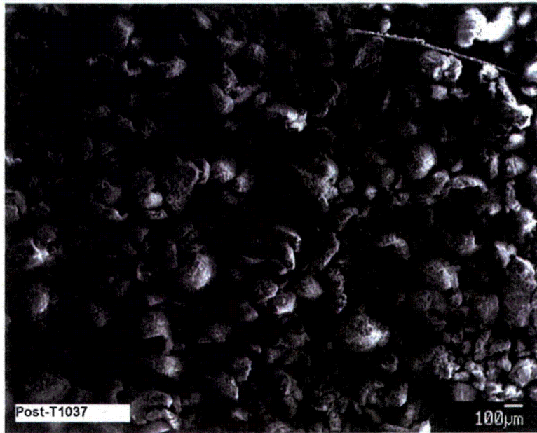
Figure D-76. Day-30, post-T1-sample-Sed1 SEM-SE image (Post-T1037) magnified 40 times; overview of particles.
