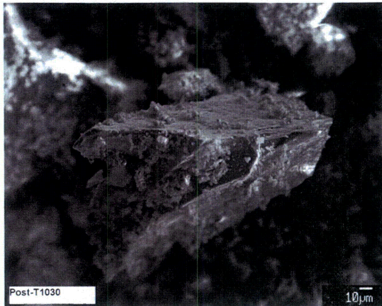
Figure D-60. Day-30, post-T1-sample-CD1 SEM-SE image (Post-T1030) magnified 400 times on the particle in the center of image Post-T1029 (see Figure D-58).
