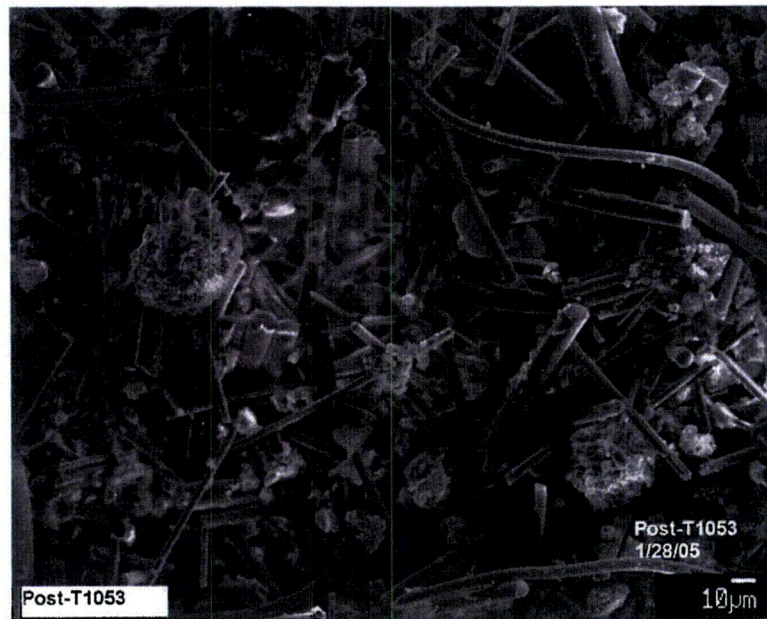
Figure D-94. Day-30, post-T1-sample-Sed2A SEM-SE image (Post-T1053) magnified 370 times on two large particles in image Post-T1052 (see Figure D-93).
