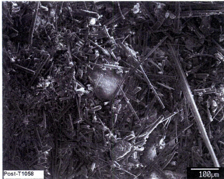
Figure D-102. Day-30, post-T1-sample-Sed2A SEM-SE image (Post-T1058) of the high-Z particles analyzed in EDS counting spectra EDS-21 and -22, magnified 150 times, as shown in Figure D-99 and Figure D-101.
