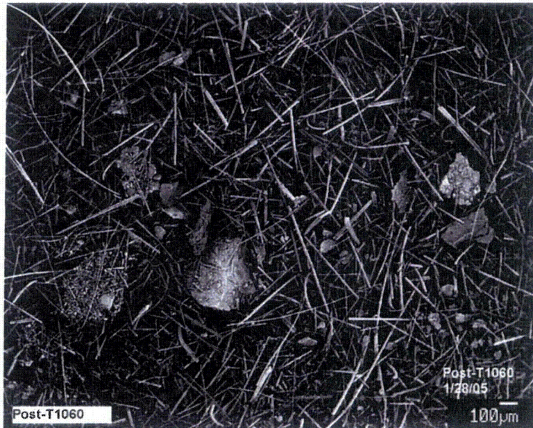
Figure D-104. Day-30, post-T1-sample-Sed2B SEM-BSE image (Post-T1060) magnified 40 times on the same particles shown above.
