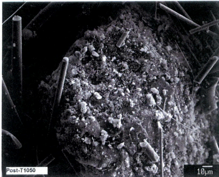
Figure D-91. Day-30, post-T1-sample-Sed2A SEM-SE image (Post-T1050) higher magnification of a representative large particle in image Post-T1049, as shown in Figure D-90.
