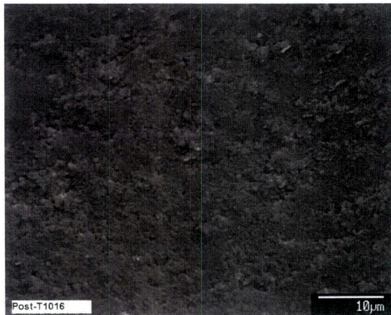
Figure D-27. End-test archive, post-T1 sample #3 SEM image (POST-T1016) magnified 2000 times on the surface of the concoidal fracture, as shown in Figure D-26.
