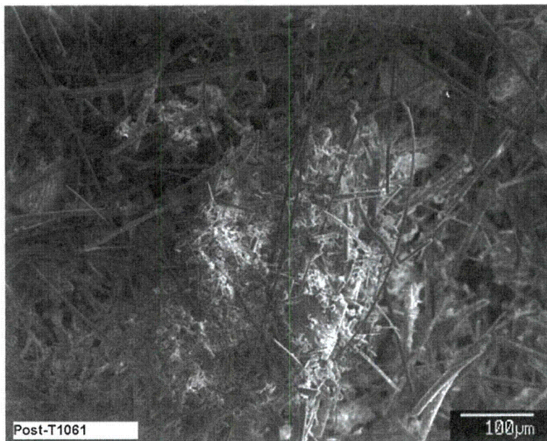
Figure D-108. Day-30, post-T1-sample-Sed2B SEM-SE image (Post-T1061) magnified 160 times on the particles and fibers at left side of image Post-T1059 (see Figure D-103).
