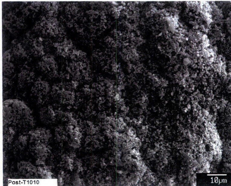
Figure D-18. End-test archive, post-T1 sample #3 SEM image (POST-T1010) magnified 1000 times on the white surface in Figure D-17, showing a coarsely granular structure on the underside of the smooth brown fragments.
