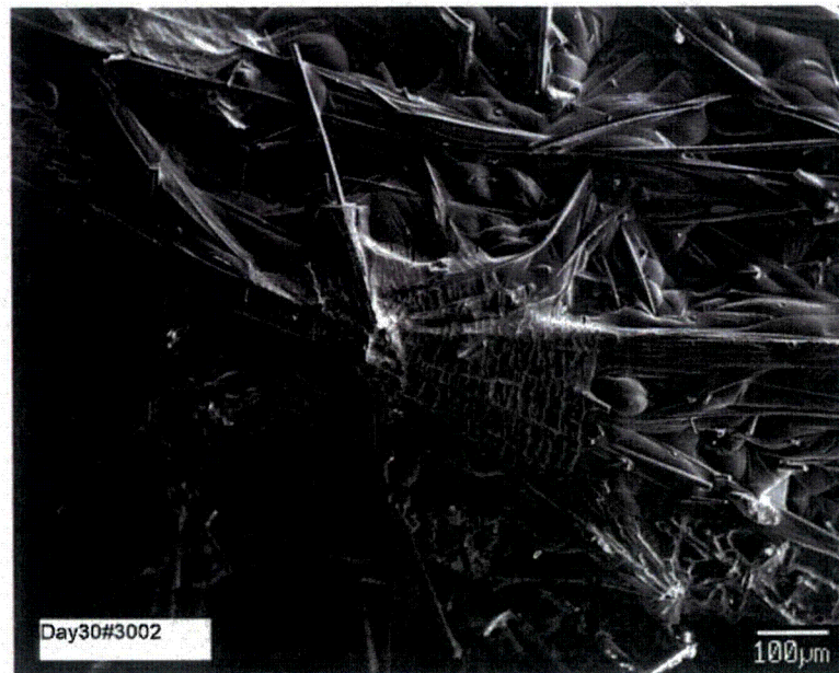
Figure C-44. Day-30, sample #3 SEM image (#3002) magnified 100 times on the fiberglass with surface coating.
