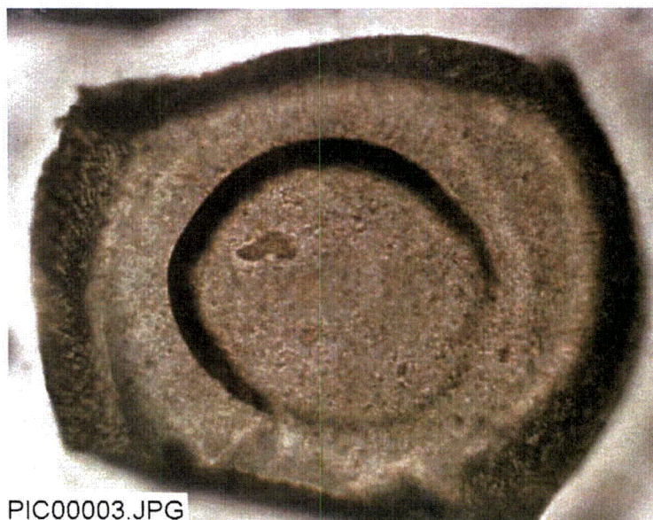
Figure C-5. Plane-polarized optical microscope photograph (PIC00003) for the Day-21 precipitation from the filtered water sample magnified 50 times on the single fragment with contraction dome, as shown in Figure C-4.
