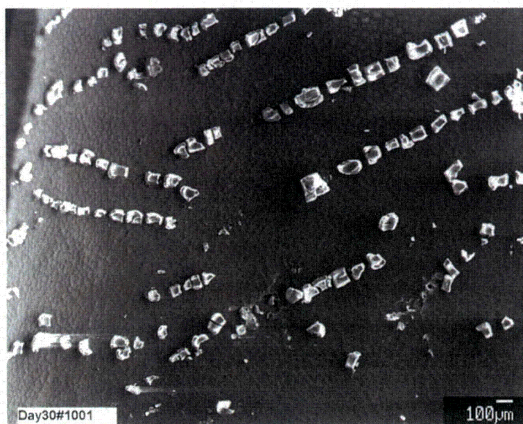
Figure C-20. Day-30, sample #1 SEM image (#1001) magnified 40 times on the string of blocky fragments.
