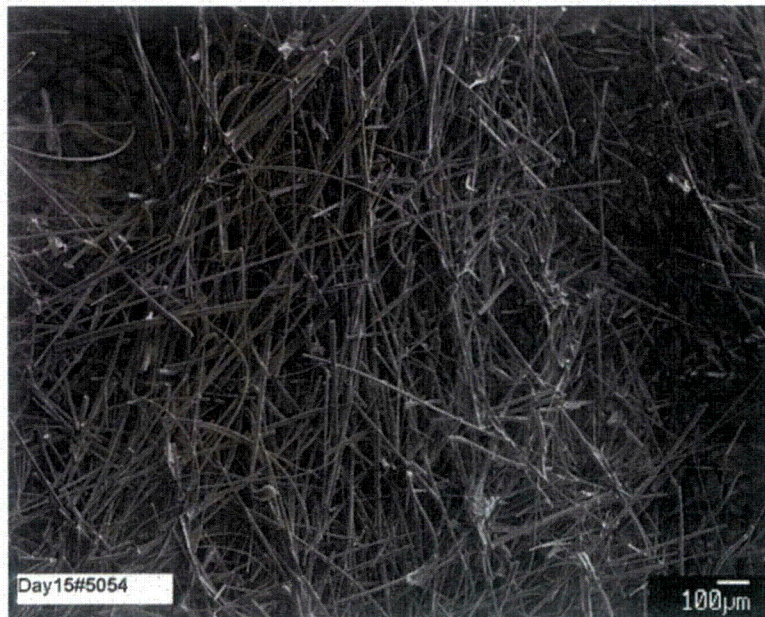
Figure B-88. Day-15, sample #5 SEM image (#5054) magnified 50 times on fiberglass in a new area.
