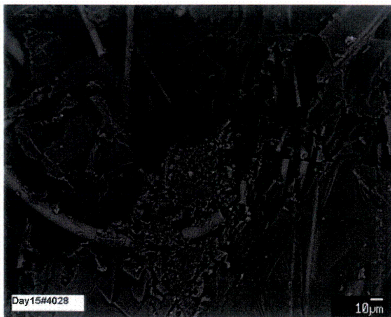
Figure B-48. Day-15, sample #4 SEM image (#4028) magnified 370 times; BSE close-up of the upper center of Figure B-46.
