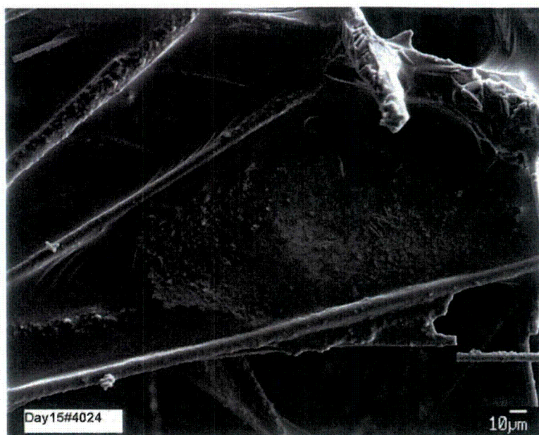
Figure B-41. Day-15, sample #4 SEM image (#4024) magnified 370 times on the film with particles.
