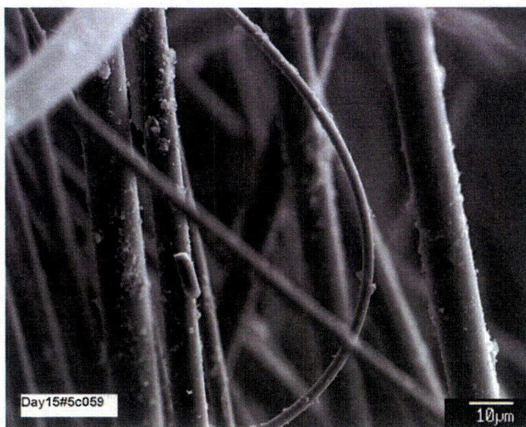
Figure B-93. Day-15, sample #5C SEM image (#5C059) magnified 1000 times on fiberglass in the different area, as shown in Figure B-91.
