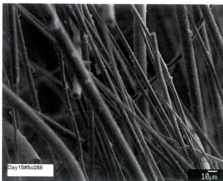
Figure B-92. Day-15, sample #5C SEM image (#5C058) magnified 500 times on fiberglass in the same area as in Figure B-91.
