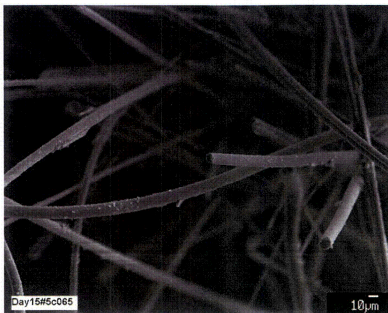
Figure B-101. Day-15, sample #5C SEM image (#5C065) magnified 300 times on fiberglass in a new area of the sample.
