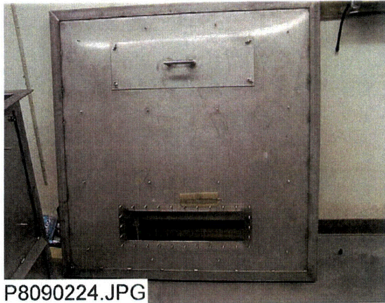
Figure 8. The cover lid of the ICET tank showing the top observation window (lower) and top access hatch with handle (upper).
