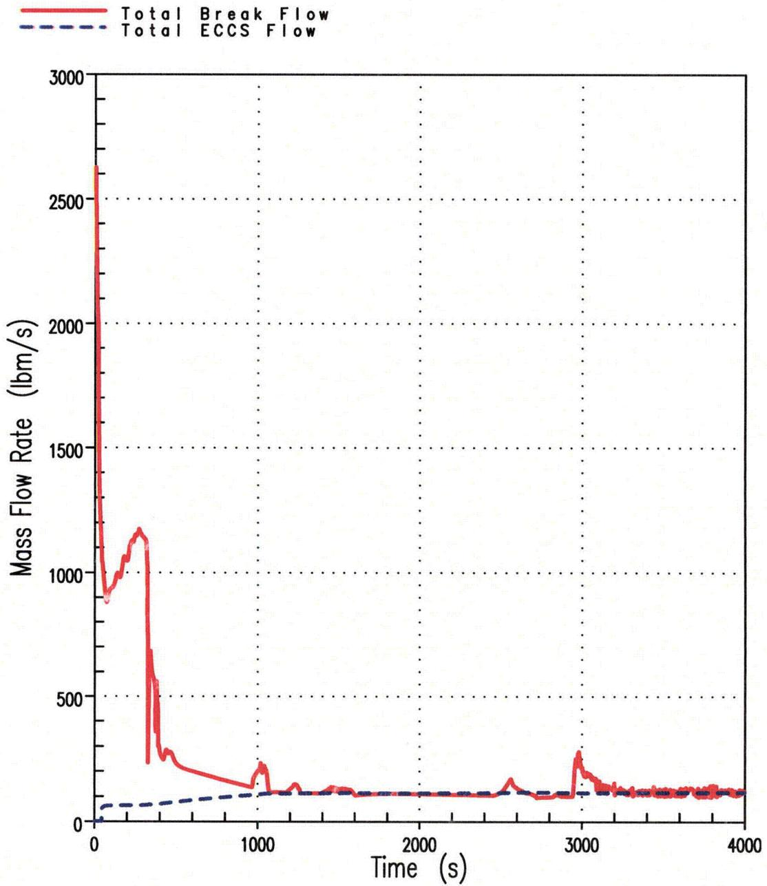
Figure 2D Break Flow Rate vs. Total ECCS Flow Rate
