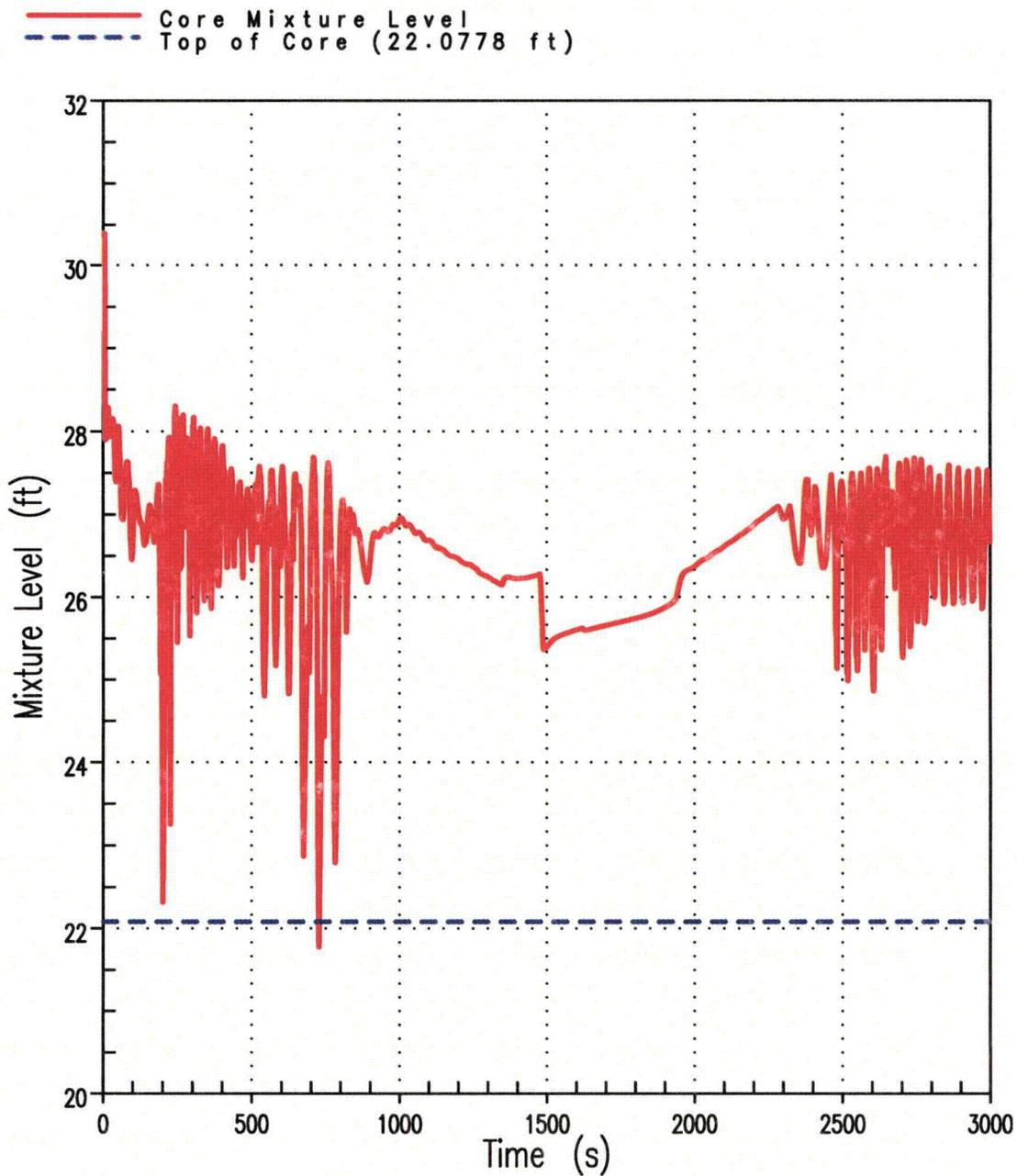
Figure 11B Core Mixture Level 8.75-Inch Break (Unit 2)
