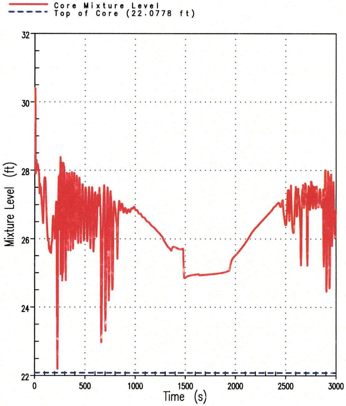
Figure 7B Core Mixture Level 8.75-Inch Break (Unit 1)
