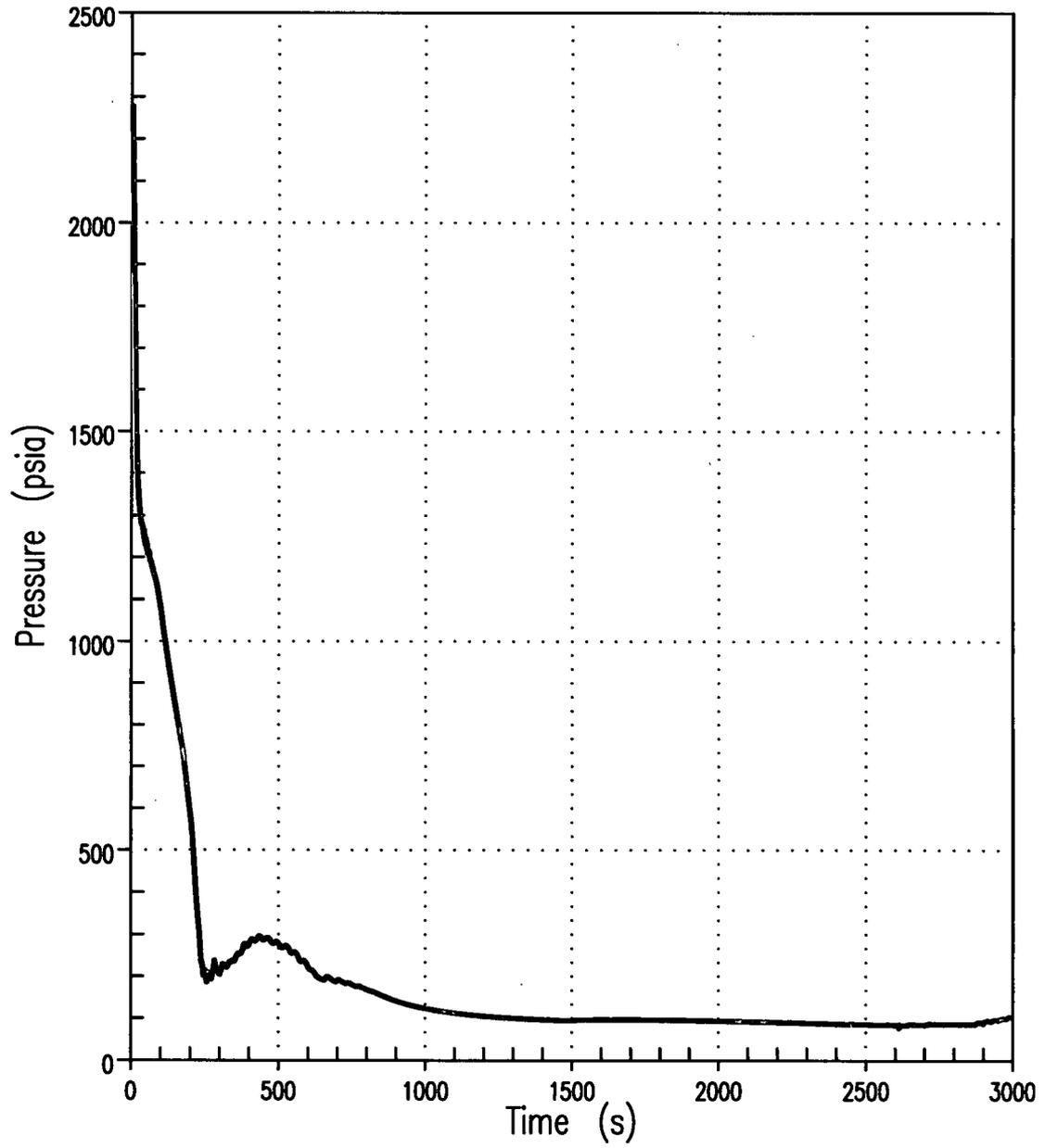
**Figure 7A RCS Pressure 8.75-Inch Break (Unit 1)**
