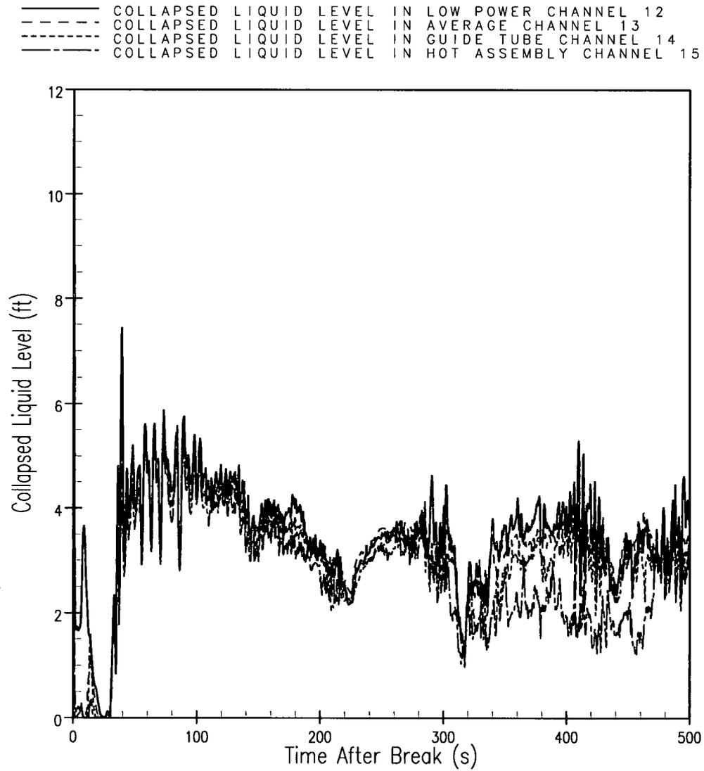
**Figure 13 – Comanche Peak Unit 1 Core Collapsed Liquid Levels for the Limiting PCT Case**
