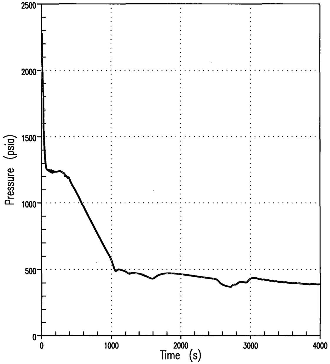
**Figure 2A** RCS Pressure 4-Inch Break (Unit 1)
