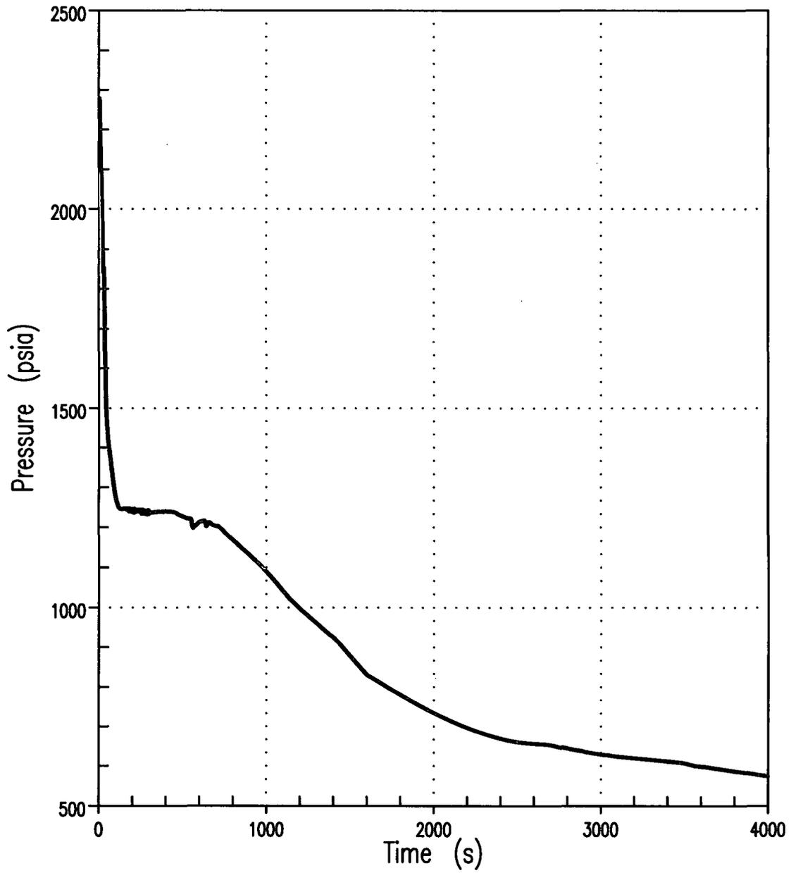
Figure 5A RCS Pressure 3-Inch Break (Unit 1)
