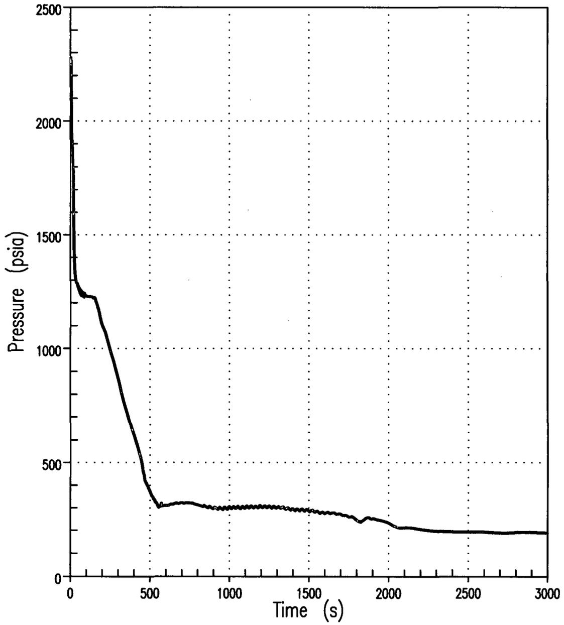
Figure 6A RCS Pressure 6-Inch Break (Unit 1)
