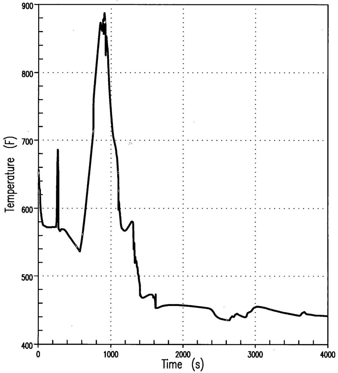
Figure 3F Core Exit Vapor Temperature 4-Inch Break (Unit 2)
