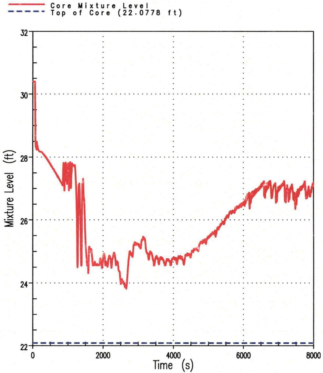
Figure 4B Core Mixture Level 2-Inch Break (Unit 1)
