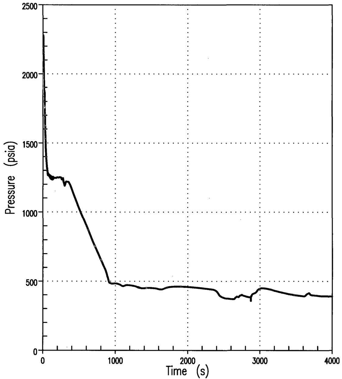
Figure 3A RCS Pressure 4-Inch Break (Unit 2)
