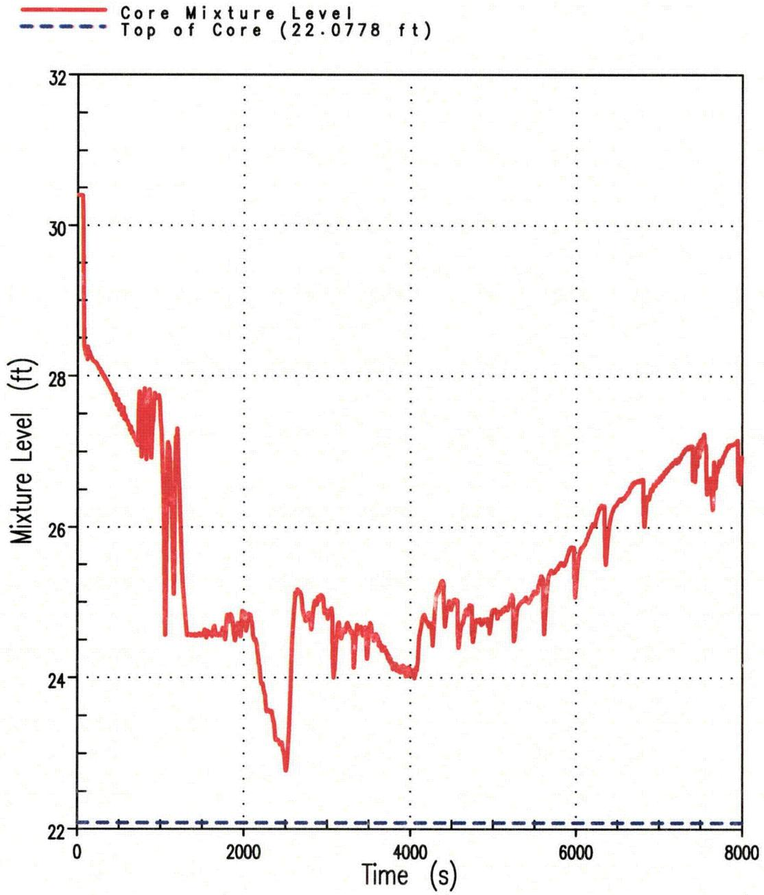
Figure 8B Core Mixture Level 2-Inch Break (Unit 2)
