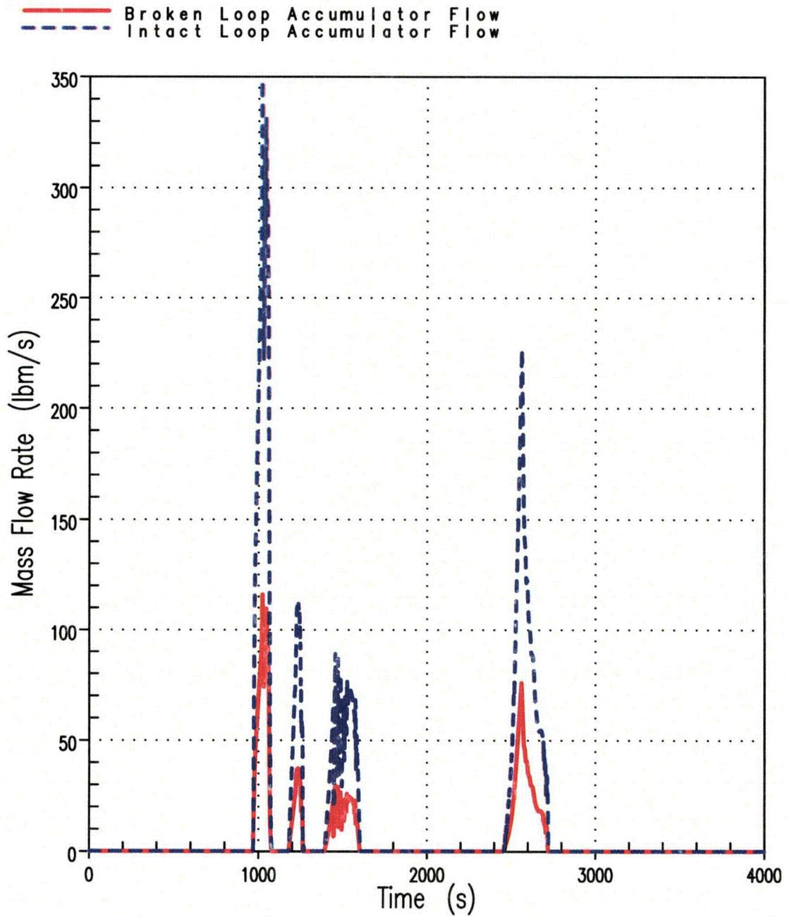
**Figure 2E Broken Loop and Intact Loop Accumulator Flow Rate
