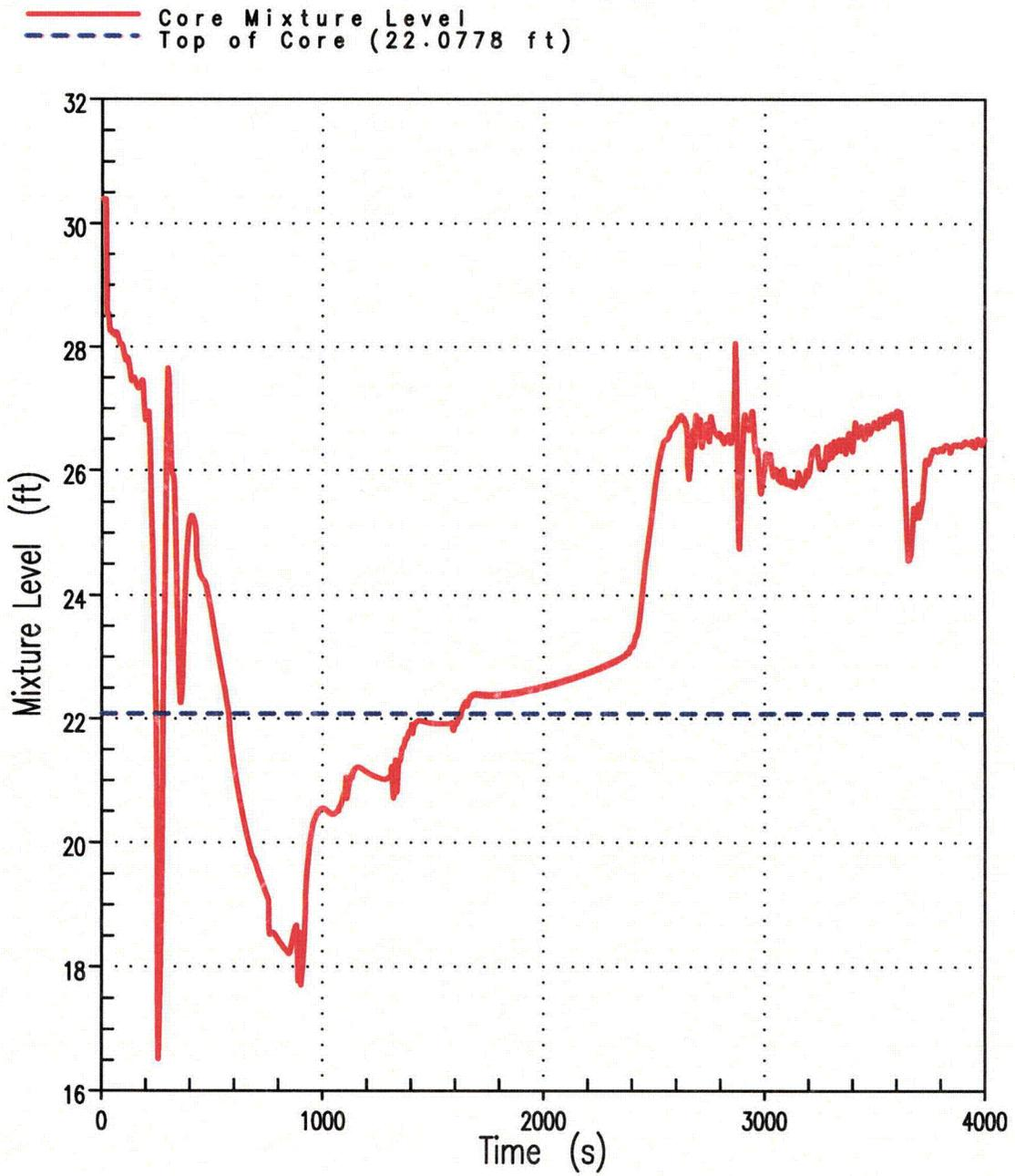
Figure 3B Core Mixture Level 4-Inch Break (Unit 2)
