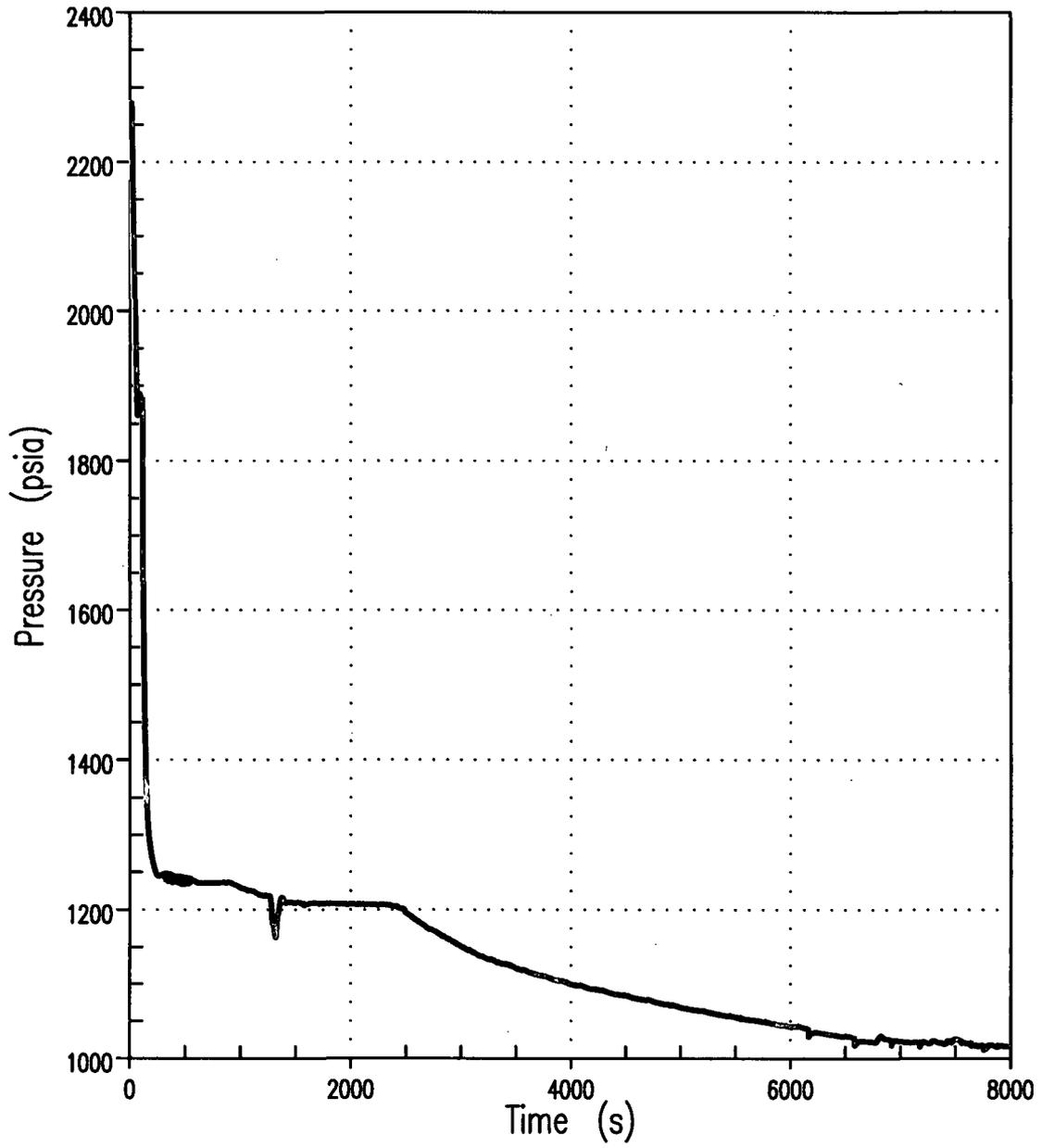
Figure 4A RCS Pressure 2-Inch Break (Unit 1)
