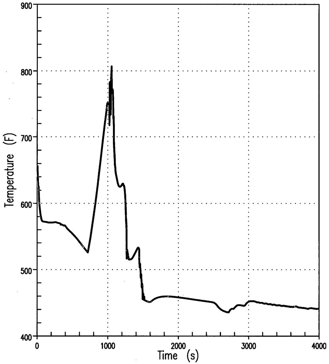
Figure 2F Core Exit Vapor Temperature 4-Inch Break (Unit 1)
