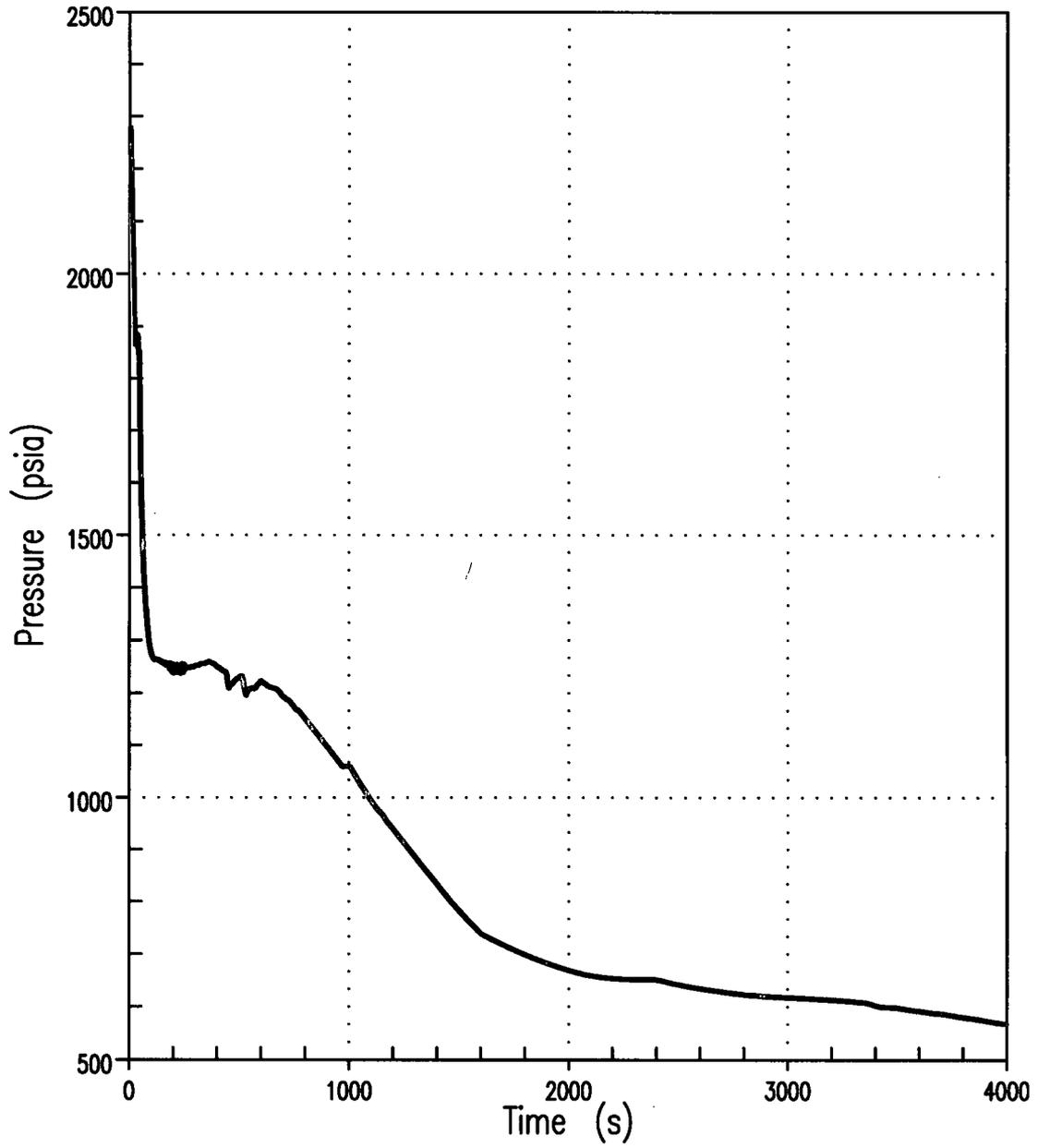
Figure 9A RCS Pressure 3-Inch Break (Unit 2)
