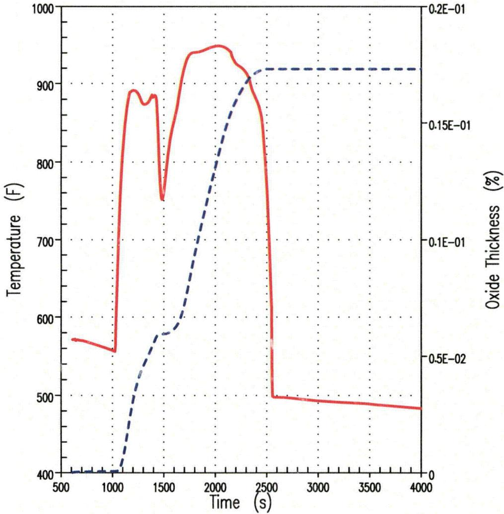
Figure 5C Hot Rod Clad Temperature and ZrO<sub>2</sub> Thickness at PCT Elevation 3-Inch Break (Unit 1)
