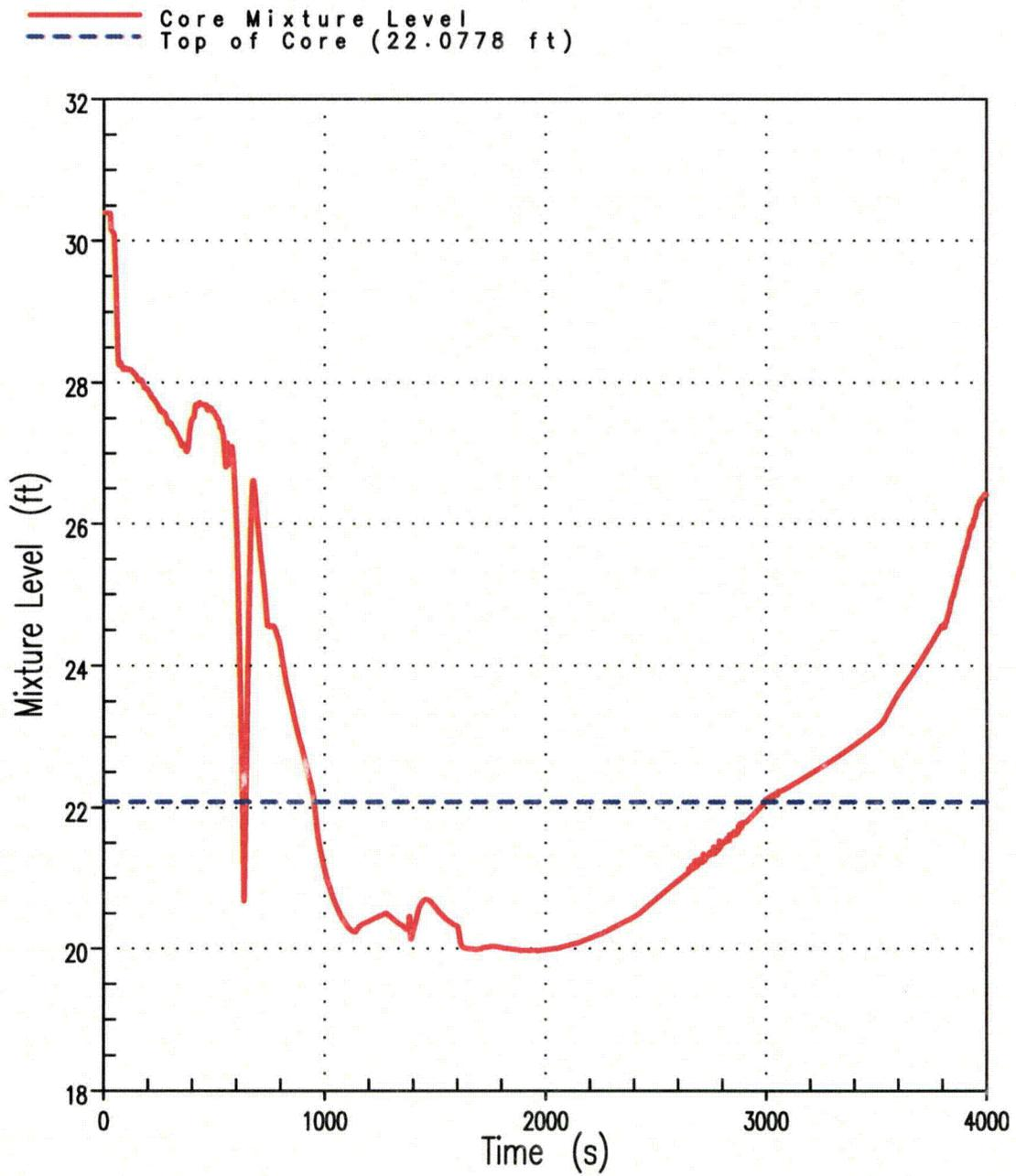
Figure 5B Core Mixture Level 3-Inch Break (Unit 1)
