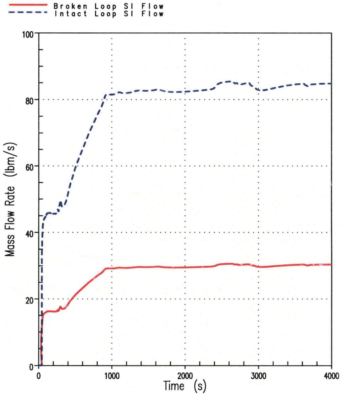
Figure 3C Broken Loop and Intact Loop Pumped Safety Injection Flow Rate
