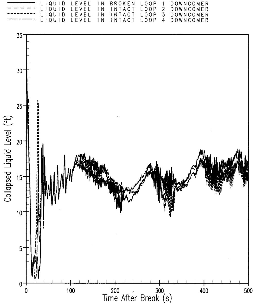
**Figure 12 – Comanche Peak Unit 1 Downcomer Collapsed Liquid Levels for the Limiting PCT Case**
