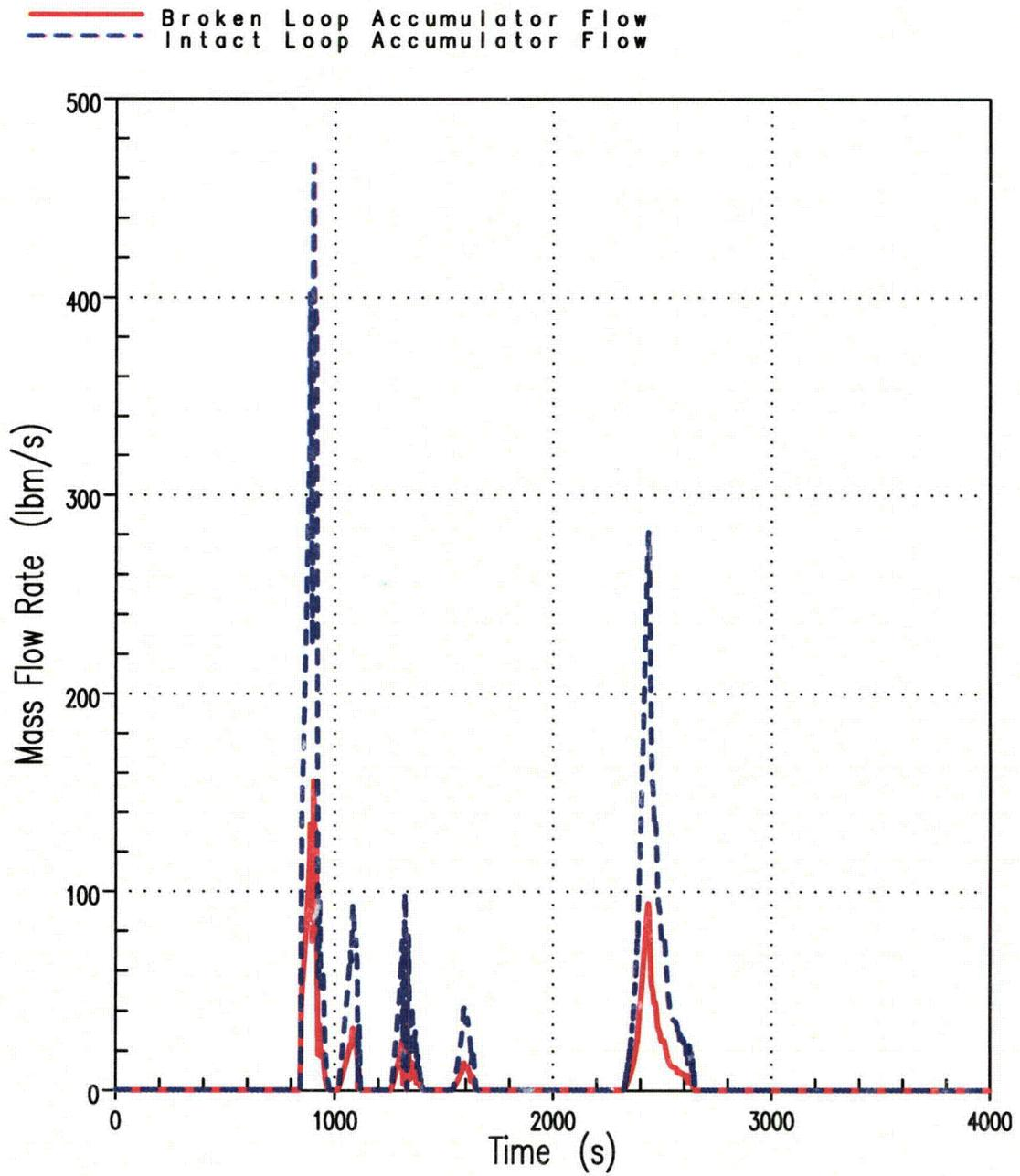
Figure 3E Broken Loop and Intact Loop Accumulator Flow Rate
