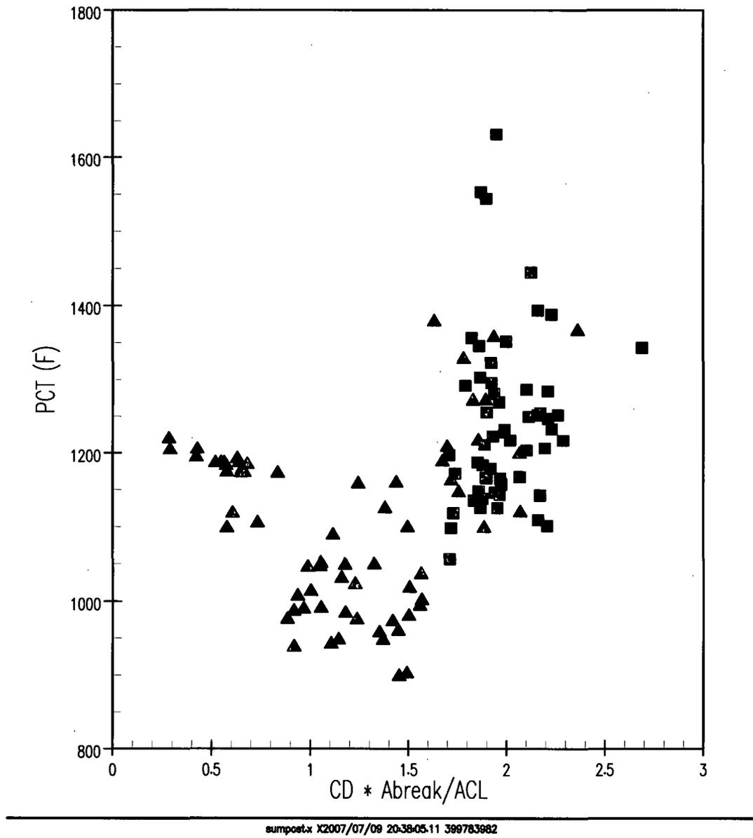
**Figure 1 – Comanche Peak Unit 2 HOTSPOT PCT versus Effective Break Area Scatter Plot (CD = Discharge Coefficient, Abreak = Break Area, ACL = Cold Leg Area)**
