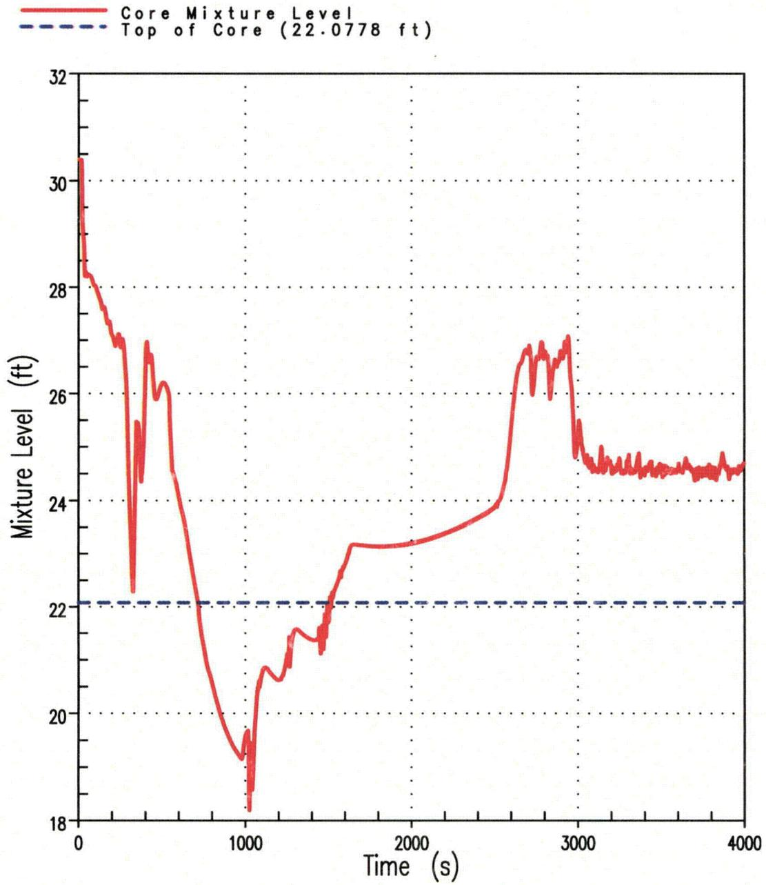
Figure 2B Core Mixture Level 4-Inch Break (Unit 1)
