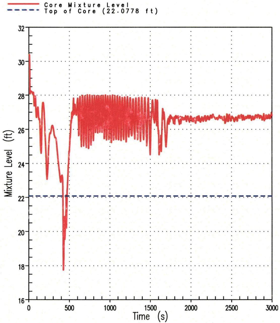
Figure 10B Core Mixture Level 6-Inch Break (Unit 2)
