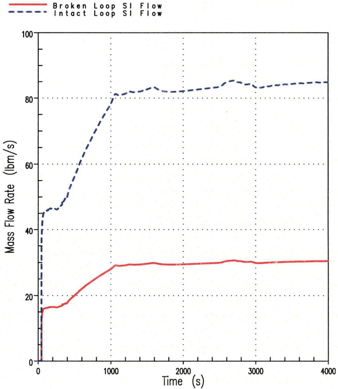
Figure 2C Broken Loop and Intact Loop Pumped Safety Injection Flow Rate
