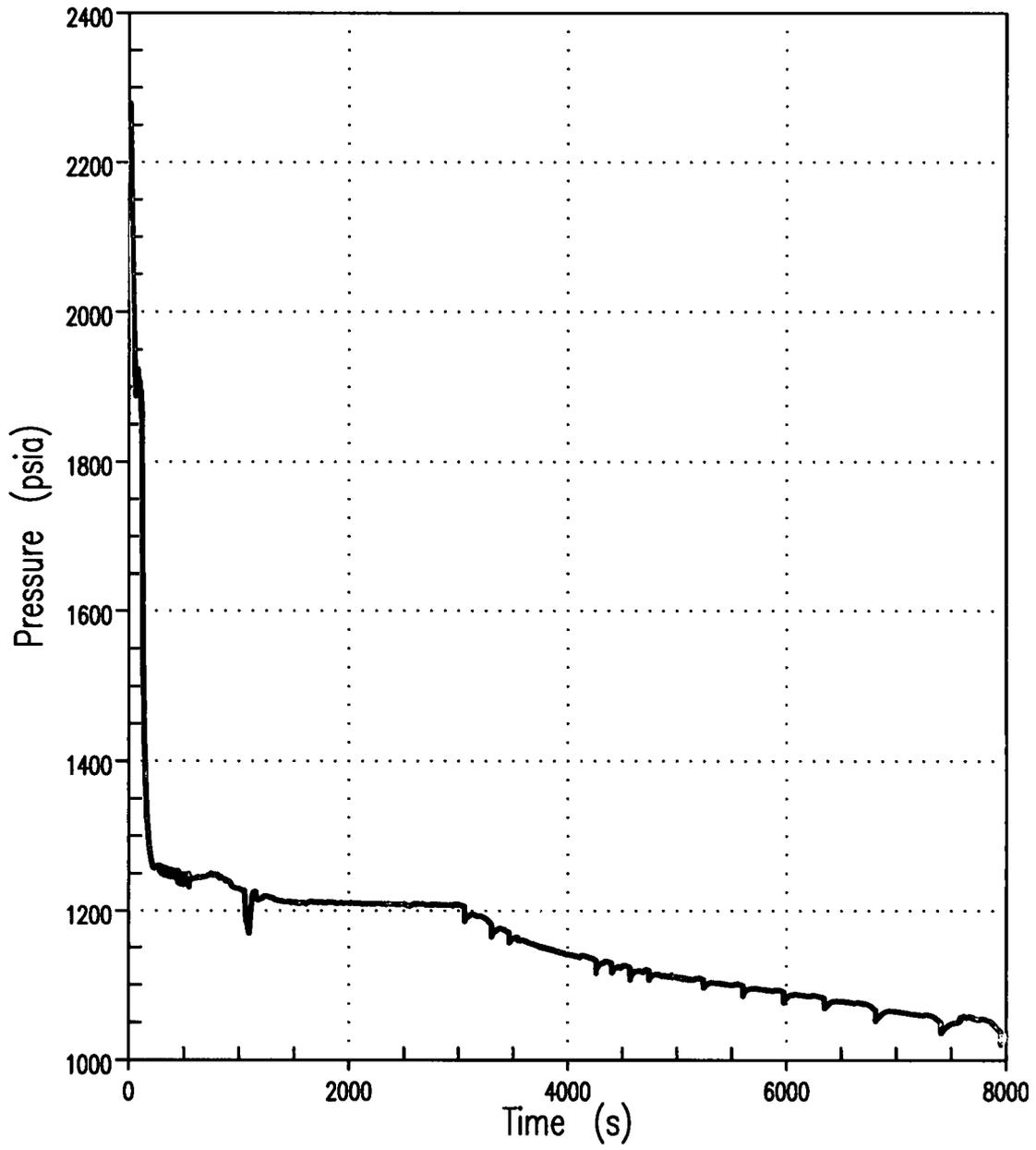
Figure 8A RCS Pressure 2-Inch Break (Unit 2)
