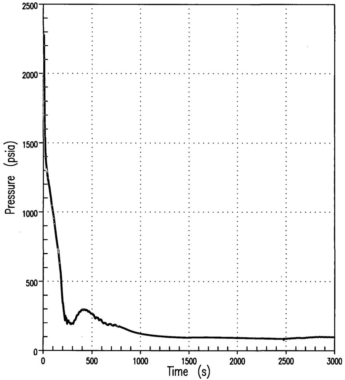
Figure 11A RCS Pressure 8.75-Inch Break (Unit 2)
