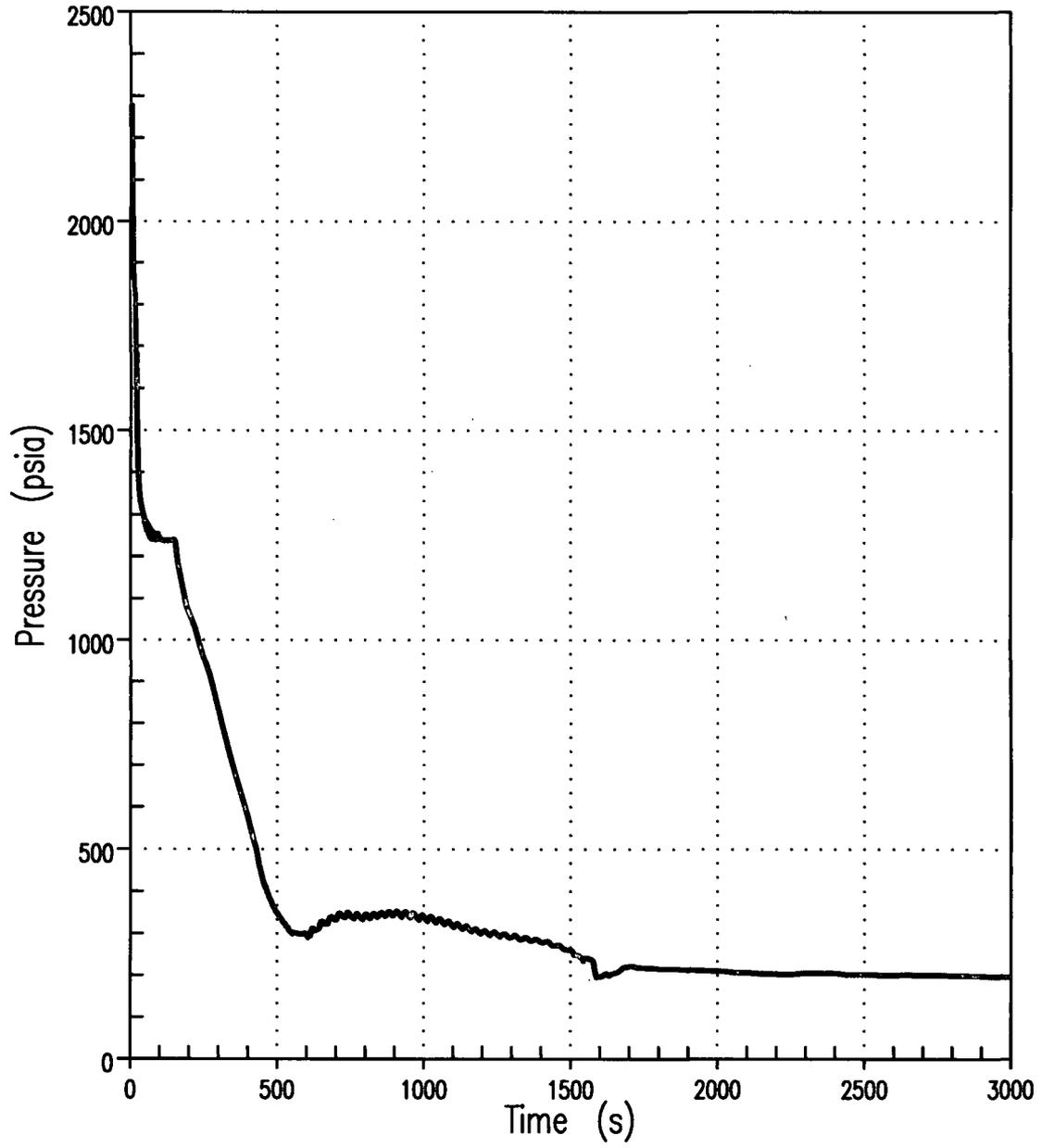
Figure 10A RCS Pressure 6-Inch Break (Unit 2)
