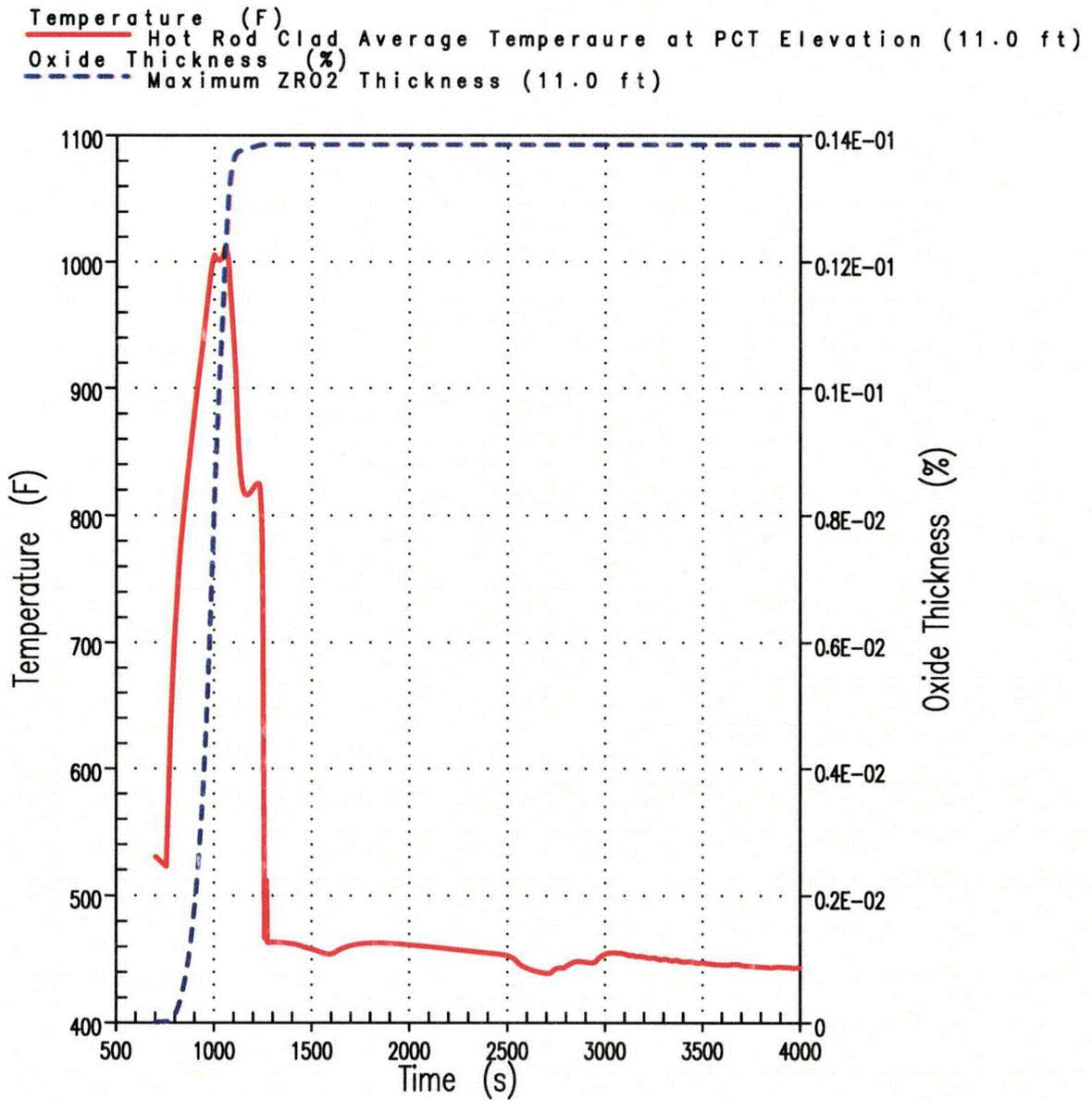
Figure 2G Hot Rod Clad Temperature and ZRO2 Thickness at PCT Elevation
