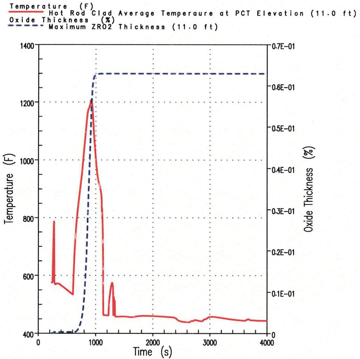
Figure 3G Hot Rod Clad Temperature and ZrO<sub>2</sub> Thickness at PCT Elevation
