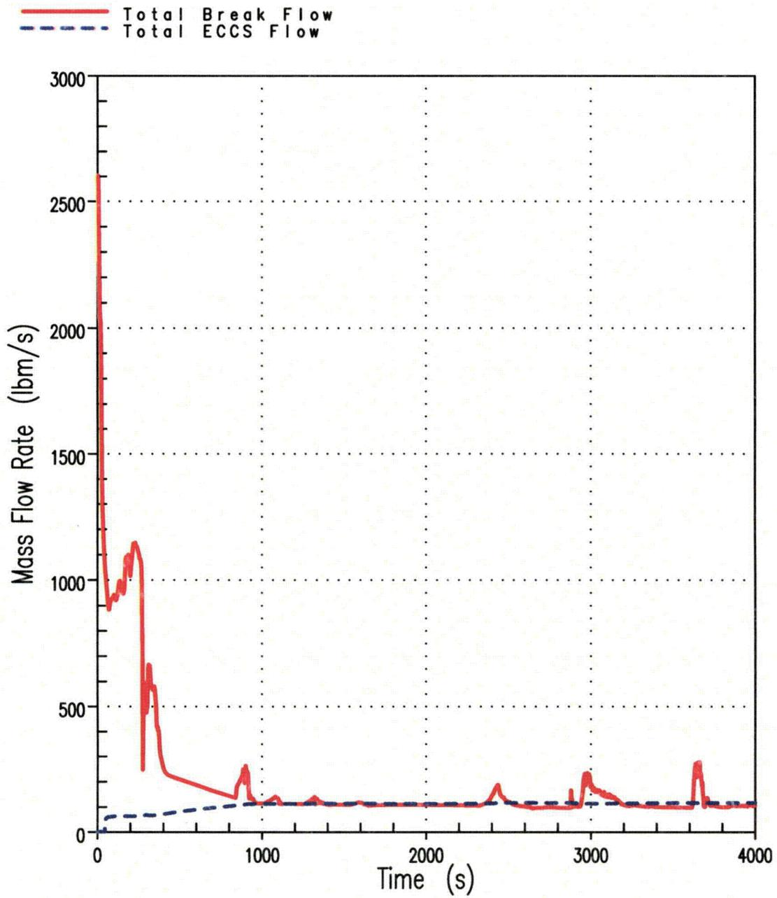
Figure 3D Break Flow Rate vs. Total ECCS Flow Rate
