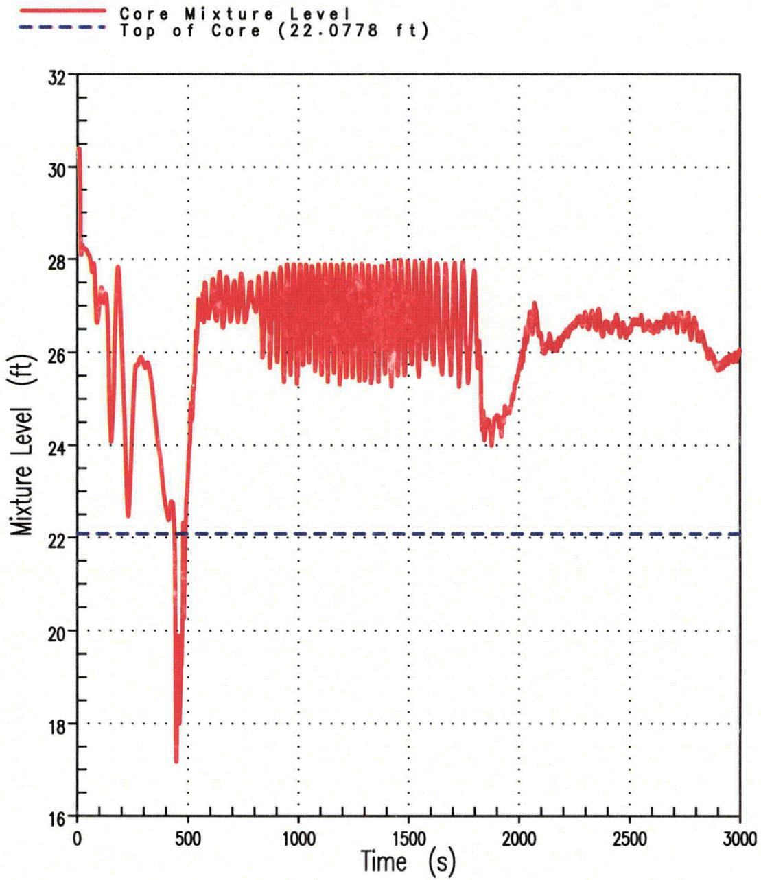
Figure 6B Core Mixture Level 6-Inch Break (Unit 1)
