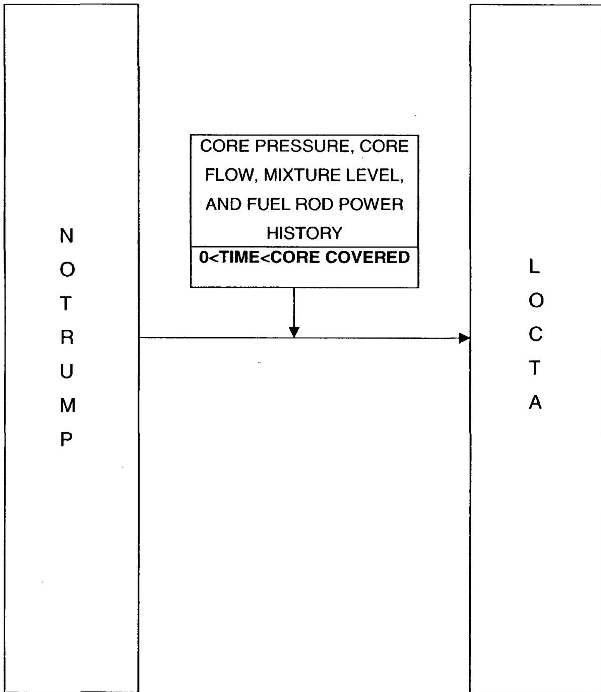
Figure 1 Code Interface Description for NOTRUMP-EM
