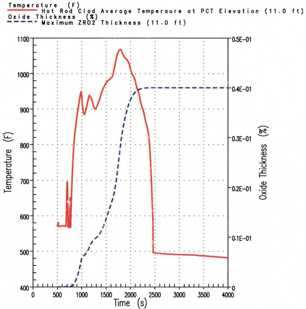
**Figure 9C Hot Rod Clad Temperature and ZrO<sub>2</sub> Thickness at PCT Elevation 3-Inch Break (Unit 2)**
