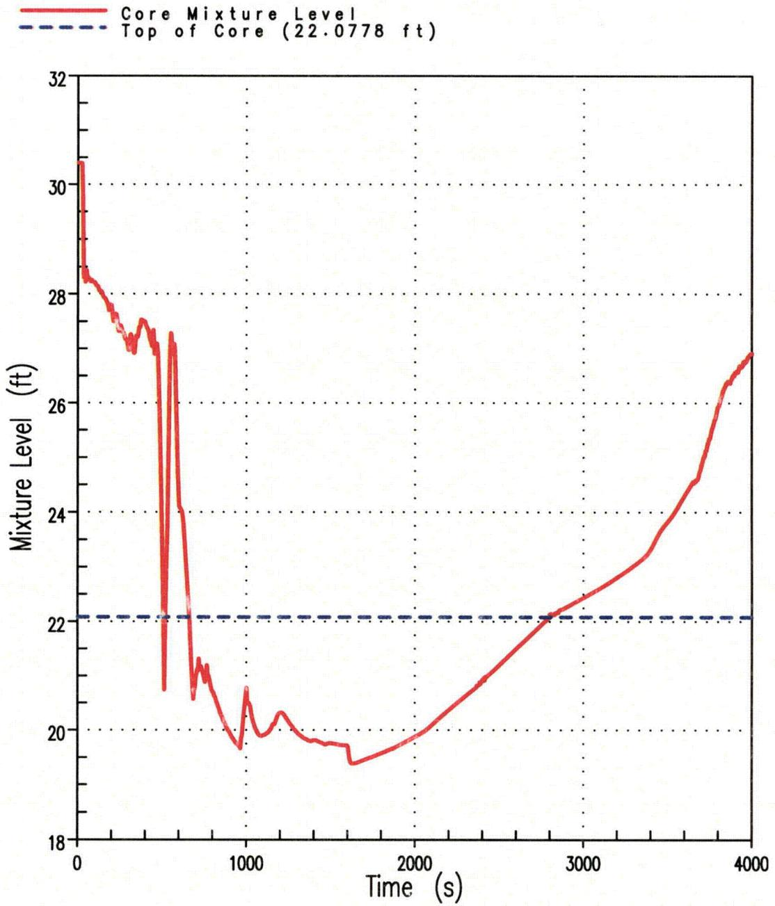
Figure 9B Core Mixture Level 3-Inch Break (Unit 2)
