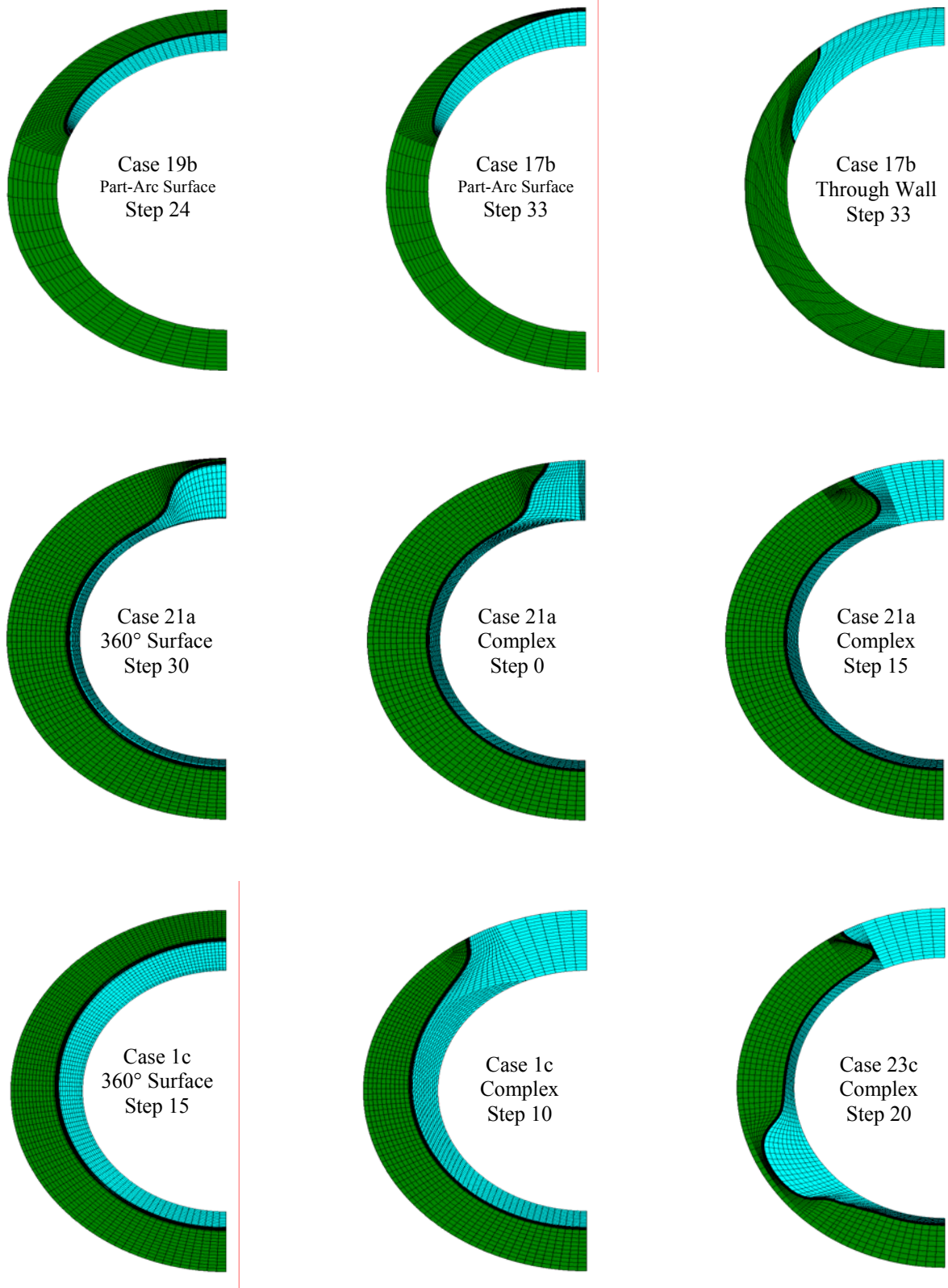
Figure 7-17 Example Crack Meshes for a Variety of Sensitivity Cases and Crack Types
