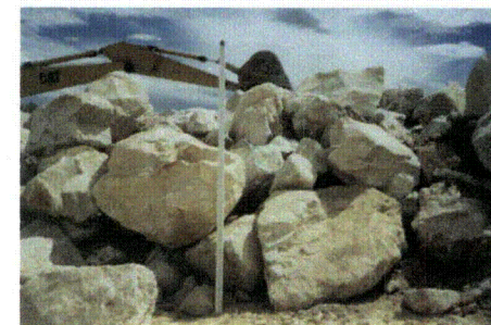
Type E Rock Depth Verification (6 feet)
