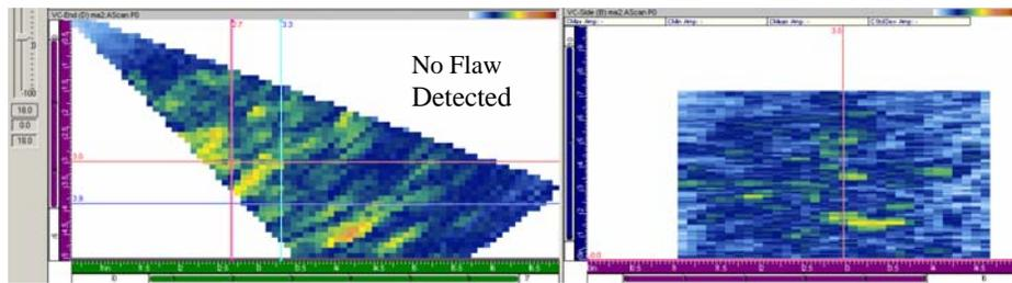
**Figure 3 Mechanical Fatigue Crack in Specimen MPE-3 As Viewed from CCSS Side at 1.0 MHz is Judged To Be Not Detected. Side View is on the Left and End View is on the Right.**
