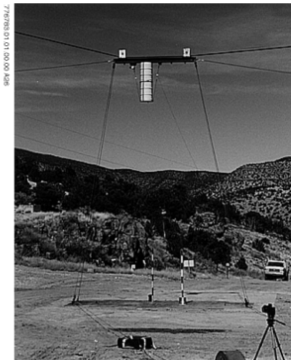
Figure 4.1-3b. Top-Impact Drop Test Set-up
