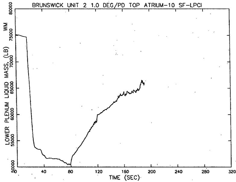
**Figure 7.19 Limiting SLO Recirculation Line Break
