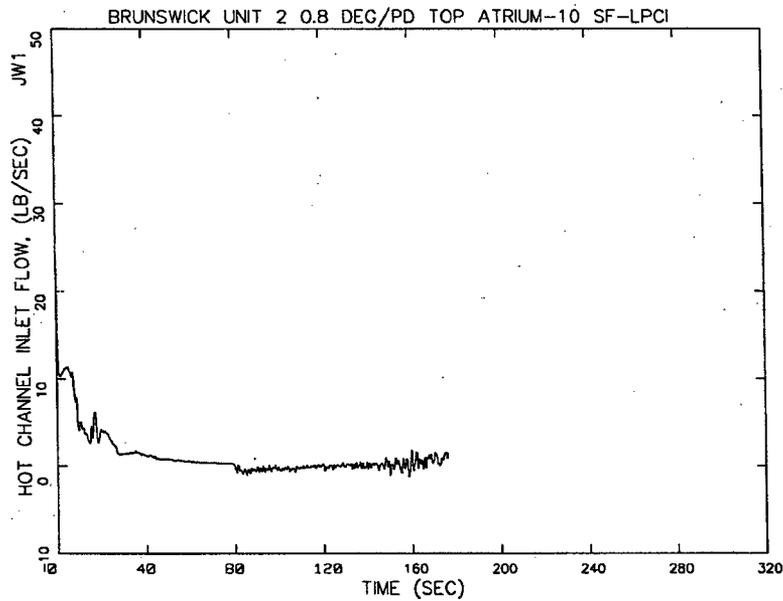
**Figure 6.20 Limiting TLO Recirculation Line Break
