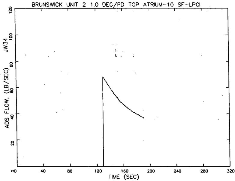
**Figure 7.11 Limiting SLO Recirculation Line Break
