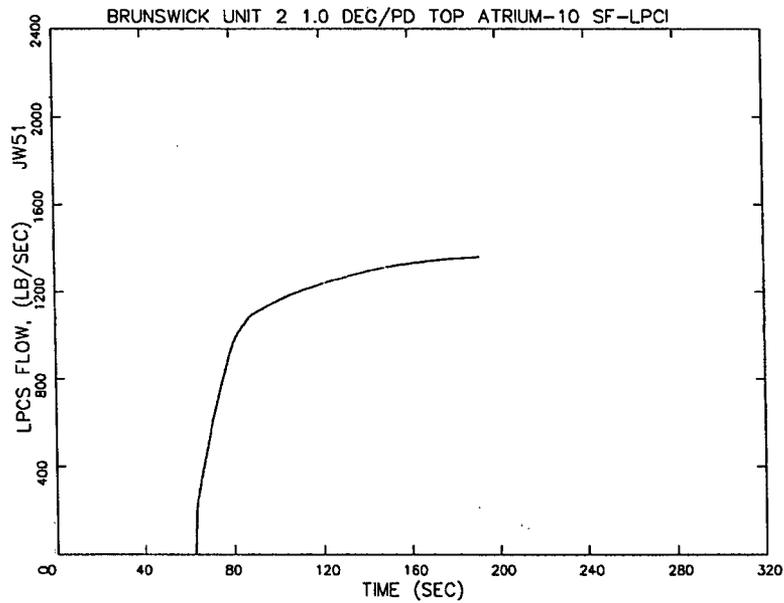
**Figure 7.12 Limiting SLO Recirculation Line Break
