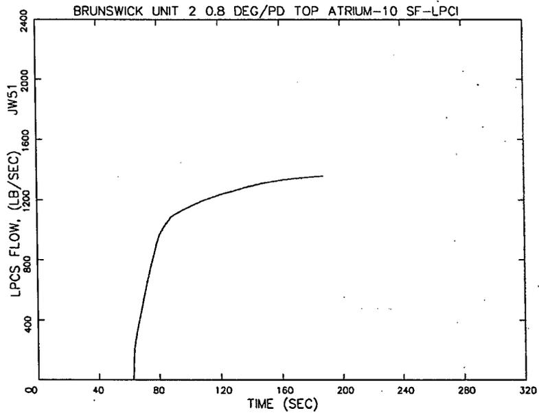
**Figure 6.12 Limiting TLO Recirculation Line Break
