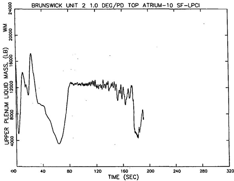
**Figure 7.18 Limiting SLO Recirculation Line Break
