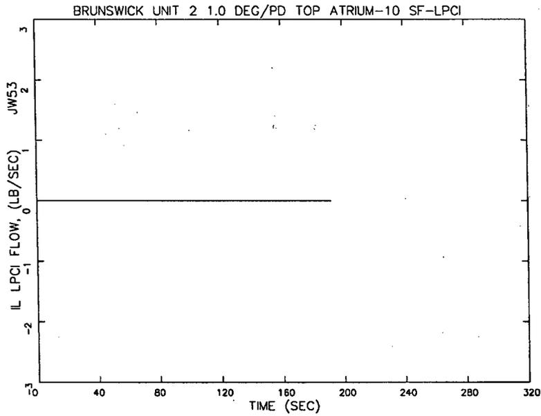
**Figure 7.13 Limiting SLO Recirculation Line Break
