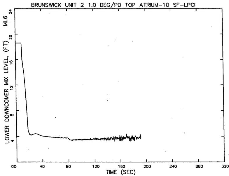
**Figure 7.16 Limiting SLO Recirculation Line Break
