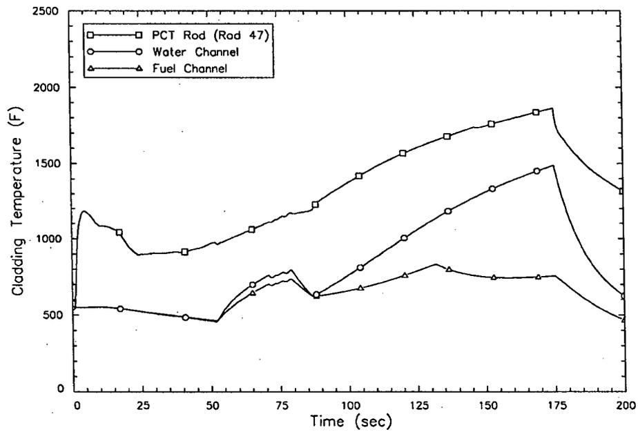
**Figure 7.26 Limiting SLO Recirculation Line Break
