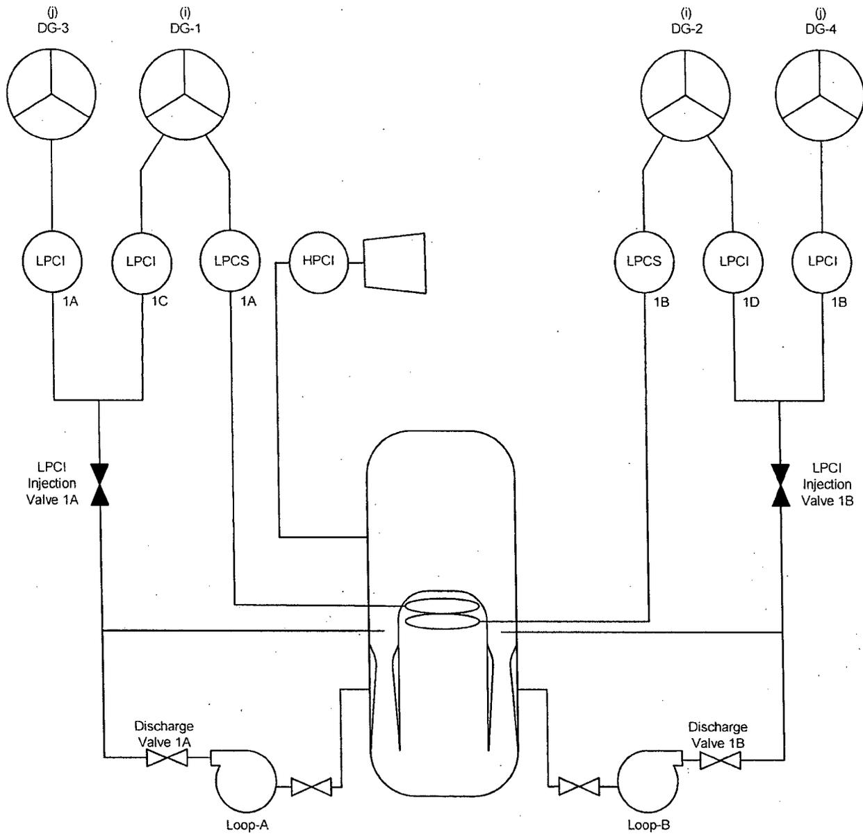
Figure 4.5 ECCS Schematic
