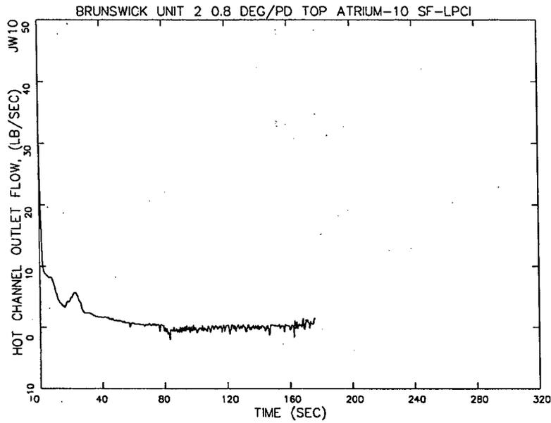
**Figure 6.21 Limiting TLO Recirculation Line Break
