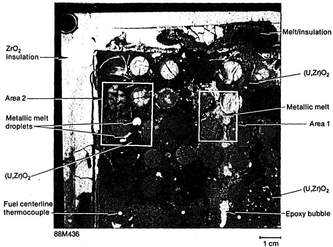
Figure 94. Metallographic cross section K1 at 0.83 m above the bottom of the instrumented fuel rods.
