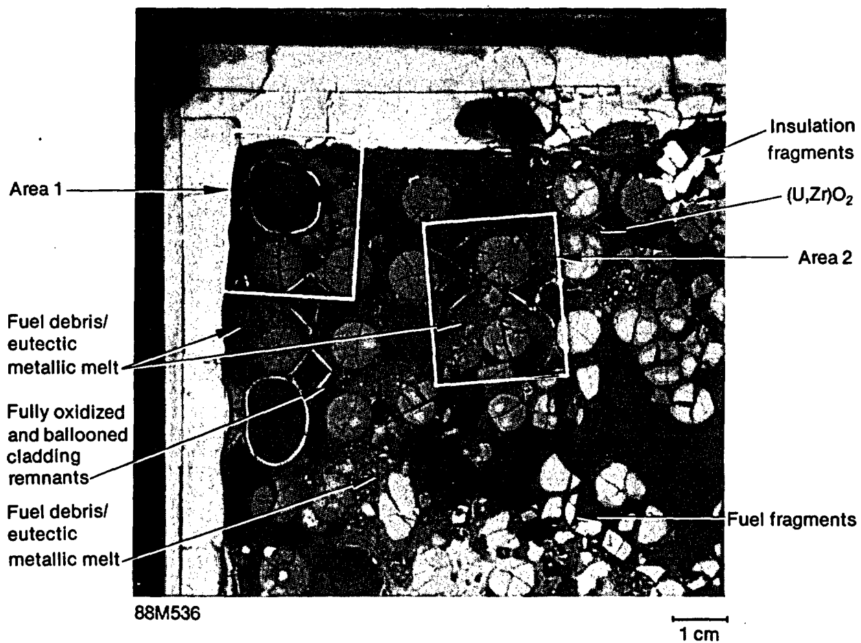
Figure 120. Metallographic cross section N1 at 1.14 m above the bottom of the instrumented fuel rods.
