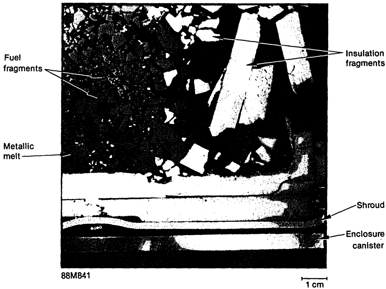
Figure 141. Metallographic cross section Q4 at 1.45 m above the bottom of the instrumented fuel rods.
