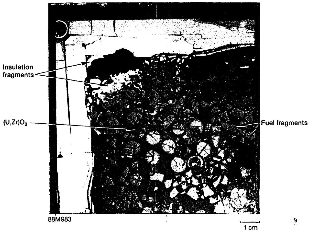
Figure 134. Metallographic cross section P1 at 1.30 m above the bottom of the instrumented fuel rods.
