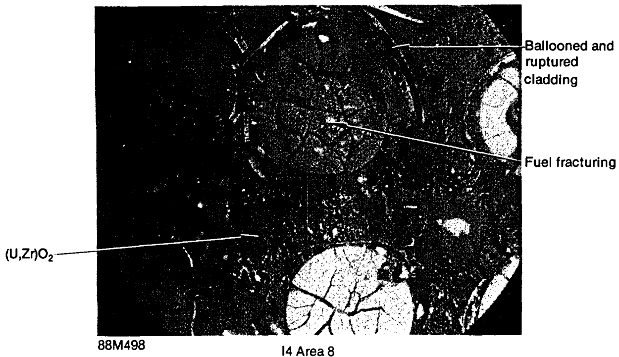
Figure 85. Details of metallographic cross section I4 at 0.66 m.
