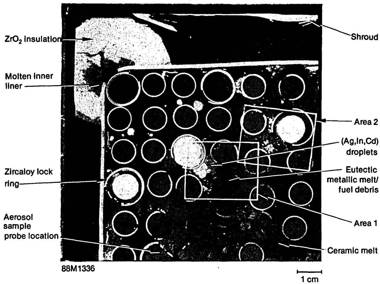
Figure 43. Metallographic cross section G2 (bottom) at 0.43 m above the bottom of the instrumented fuel rods.
