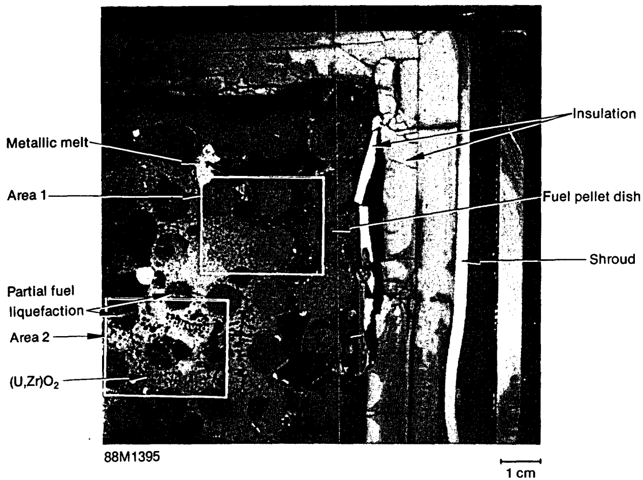
Figure 95. Metallographic cross section K2 at 0.88 m above the bottom of the instrumented fuel rods.
