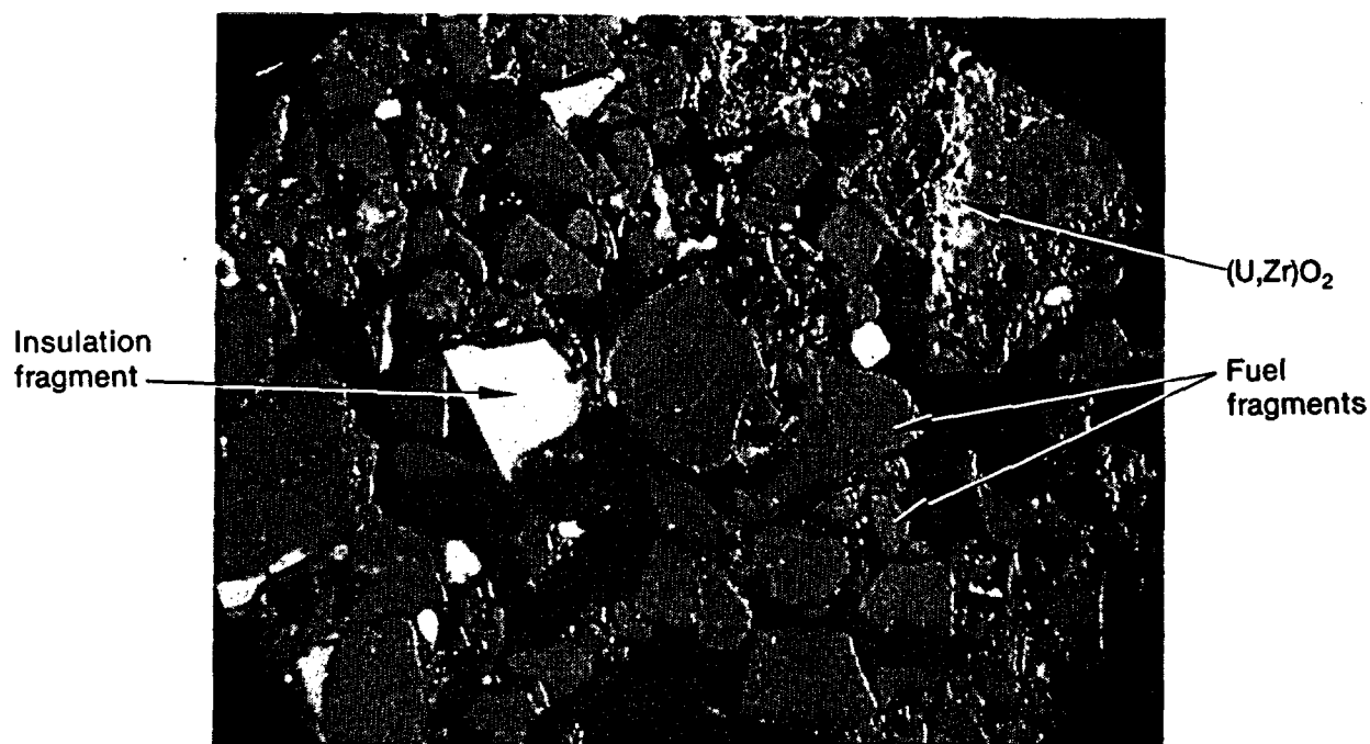
Figure 143. Details of metallographic cross section Q3 at 1.45 m.
