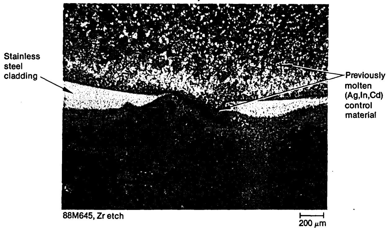
Figure 170. Molten droplet of (Ag,In,Cd) escaping through failed stainless steel cladding at 0.46 m.
