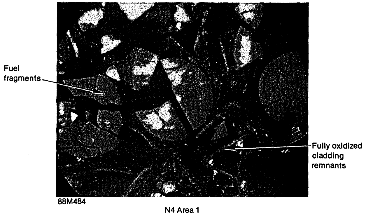
Figure 126. Details of metallographic cross section N4 at 1.14 m.
