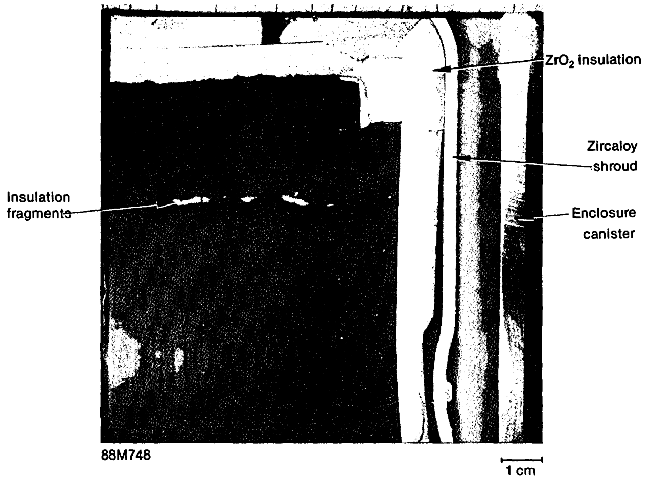
Figure 145. Metallographic cross section R2 at 1.68 m above the bottom of the instrumented fuel rods.
