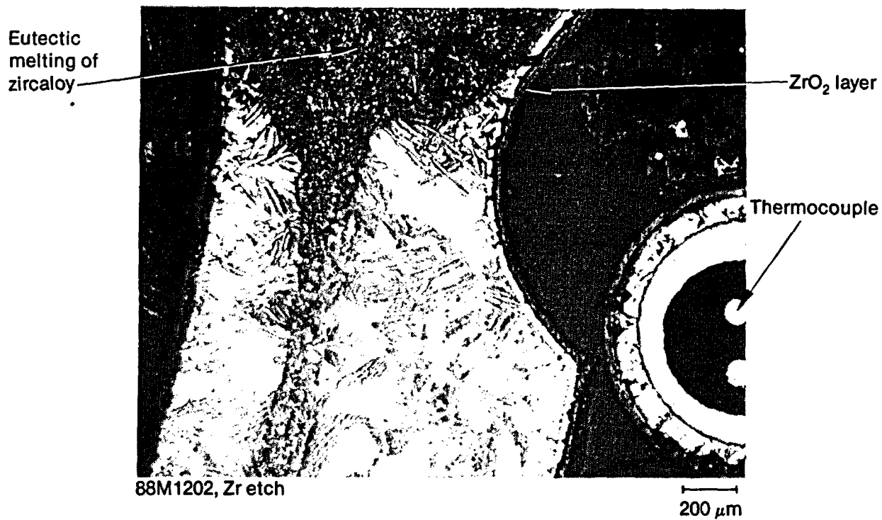
Figure 243. Liquefaction of upper portion of zircaloy guide tubes at 1.80 m.
