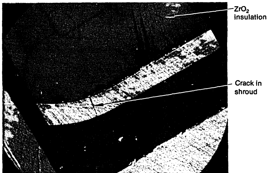
Figure 117. Details of metallographic cross section M1 and M2 at 1.04 m.
