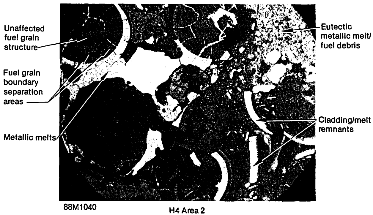
Figure 66. Details of metallographic cross section H4 at 0.58 m.
