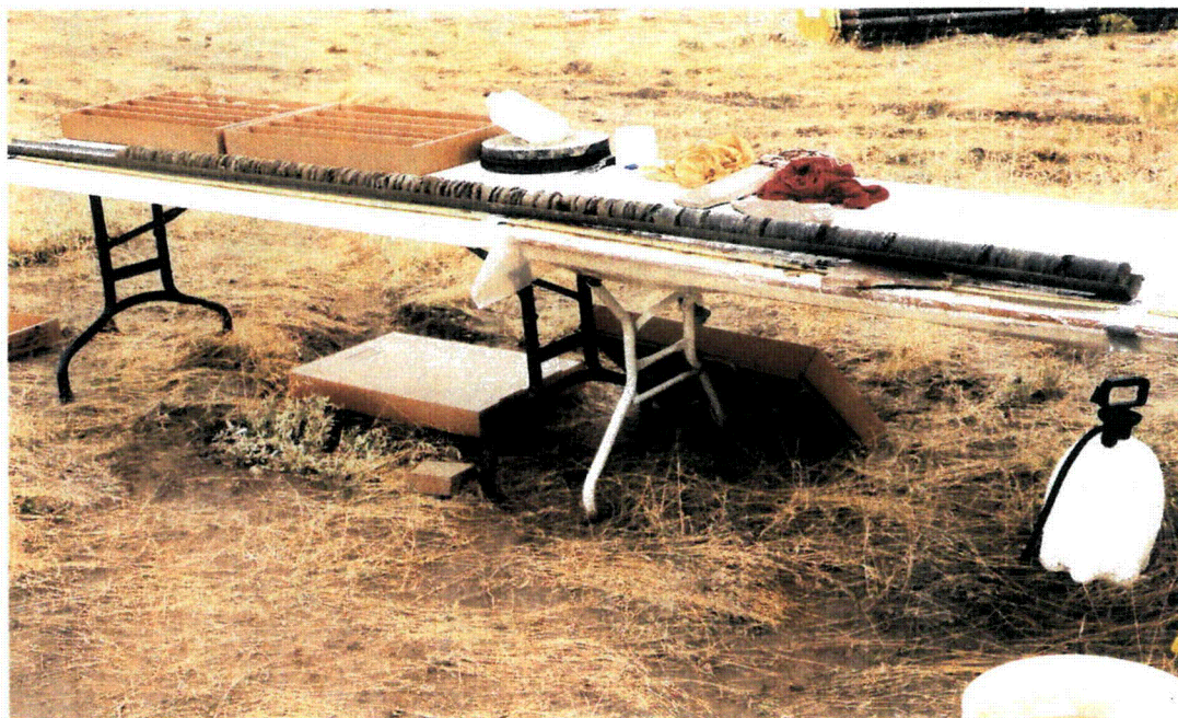
Figure 7. Core from hole 0210, from 26 (left) to 36 ft (right), showing progression in depth from highly weathered to slightly weathered bedrock in the Prairie Canyon Member.
