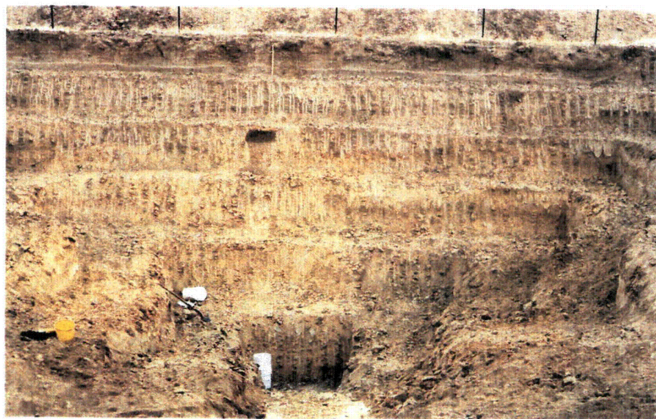
Figure 2. Test pit 0156. Alluvial-mud deposits are approximately 20 ft thick, and Mancos Shale is at bottom of pit. White 5-gallon buckets and shovel provide scale.
