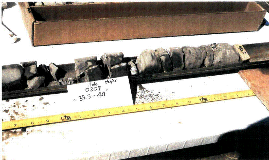
Figure 9. Gypsum (white) filling a vertical fracture at 39.5- to 40-ft depth in moderately weathered lower Blue Gate Member bedrock at corehole 0209.
