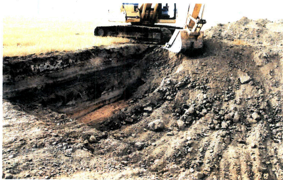
Figure 1. View of brown eolian material exposed at a depth of 7 ft in test pit 0151.
