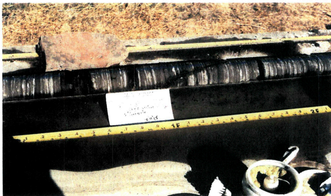
Figure 10. Limonite (orange) coating high-angle fracture at about a 62-ft depth in slightly weathered lower Blue Gate Member bedrock at corehole 0207.
