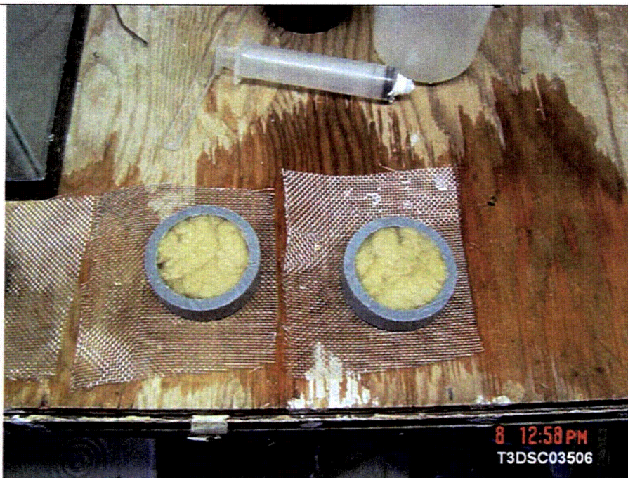
Figure 1. Example fiber pucks prepared for immersion in ICET test solution.
