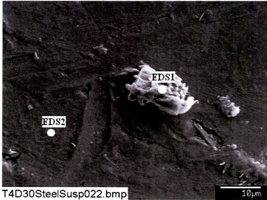
Figure F4-3. Annotated SEM image magnified 1800 times for a Test #4, Day-30 unsubmerged uncoated steel coupon sample. (T4D30SteelSusp022.bmp)
