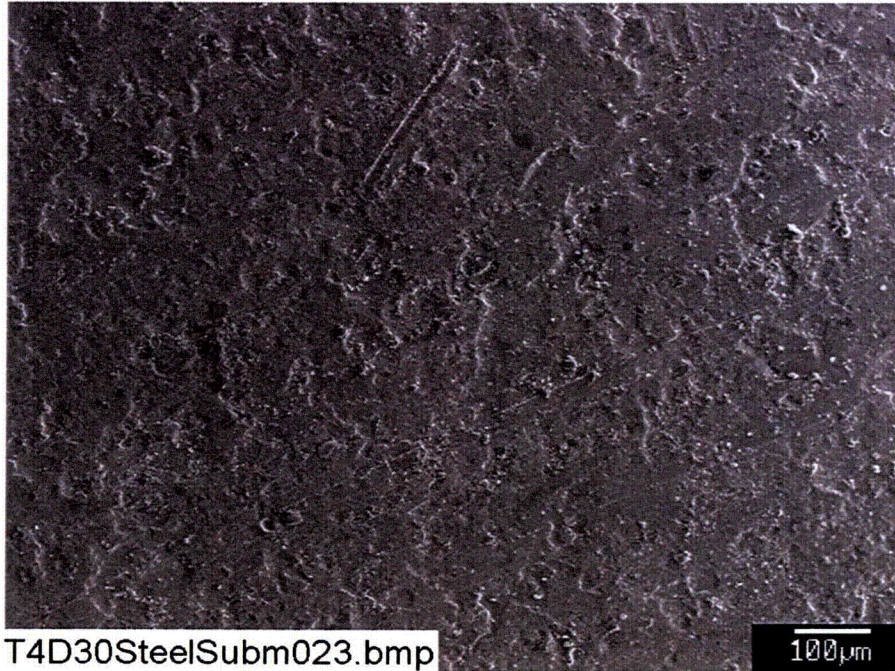
Figure F4-6. SEM image magnified 100 times for a Test #4, Day-30 submerged uncoated steel coupon sample. (T4D30SteelSubm023.bmp)
