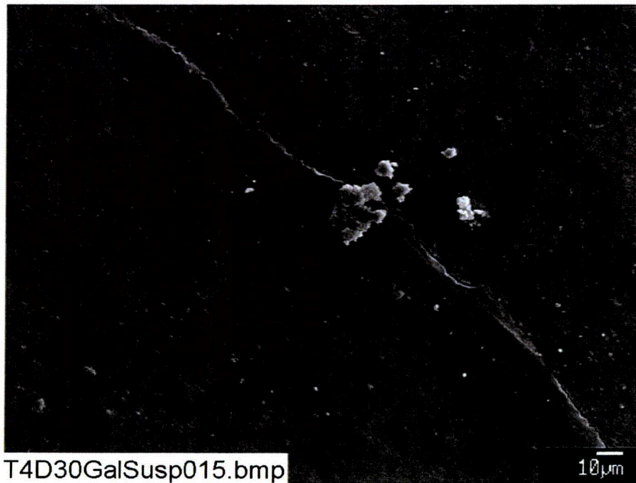
Figure F3-2. SEM image magnified 500 times for a Test #4, Day-30 unsubmerged galvanized steel coupon sample. (T4D30GalSusp015.bmp)
