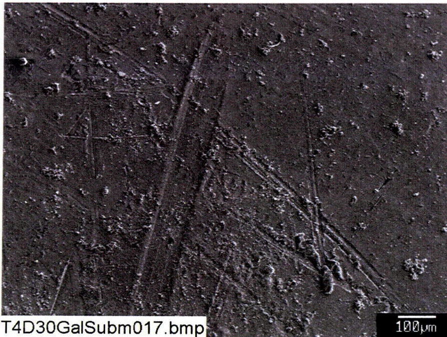
Figure F3-6. SEM image magnified 100 times for a Test #4, Day-30 submerged galvanized steel coupon sample. (T4D30GalSubm017.bmp)
