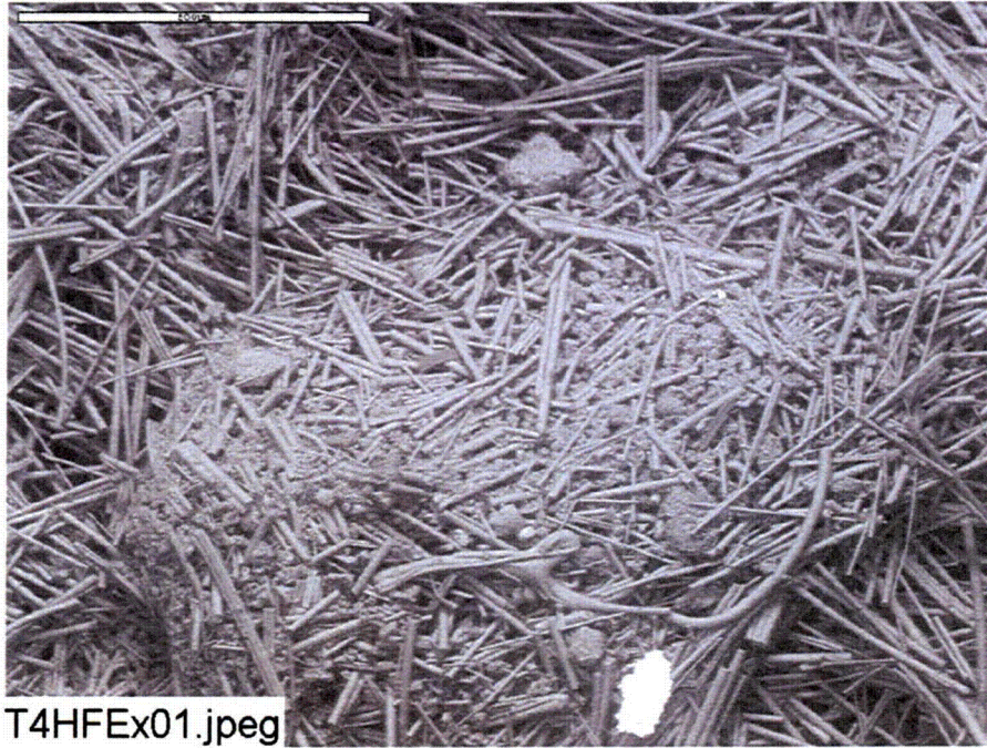
Figure C4-1. Environmental SEM image magnified 100 times for a Test #4, Day-30 exterior high-flow fiberglass sample. (T4HFEx01.jpeg)
