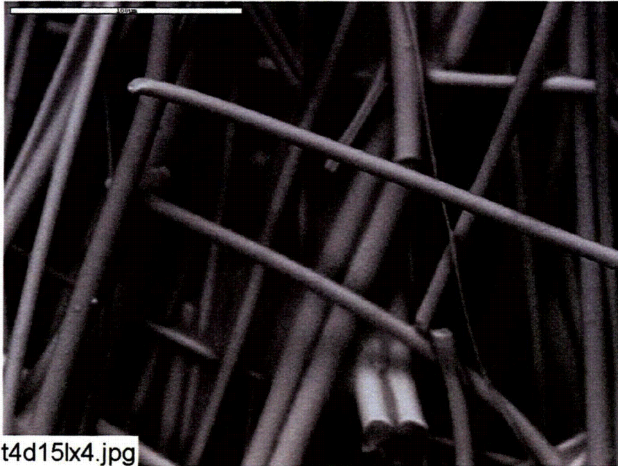
Figure B1-3. Environmental SEM image magnified 500 times for a Test #4, Day-15 exterior low-flow fiberglass sample. (t4d15lx4.jpg)
