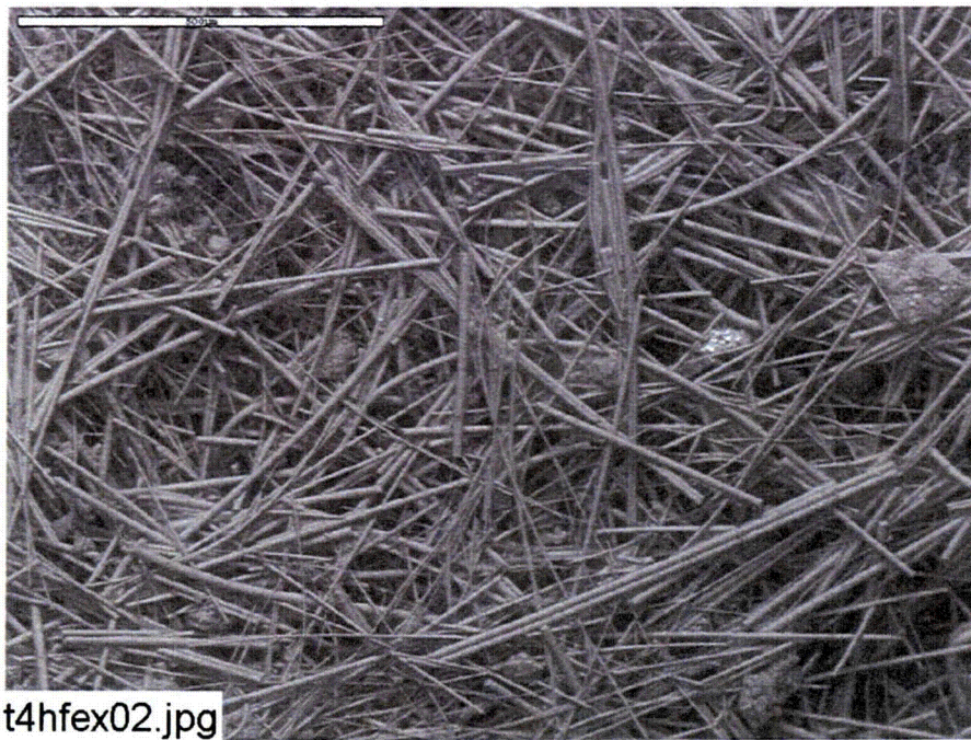
Figure C4-2. Environmental SEM image magnified 100 times for a Test #4, Day-30 exterior high-flow fiberglass sample. (t4hfex02.jpg)
