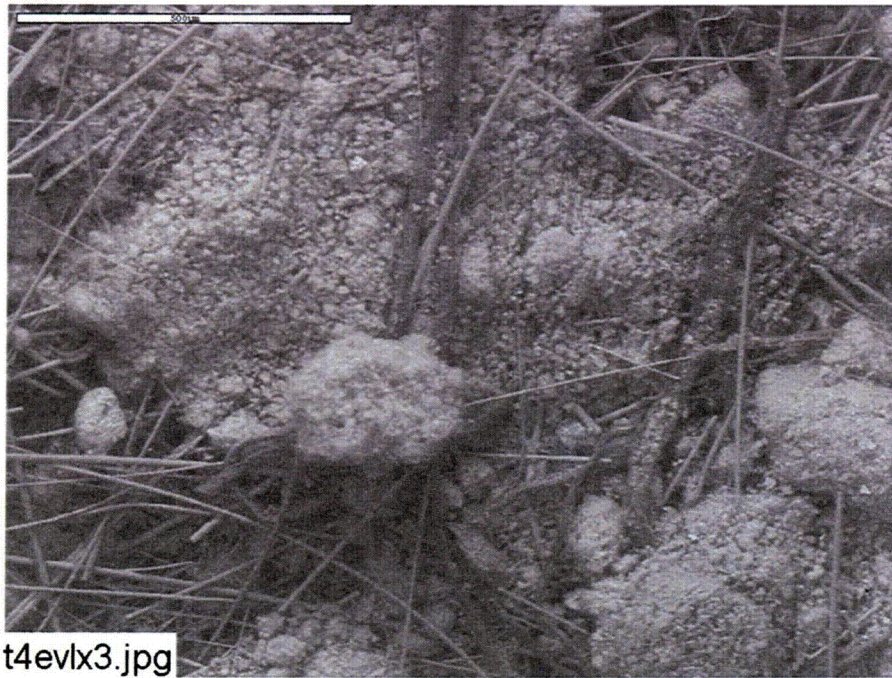
Figure C3-2. Environmental SEM image magnified 100 times for a Test #4, Day-30 exterior low-flow fiberglass sample in a big envelope. (t4evlx3.jpg)
