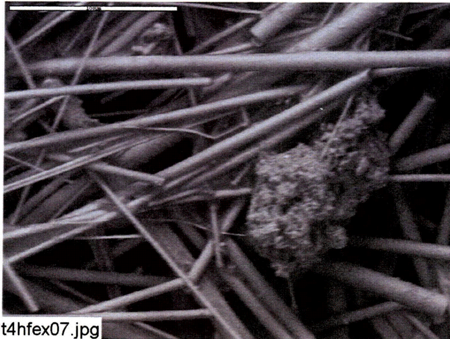
Figure C4-3. Environmental SEM image magnified 500 times for a Test #4, Day-30 exterior high-flow fiberglass sample. (t4hfex07.jpg)
