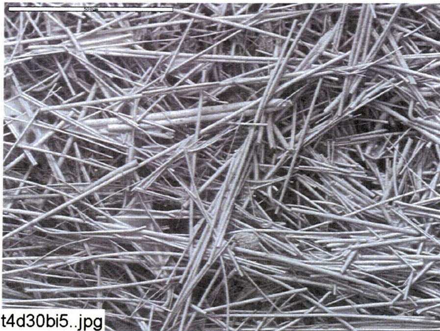
Figure C7-4. Environmental SEM image magnified 100 times for a Test #4, Day-30 interior fiberglass sample within the birdcage. (t4d30bi5.jpg)
