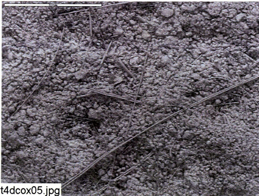
Figure C6-2. Environmental SEM image magnified 100 times for a Test #4, Day-30 exterior fiberglass sample on the drain collar (away from the drain screen). (t4dcox05.jpg)
