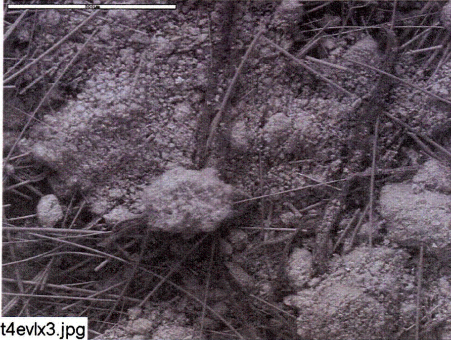
Figure 3-50. ESEM image magnified 100 times for a Test #4, Day-30 exterior low-flow fiberglass sample in a big envelope. (t4evlx3.jpg)
