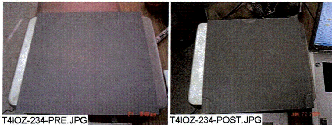
Figure 3-105. IOZ-234 submerged, pre-test (left) and post-test (right).
