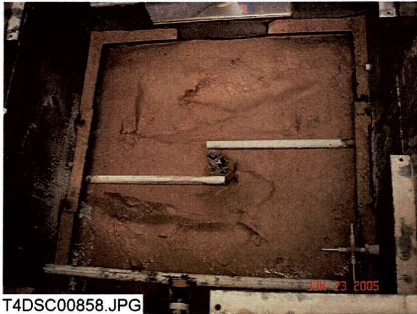
Figure 3-120. Sediment on the tank bottom.
