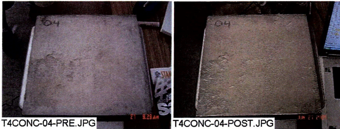
Figure 3-109. Conc-004 submerged, pre-test (left) and post-test (right).
