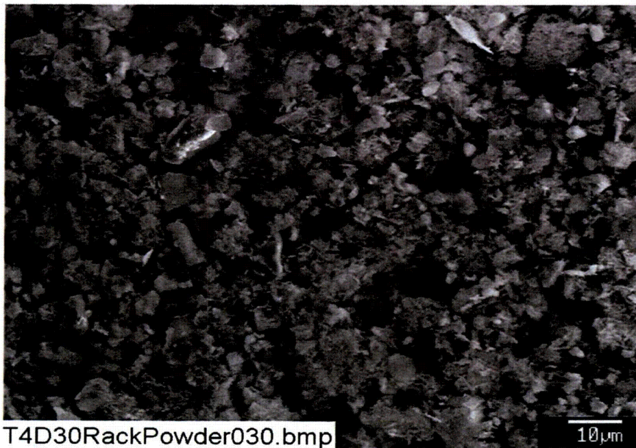
Figure 3-130. SEM image magnified 1000 times for a Test #4, Day-30 fine powder on the submerged rack. (T4D30RackPowder030.bmp)
