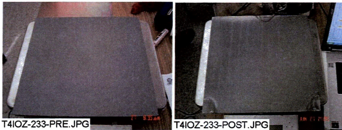
Figure 3-104. IOZ-233 submerged, pre-test (left) and post-test (right).
