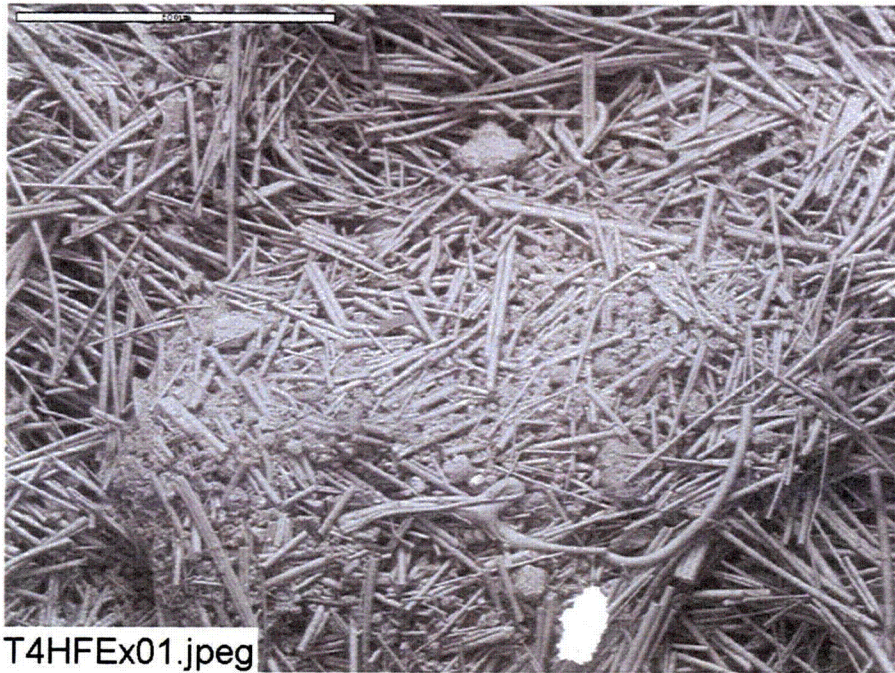
Figure 3-54. ESEM image magnified 100 times for a Test #4, Day-30 exterior high-flow fiberglass sample. (T4HFEx01.jpg)
