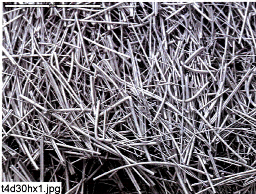
Figure 3-62. ESEM image magnified 100 times for a Test #4, Day-30 exterior high-flow fiberglass sample in front of a header (inserted on Day 4). (t4d30hx1.jpg)
