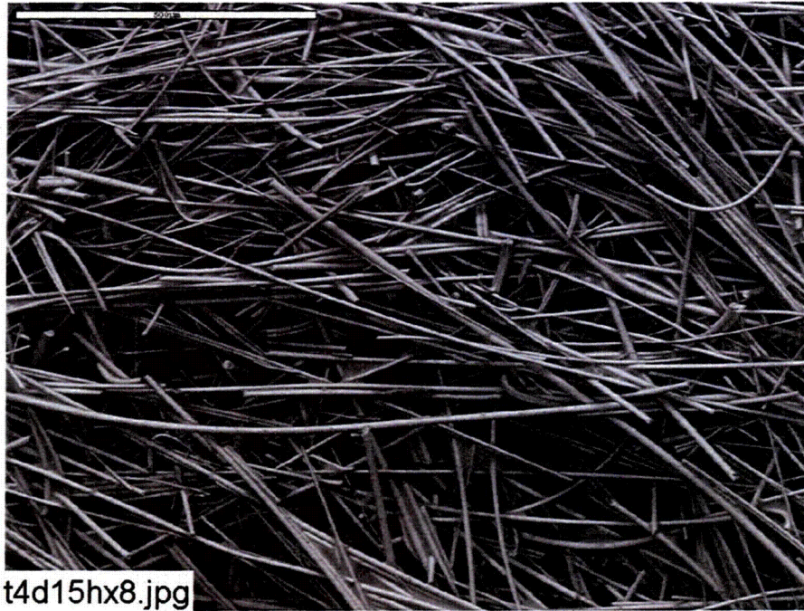
Figure 3-31. ESEM image magnified 100 times for a Test #4, Day-15 exterior high-flow fiberglass sample. (t4d15hx8.jpg)
