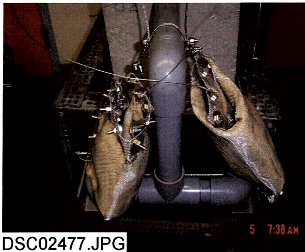
Figure 2-4. Fiberglass samples attached to a submerged coupon rack.
