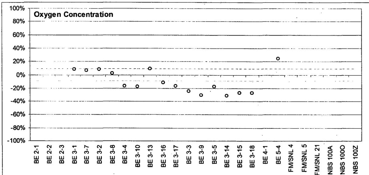
Figure 6-4: Scatter Plot of Relative Differences for Oxygen Concentration in ICFMP BE #3 and #5 (Experimental uncertainty is 9%.)
