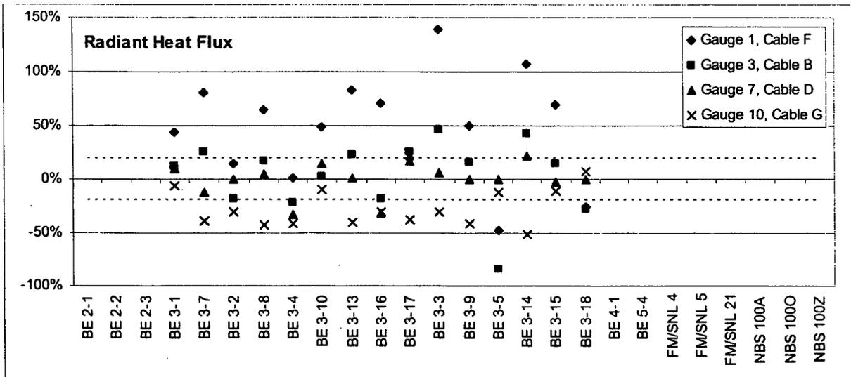
Figure 6-9: Scatter Plot of Relative Differences for Radiant Heat Flux in ICMP BE #3 (Experimental uncertainty is 20%.)
