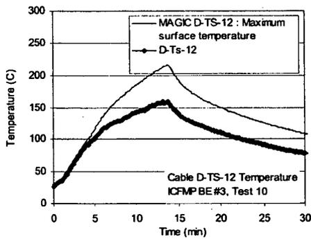
Figure A-46: Thermal Environment near Cable D, ICFMP BE #3, Tests 4 and 10
