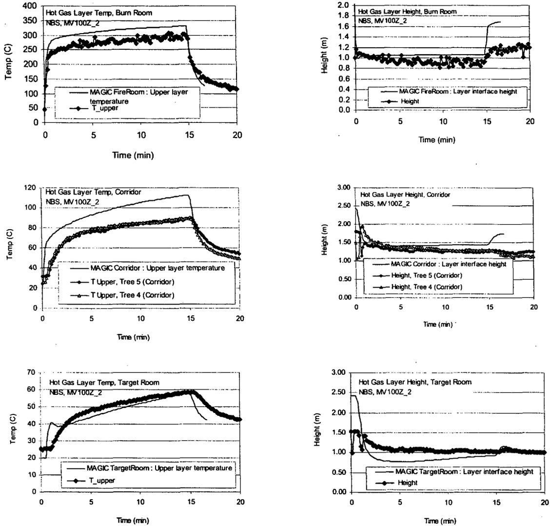
Figure A-17: Hot Gas Layer (HGL) Temperature and Height, NBS Multiroom Test 100Z
