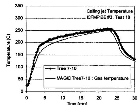
Figure A-19: Near-Ceiling Gas (Ceiling Jet) Temperatures, ICFMP BE #3, Open-Door Tests
