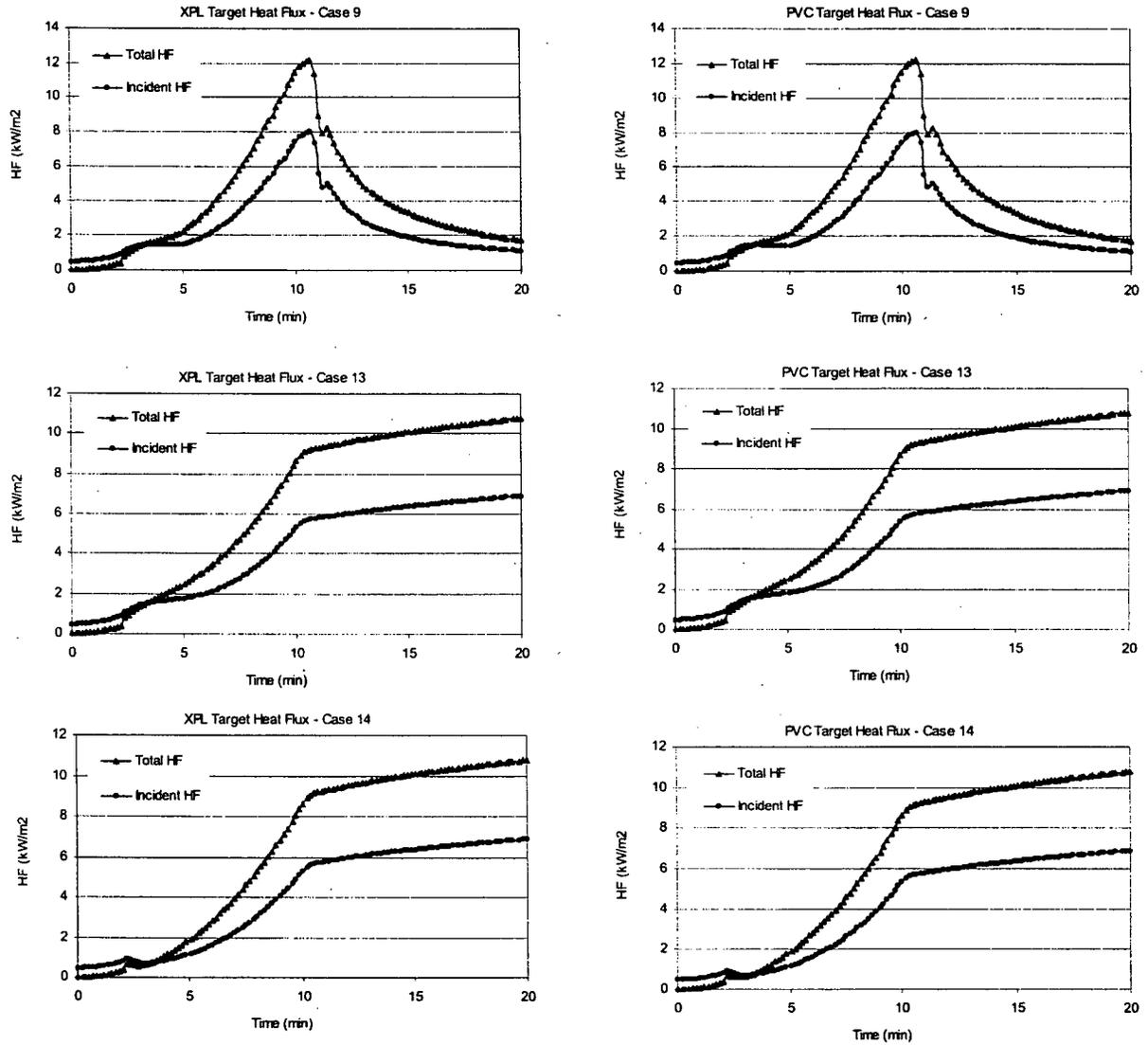
Figure 5-13: Target Heat Flux Profiles, 5-MW Fire
