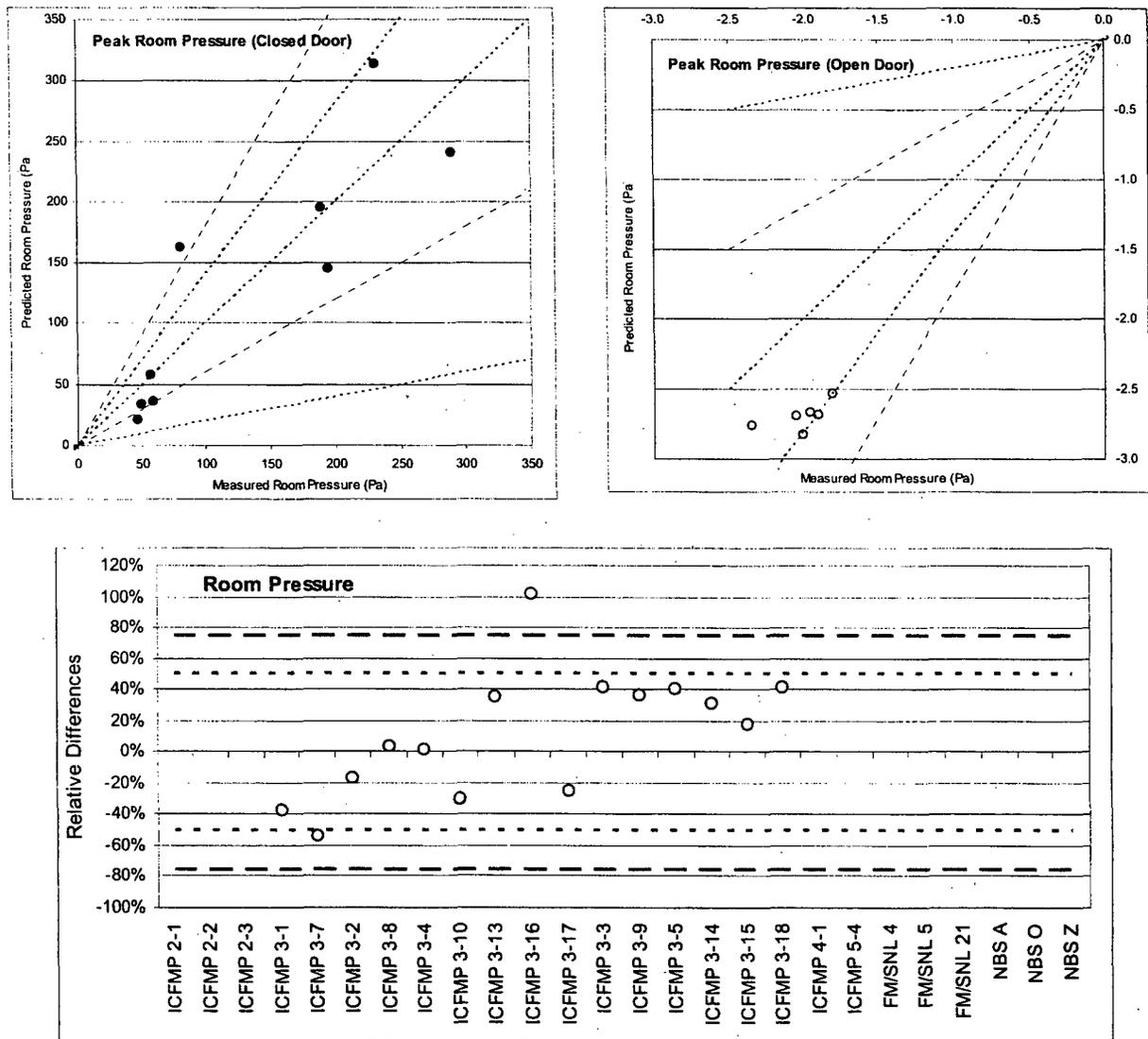
Figure 6-6: Scatter Plot of Relative Differences for Room Pressure in ICFMP BE #3 [Experimental uncertainties are 40% (no forced vent) and 80% (forced vent).]
