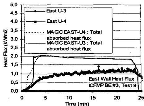
Figure A-76: Short-Wall Heat Flux and Surface Temperature, ICFMP BE #3, Closed- and Open-Door Tests
