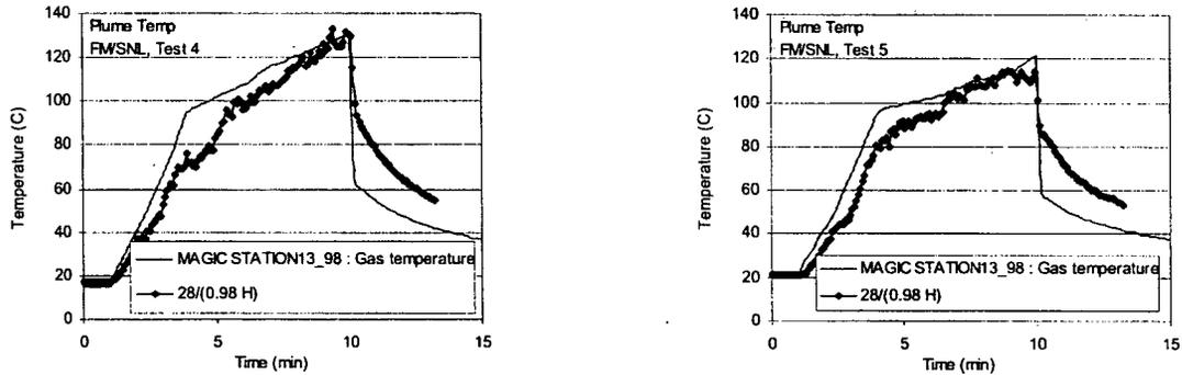
Figure A-23: Near-Plume Temperatures, FM/SNL Series, Sector 13
