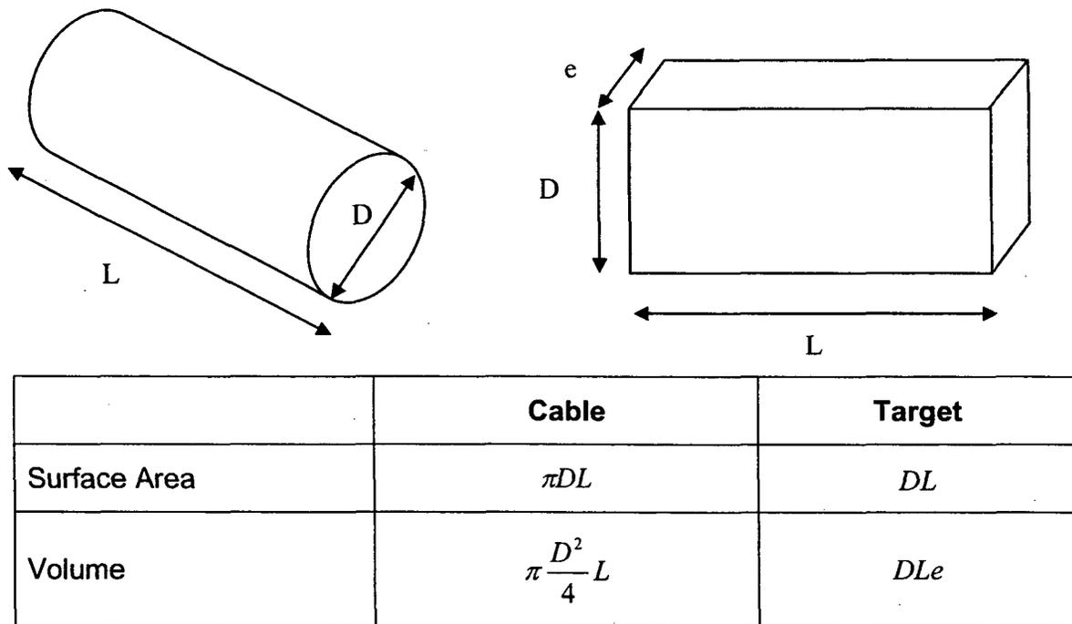
Figure 5-10: Equivalence between Cable and Targets
