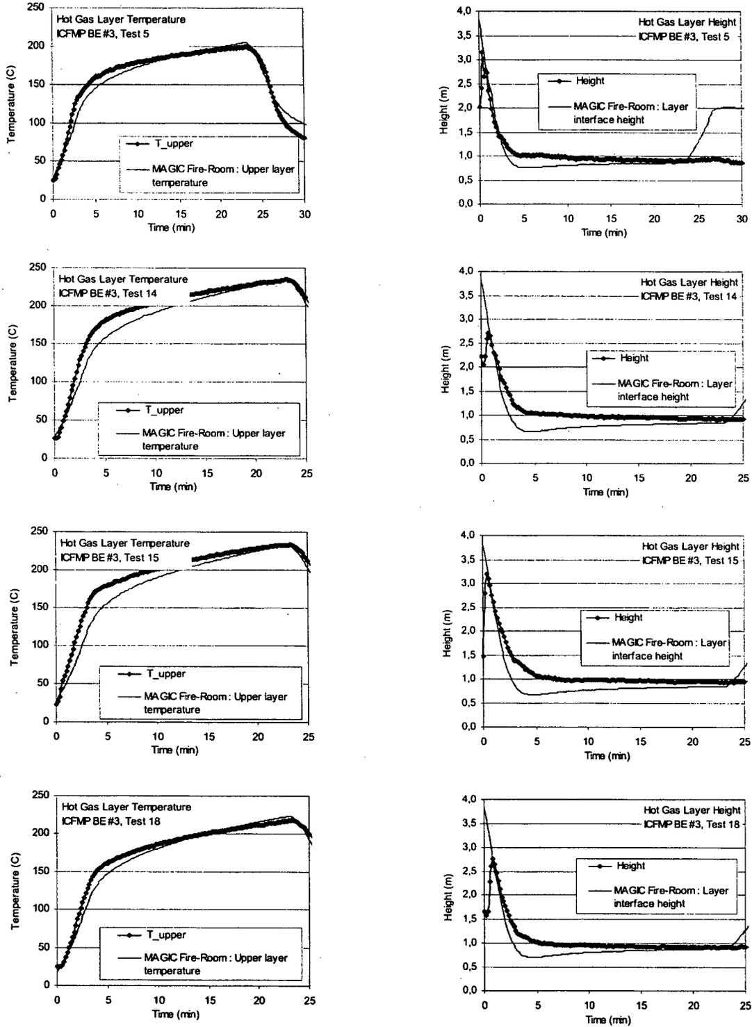
Figure A-7: Hot Gas Layer (HGL) Temperature and Height, ICMP BE #3, Open-Door Tests
