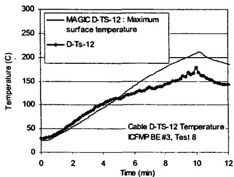
Figure A-45: Thermal Environment near Cable D, ICFMP BE #3, Tests 2 and 8
