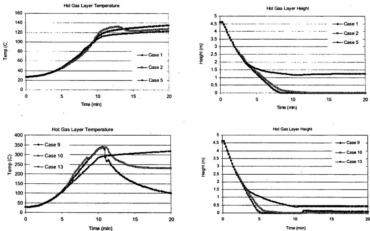
Figure 5-3: Hot Gas Layer Temperature Profiles
