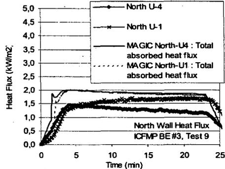
**Figure A-72: Long-Wall Heat Flux and Surface Temperature, ICFMP BE #3, Closed- and Open-Door Tests**
