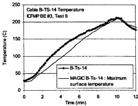
Figure A-37: Thermal Environment near Cable B, ICFMP BE #3, Tests 2 and 8
