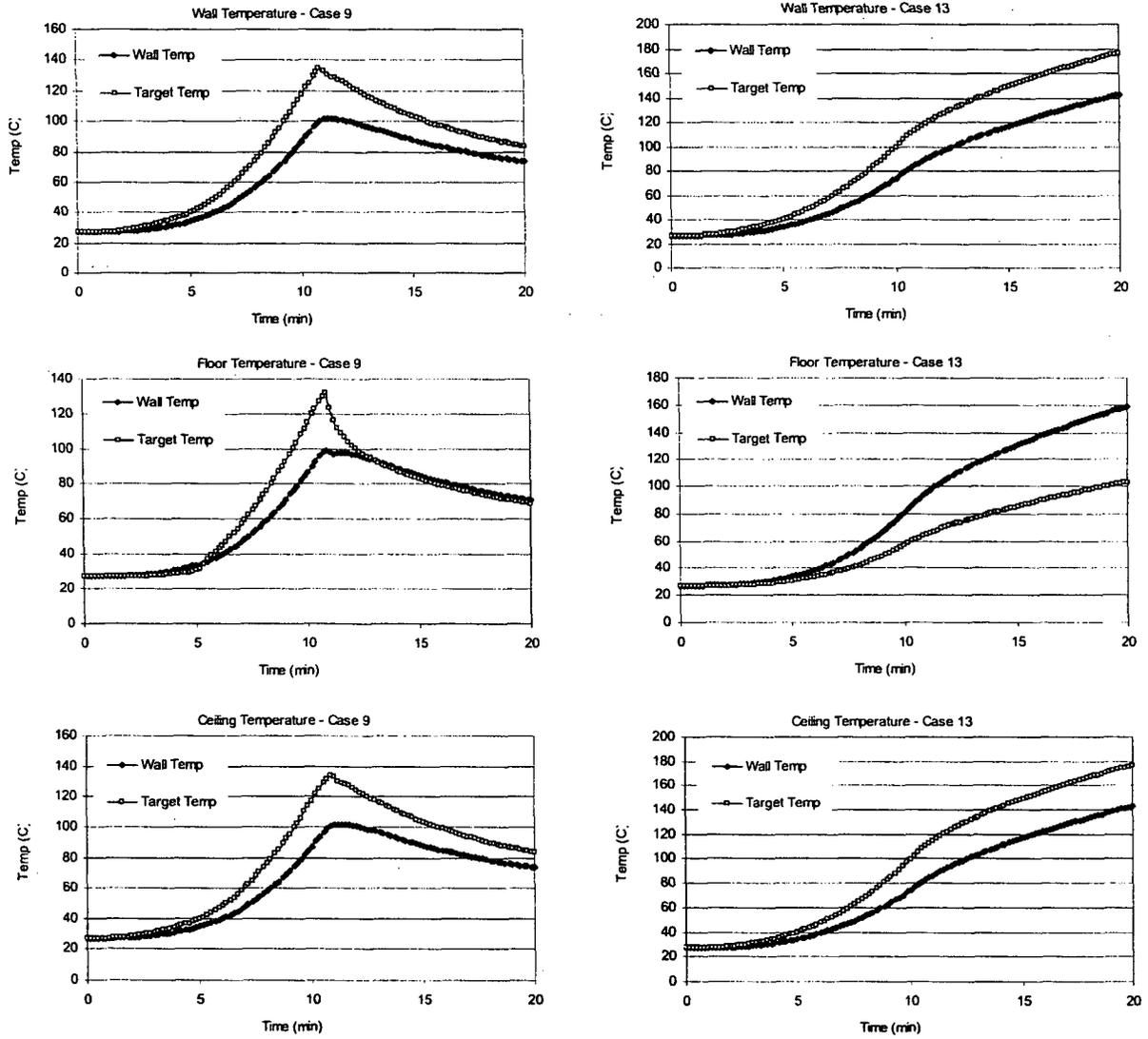
Figure 5-15: Target Temperature vs. Wall Temperature, 5-MW Fire
