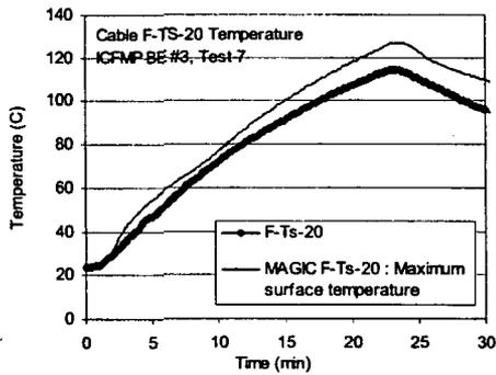
Figure A-52: Thermal Environment near Cable F, ICFMP BE #3, Tests 1 and 7
