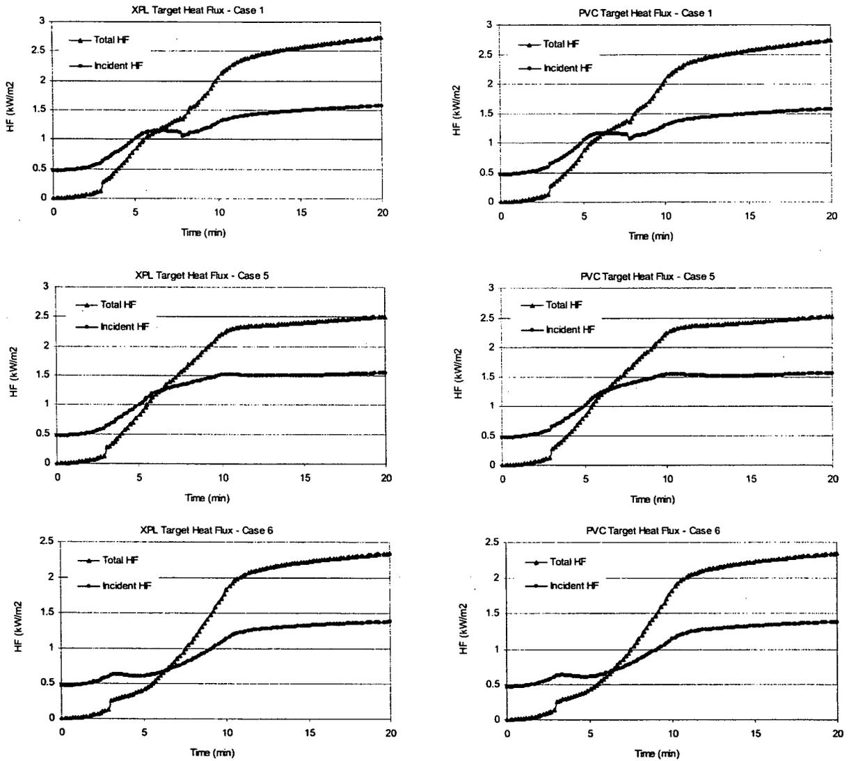
Figure 5-12: Target Heat Flux Profiles, 1-MW Fire
