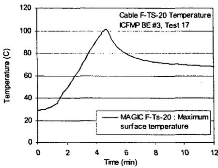
Figure A-56: Thermal Environment near Cable F, ICFMP BE #3, Test 17
