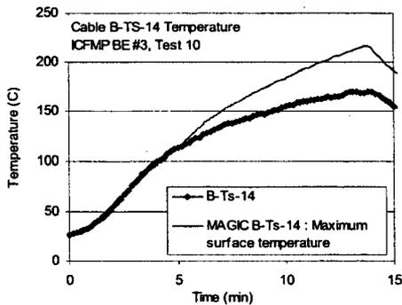
Figure A-38: Thermal Environment near Cable B, ICFMP BE #3, Tests 4 and 10
