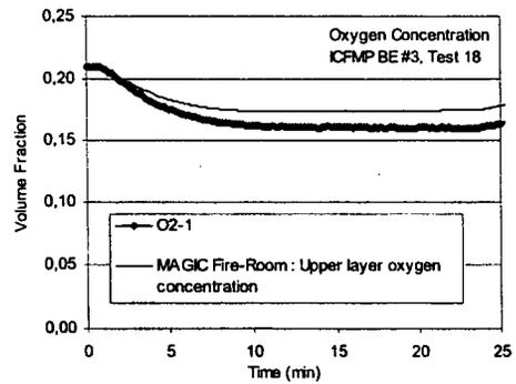
Figure A-30: Oxygen Concentration ICFMP BE #3, Open-Door Tests
