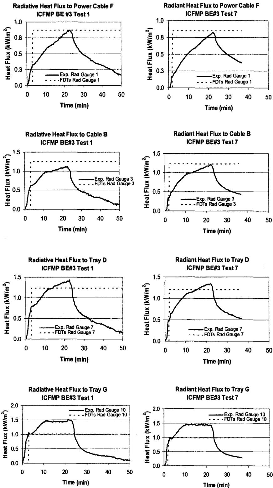
Figure A-22: Radiant Heat Flux, ICFMP BE #3, Tests 1 and 7
