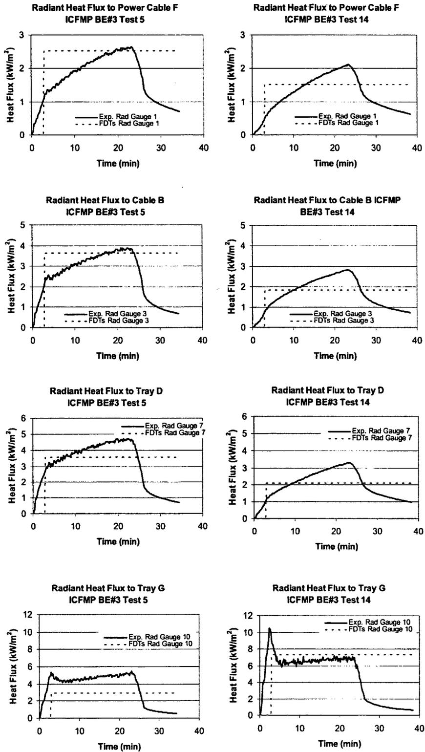
Figure A-26: Radiant Heat Flux, ICFMP BE #3, Tests 5 and 14
