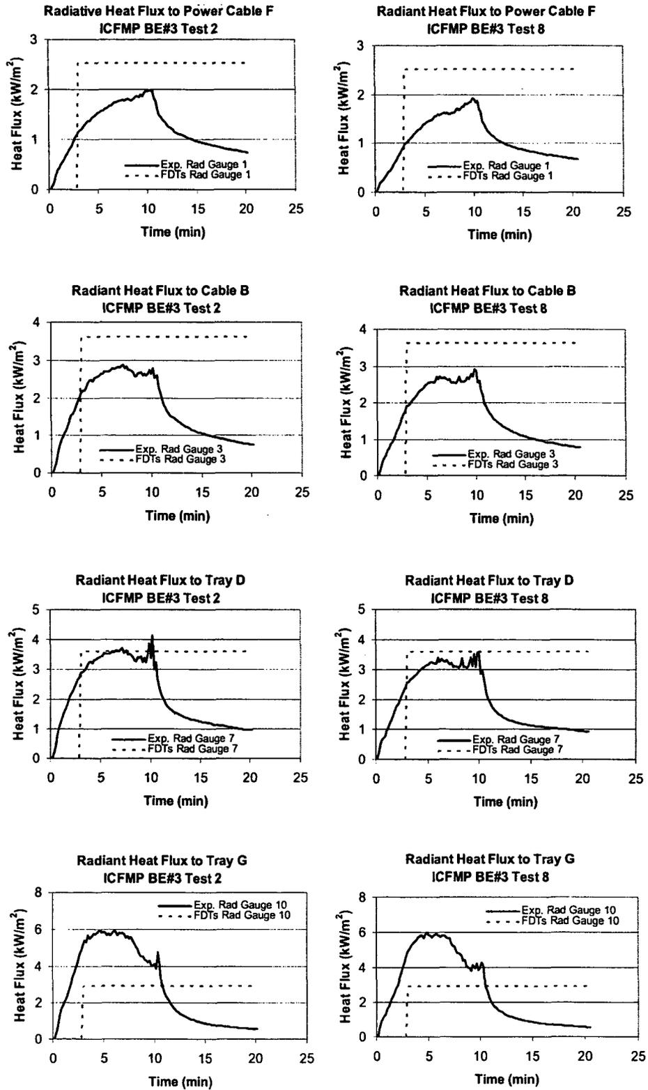
Figure A-23: Radiant Heat Flux, ICFMP BE #3, Tests 2 and 8
