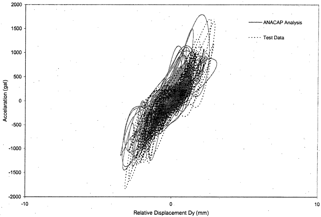
Figure 5-64 Comparison of Hysteresis Loops in Y-Direction for Run-5
