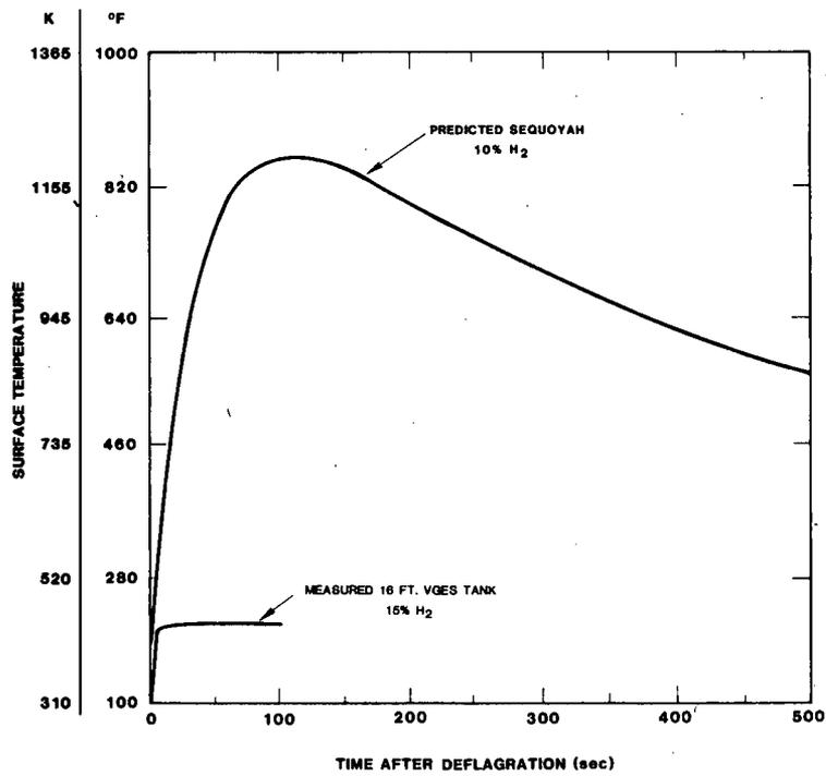
Figure 5-2. Comparison of Hollow Aluminum Cube Thermal Response Obtained From VGES Experiments and Sequoyah Upper Compartment Analysis
