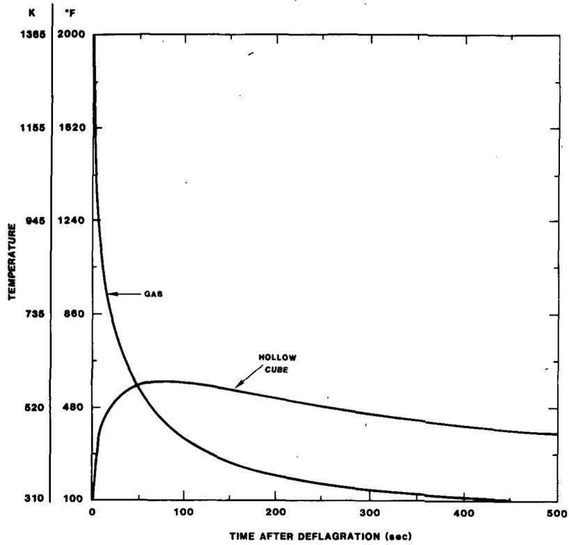
Figure 3-2. Temperature Profiles of Gas and Hollow Aluminum Cube Resulting From a 10% Hydrogen Burn in the Sequoyah Upper Compartment
