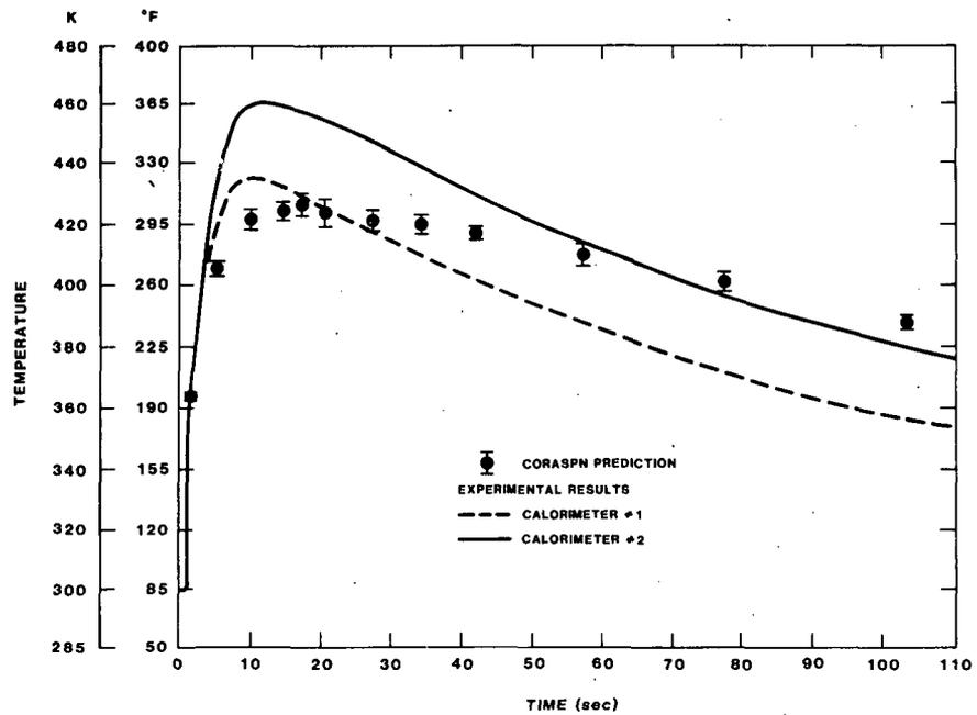
Figure 4-2. Gas Temperature Response Resulting from 15% Hydrogen Burn - Predicted vs. Flat-Plate Calorimeter Measurements.
