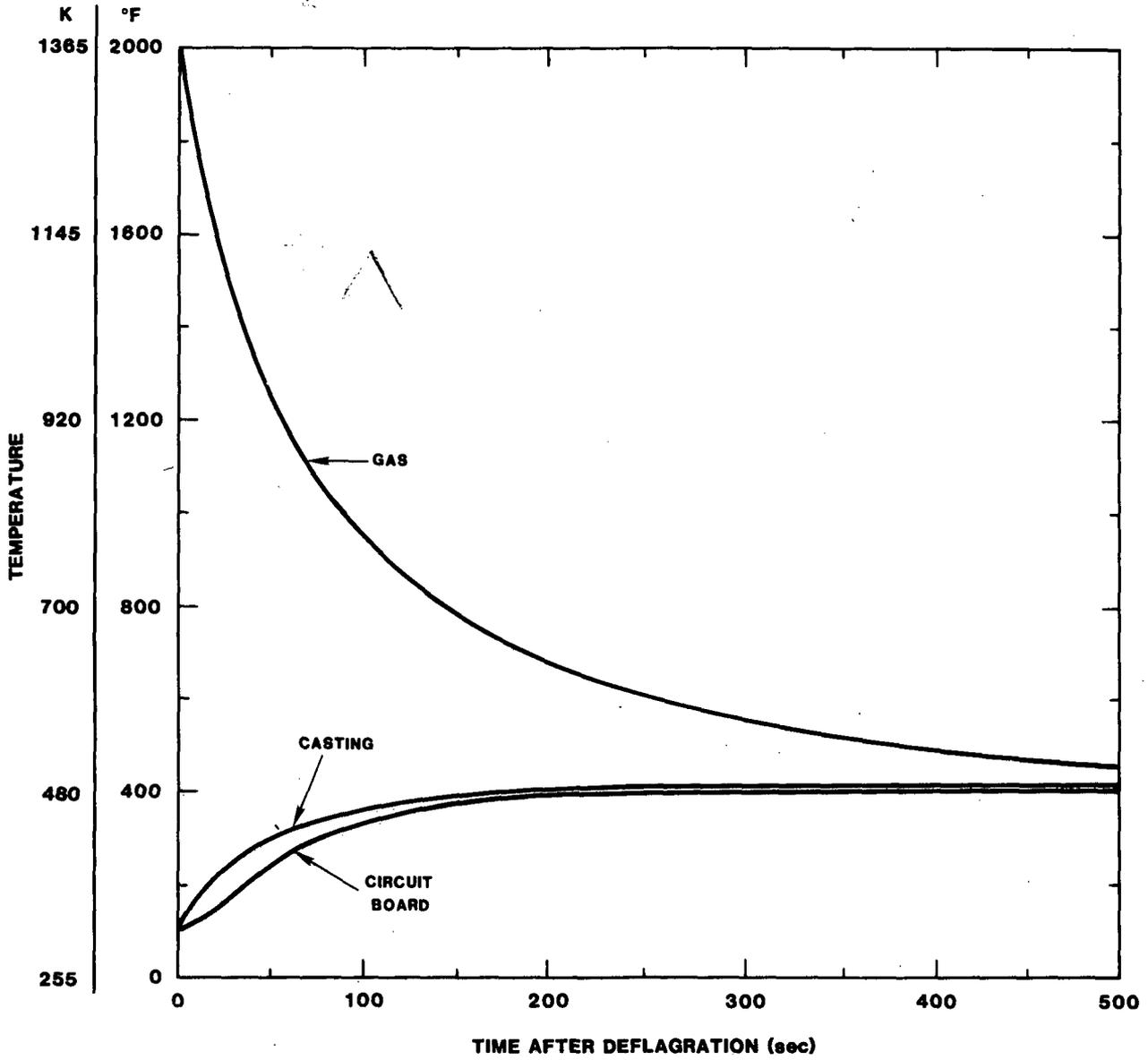
Figure 3-6. Temperature Profiles of Gas and Pressure Transducer Resulting From a 10% Hydrogen Burn in the Sequoyah Upper Compartment
