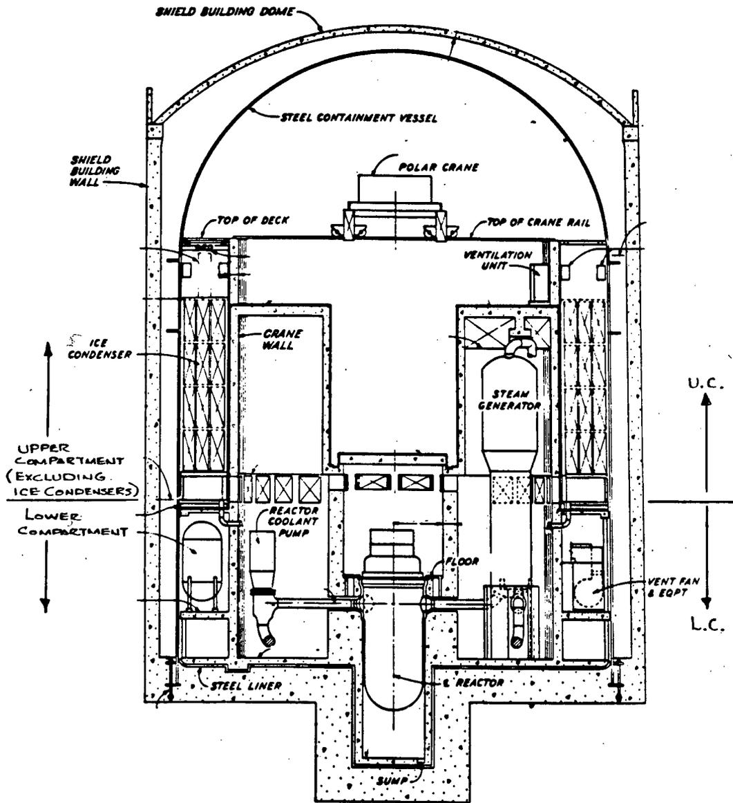
Figure 3-1. Sequoyah Ice Condenser Pressurized Water Reactor Containment Building
