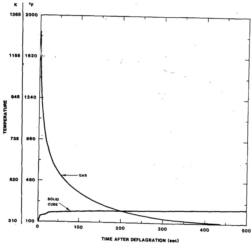
Figure 3-5. Temperature Profiles of Gas and Solid Aluminum Cube Resulting From a 10% Hydrogen Burn in the Sequoyah Lower Compartment
