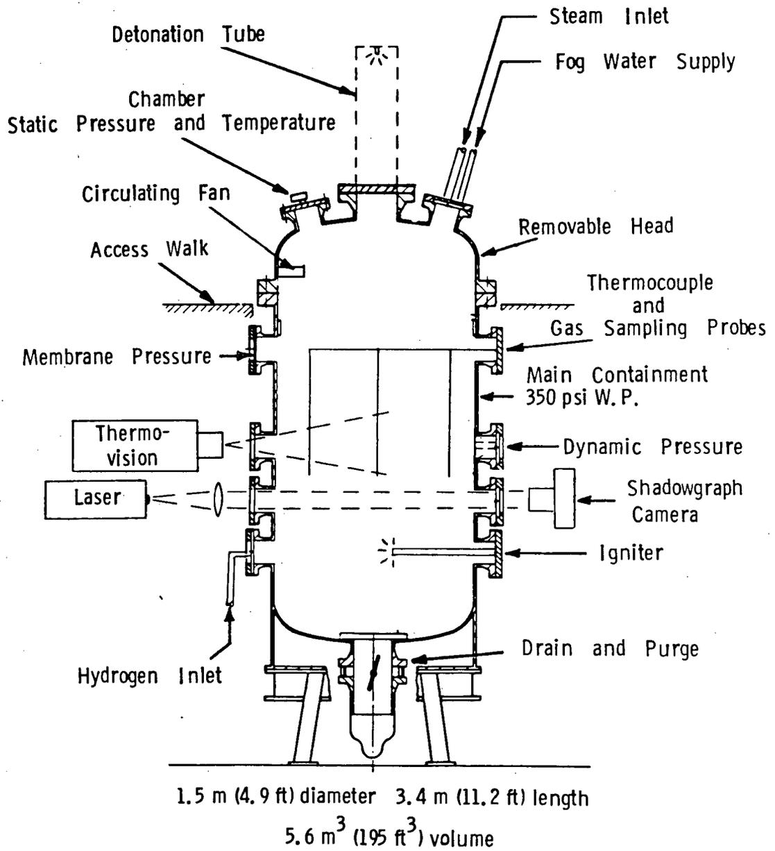
Figure 2-3. Fully Instrumented Test System (FITS)
