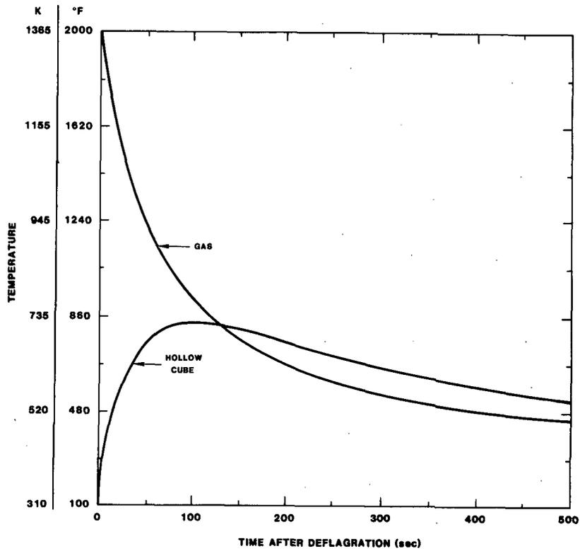
Figure 3-3. Temperature Profiles of Gas and Hollow Aluminum Cube Resulting From a 10% Hydrogen Burn in the Sequoyah Lower Compartment
