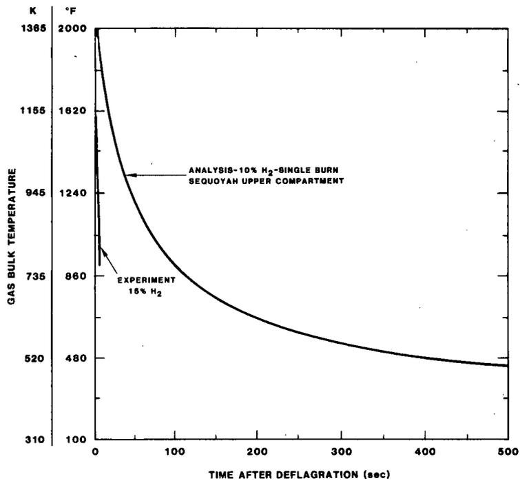
Figure 5-1. Comparison of Temperature Profiles Obtained From VGES Experiments and Sequoyah Upper Compartment Analysis
