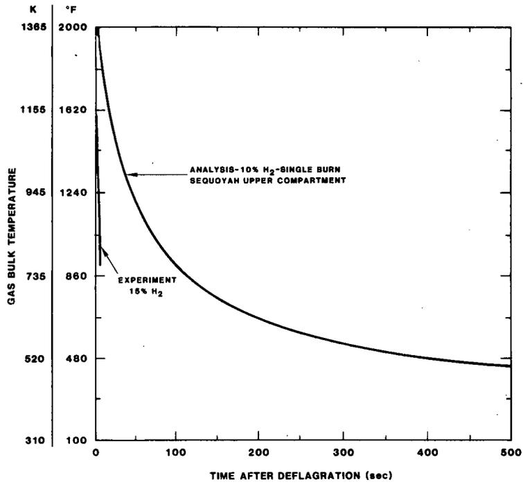
Figure 5-1. Comparison of Temperature Profiles Obtained From VGES Experiments and Sequoyah Upper Compartment Analysis
