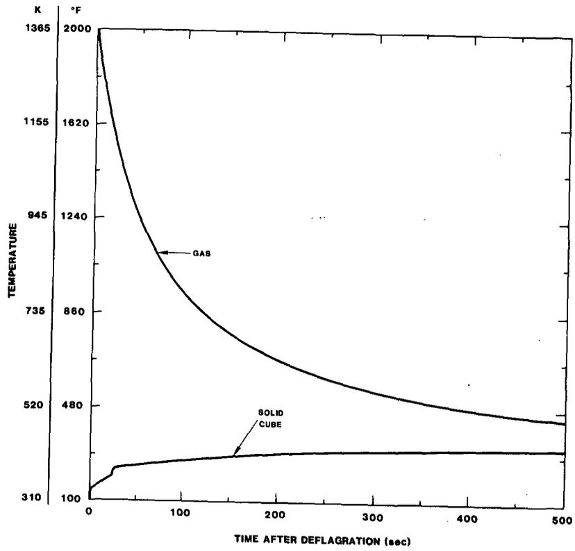
Figure 3-4. Temperature Profiles Gas and Solid Aluminum Cube Resulting From a 10% Hydrogen Burn in the Sequoyah Upper Compartment
